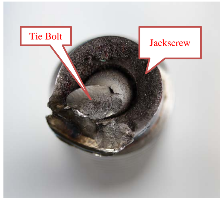
Figure 4 - Actuator Jackscrew Fracture Surface.
