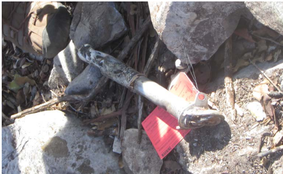
Figure 1 - The Horizontal Stabilizer Actuator, jackscrew segment, in its found location at accident site (Photograph courtesy of the DGAC).
