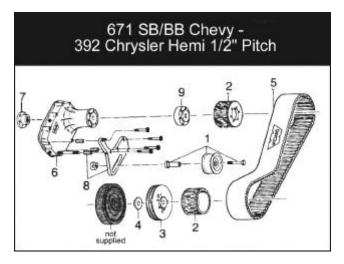
Components Parts List for 1/2" Pitch Street Drives (Listed parts are included in 671, 1/2" pitch kits).
