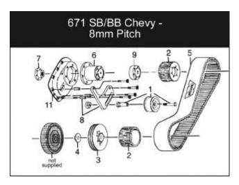
Components Parts List for 8mm Street/Comp Drives (Listed parts are included in 671, 8mm kits.)
