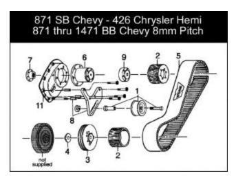
Individual Component Parts List for 8mm Street-Marine/Comp Drives (Listed parts are included in 871, 8mm kits).
