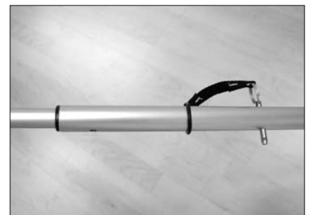
The drawbar is adjustable for three lengths. Pull out the inner tube and insert the securing pin when the holes of inner and outer tube are aligned with each other.
