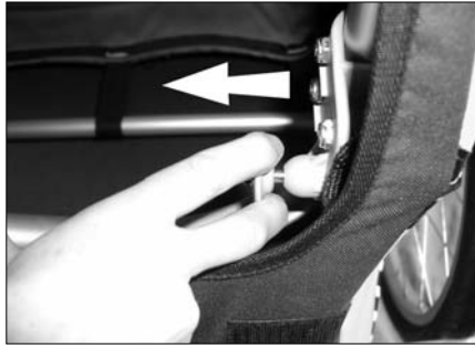
Releasing the disks of the auto-lock.
