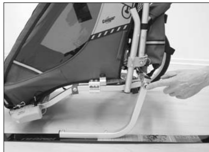
Insert the skier into the hollow axle while depressing the axle knob and ensure that the axle safely engages.
