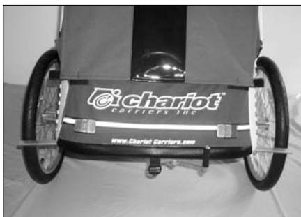
Plastic wheel on the Cabriolet, Comfort and Cheetah. Screw two reflectors onto each wheel at the corresponding brackets.
