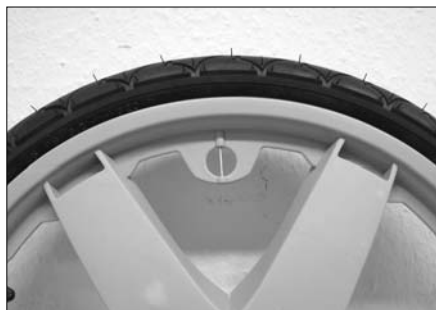
Plastic wheel on the Cabriolet, Comfort and Cheetah. Screw two reflectors onto each wheel at the corresponding brackets.
