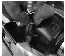
27 Once he has routed the clutch cable to the left hand lever, Dan reassembles the clutch lever setup using all stock parts. He then torques the bolts to 60–80 in–lbs.
