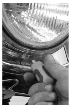
Conce the headlight trim is back in place, Dan reinstalls the single stock screw using a Phillips screwdriver. He then adjusts the clutch cable as per the H-D service manual procedure.
