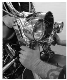
Dan positions the spotlight assembly onto its stock mounting points and reattaches the two switch harness connectors. He then checks that all switches and lights, except for the headlight, work.
