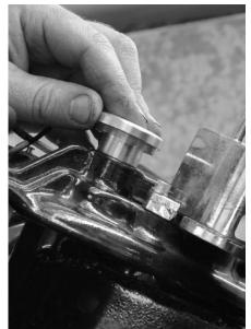
After putting a little WD-40 on them, the rest of the H-D riser bushing set (aluminum and neoprene) goes into the top of the top triple tree.
