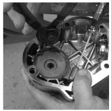
With the inner ramp positioned over the outer ramp so the balls are in their pockets, Dan secures the outer ramp to the end cover using the stock retaining ring and internal snap ring pliers.
