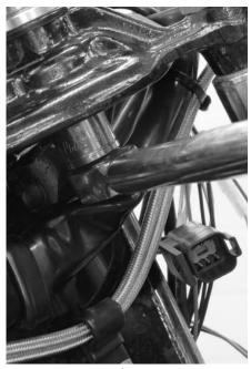
After slipping a 1/2" flat washer onto the other riser bolt and then installing it, Dan torques both bolts to 35 ft-lbs. using a 3/4" socket. And, yes, you'll have to turn the front end to get the riser bolts into the top tree.
