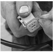
Once both harnesses are through the bars, Dan can reassemble the connectors by inserting the pins as per his diagram and popping in the end cap, followed by the rubber moisture barrier.
