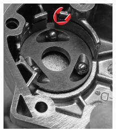
After aligning its tab with the slot in the cover (arrow), Dan drops in the outer clutch ramp, followed by the three stock balls.
