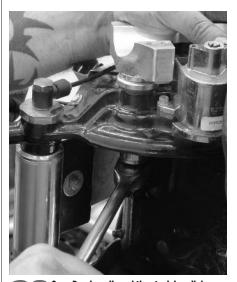
Once Dan has slipped the stock handlebar ground strap over a 1/2" x 2-1/4" coarsethreaded bolt, he threads the bolt into the Carlini riser using red Loctite and a 3/4" socket.
