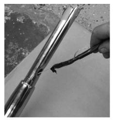
With a guide string taped to the end of the wiring harness, Dan coats the harness with a little WD-40 and feeds it into the switch hole while a buddy gently pulls on the guide string.
