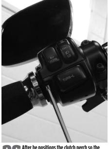
**26** After he positions the clutch perch so the lever is comfortable for Terry, Dan secures the switch housing to the handlebars using the two stock bolts and a T-25 Torx. He torgues the bolts to 25-35 in-lbs.
