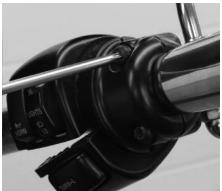
After positioning the clutch perch onto the 24 Carlini bars and against the switch housing, Dan uses the stock bolts and a T-27 Torx to loosely secure it to the bars.
