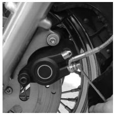
He then attaches the line to the stock brake caliper using a 12-point 3/8" wrench. After positioning the banjo so the line follows the same route as the stock line, Dan torques the bolt to 17-22 ft-lbs.
