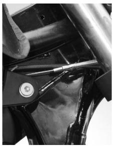
Before he pulled them out from under the gas tank, Dan tied a string to each of the old throttle cables so he could use the strings to pull the new Tec/Barnett stainless steel throttle cables through along the same route.
