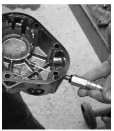
With the new Tec stainless steel clutch cable routed to the tranny, Dan slips a new O-ring onto the cable and then threads the new cable into the stock end cover. It's easy to cross thread this cable, so be careful.
