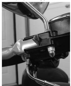
With a wedge of cardboard between the brake lever and its perch to prevent the lever from breaking the front brake light switch (it's in the switch housing), Dan installs the master cylinder.
