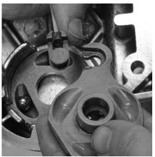
After attaching the stock cable holder onto the end of the new Tec/Barnett cable, Dan slips the stock inner ramp onto the holder and rotates it so the cable holder engages the ramp.
