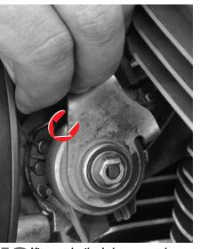
After removing the air cleaner cover using a 5/16" Allen, Dan attaches the new cables to the throttle wheel, first the pull cable and then the push cable, which goes into the top hole (arrow). This year bike does not use a spring on the push cable.
