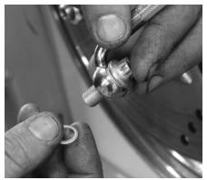
With a new Tec-supplied crush washer under the head of the stock banjo bolt, Dan slips the bolt into the banjo fitting on the new brake line, followed by another crush washer.
