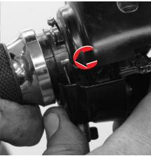
28 On the right switch housing, Dan connects the cables to the new H-D handgrip. The pull cable goes into the forward hole of the switch housing and in the lower hole (arrow) on the handgrip.
