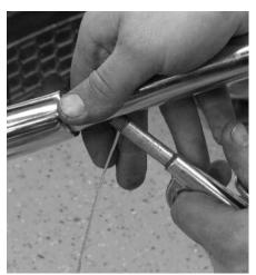
After covering the entire harness with the Tecsupplied shrink wrap, Dan blows a guide string through the bars. This string is to take up slack in the harness as it is fed into the bars, not to pull the harness through.
