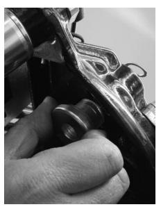
After putting a little WD-40 on them, Dan slips the lower part of the H-D riser bushing set (aluminum and neoprene) into the bottom of the top triple tree. Note: you'll have to turn the front end to get them in. good folks at TEC Distributing, the one-stop shop for the complicated aspect of installing apehangers, namely the wiring extensions, and stainless braided cables and brake lines. We told
