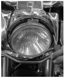
After sliding the headlight trim into place on top of the nacelle and reattaching the headlight connector, Dan reinstalls the headlight assembly using the stock seven screws and a Phillips screwdriver.
