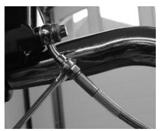
BO Once he has installed the Tec/Barnett upper front brake line from the brake line spider to the master cylinder following the stock route, Dan connects it using a 3/8" 12-point wrench and a 7/16" wrench.
