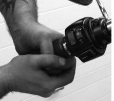
**25** Dan then pushes the new H-D chrome and rubber handgrip onto the bars until it reaches the switch housings. He then reinstalls the clutch lever using just its pivot pin.
