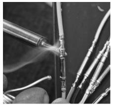
Dan now plugs the Tec switch harness extensions into the stock switch harnesses. Though they don't need to be, Dan also solders each connection before covering it with the Tec-supplied shrink wrap.
