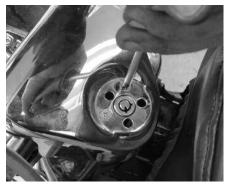
After securing all the wiring with wire-ties, Dan installs the riser cover using the two stock screws and a Phillips screwdriver. After aligning the front of both nacelle halves, he tightens the nacelle and spotlight nuts using a 1/2" socket.
