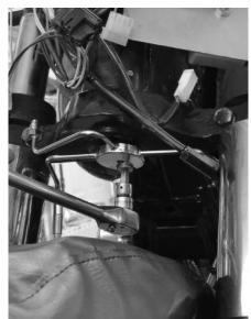
After putting wire-ties on the clutch and throttle cables, Dan attaches the Tec stainless steel brake line spider to the bottom of the bottom triple tree using the stock hardware, blue Loctite, and a T-40 Torx.
