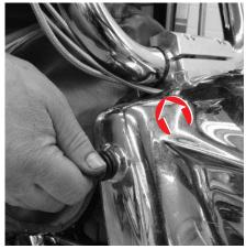
After reconnecting the nacelle's switches, Dan loosely installs the headlight nacelle using the stock washers and nuts. The throttle cables and brake line are routed through the riser opening (arrow) in the nacelle.
