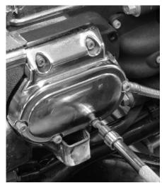
With a new gasket on the tranny, Dan reinstalls the end cover using the stock bolts, blue Loctite, and a 3/16" Allen. He torques the bolts to 100 in-lbs. up to the magnum sizing, which is a bit bigger than what he was used to. We also went with Harley's polyurethane riser isolators (#56298-03/\$29.85) so he would have a factory-quality
