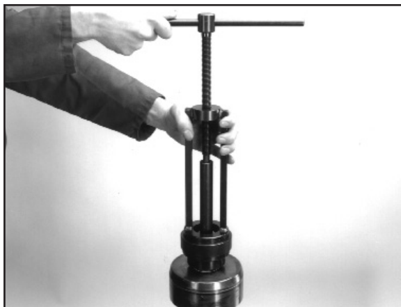
8.15 Invert the shaft and remove the front bearing using the appropriate tool. (Tool No. KM3516)
