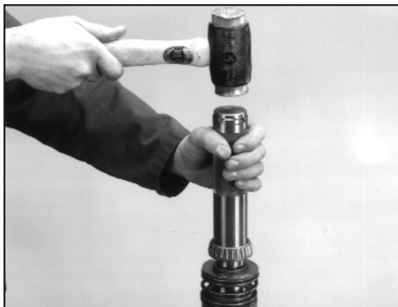
6:18 Using an appropriately sized tube refit the front bearing.
