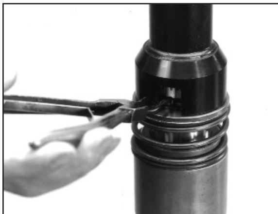
6:17 Using the appropriate tool compress the spring and retainer and refit the circlip. (Tool No.KM3523)
