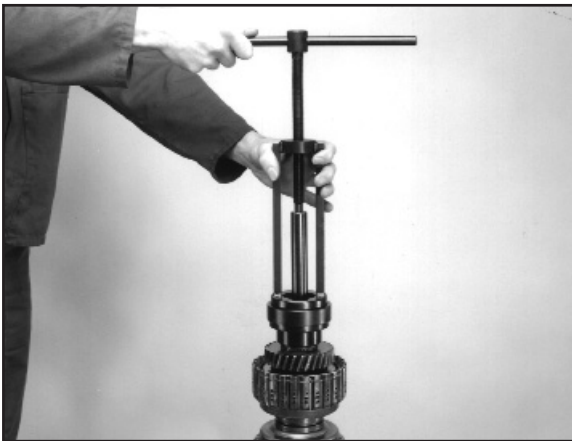
2:3 Using the appropriate bearing puller remove the rear bearing. (Tool No.KM3509)
