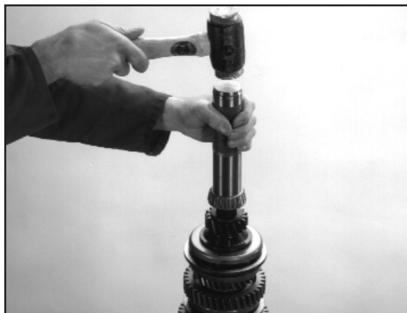
5:24 Using an appropriately sized tube replace the front bearing.
