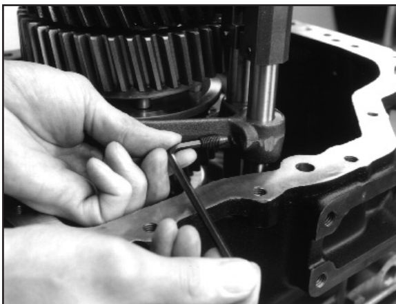
1:14 Ensure both synchronisers are in the neutral position then remove the 1st / 2nd shift fork screw.
