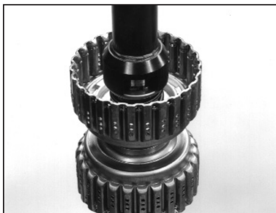
2:18 Using the appropriate tool compress the spring and locate the circlip into its groove. ( Tool No.KM3520)
