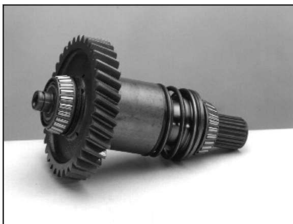
6:1 The hydraulic dog clutch 4 wheel drive assembly.
