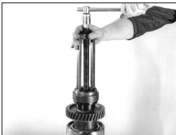
8:3 Using the appropriate tool remove the rear bearing. (Tool No.KM3516)
