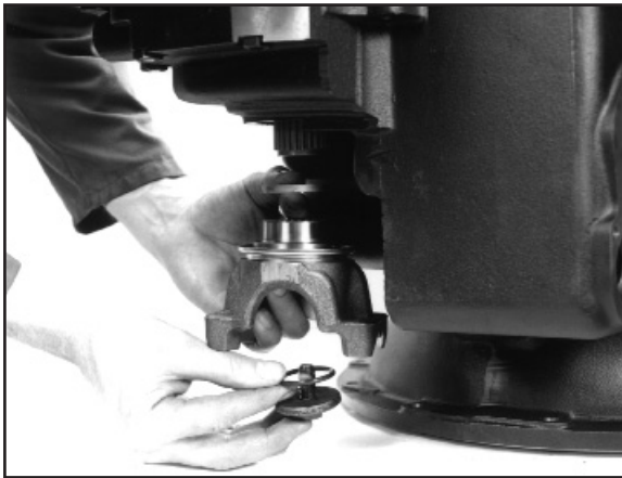
12:28 Replace the spacer, 4WD yoke, O ring, washer and bolt. Then tighten to a torque of 50 to 65 lb.ft.
