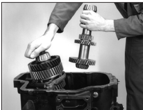
1:19 Remove the counter shaft assembly.
