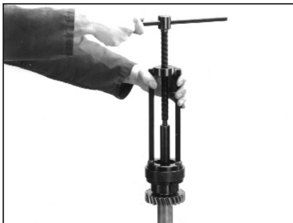
4:2 Using the appropriate bearing puller remove the front and rear bearings. (Tool No.KM3509)
