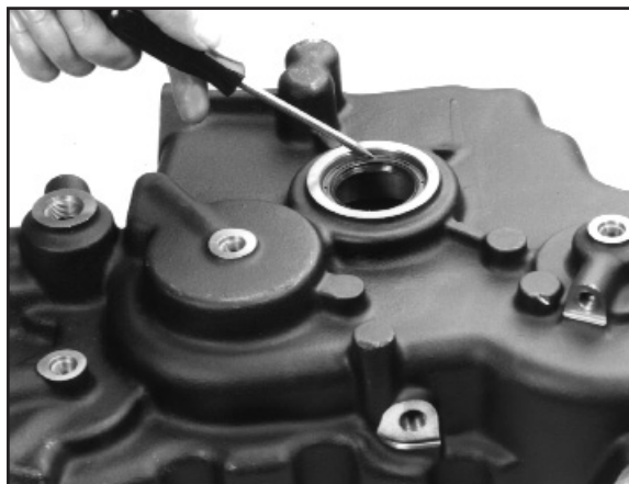
12:15 Position the rear case as shown and using a suitably sized tube fit a new output shaft oil seal to a depth of 6mm below the housing face. Fill the seal lip with a light grease.
