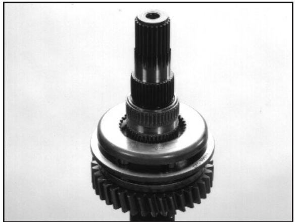
5:17 Replace the 1st gear needle bearings and spacer as shown.
