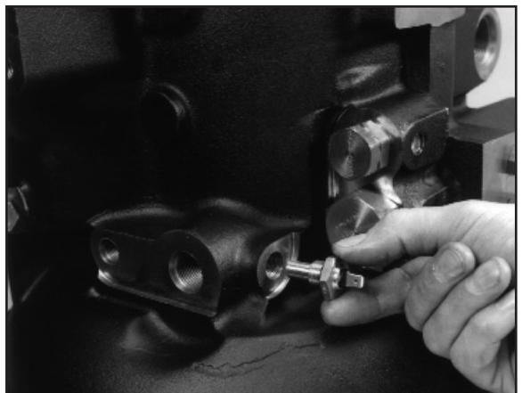
12:32 Refit the temperature sender and tighten to a torque of 15 to 20 lb.ft.
