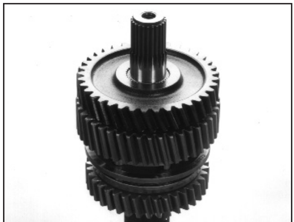
5:19 Replace the 4 wheel drive gear using Loctite 649 spline lock or equivalent.
