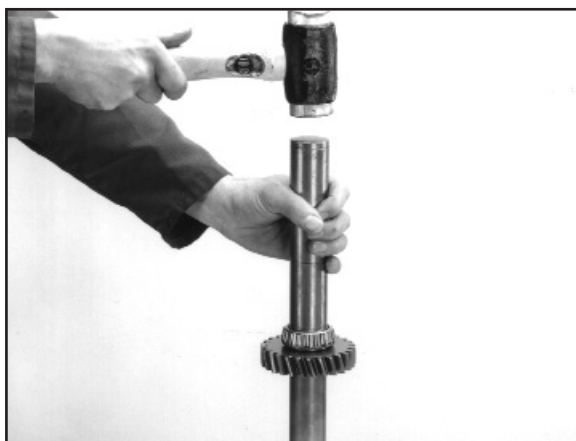
4:3 Using an appropriately sized tube replace the front and rear bearings.
