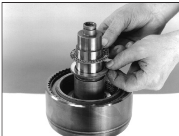
8:23 Refit the thrust washer and needle bearing.
