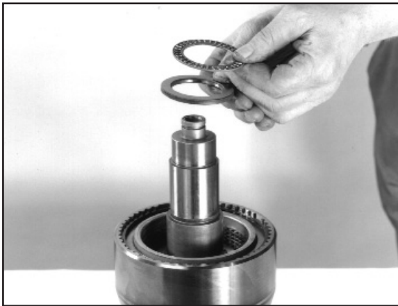
8:7 Remove the needle bearing and thrust washer.
