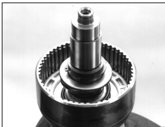
8:19 Lubricate the seals with a light grease and re-fit the piston into the clutch drum. Then replace the spring, retainer and circlip as shown.
