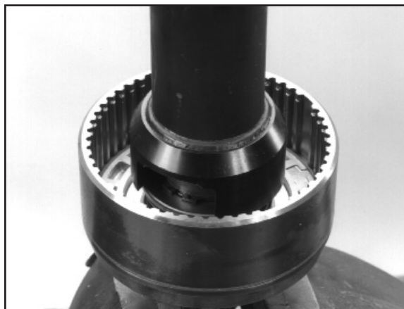
8:20 Using the appropriate tool compress the piston return spring and locate the circlip into its groove. (Tool No.KM3521)
