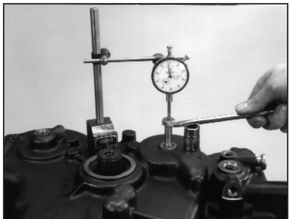
12:20 Attach a suitable shimming tool, (with a 12mm thread), to the end of the countershaft. Position a D.T.I. as shown, and using a pry bar lift the shaft, then measure and note the end float. (Tool No.KM3524)
