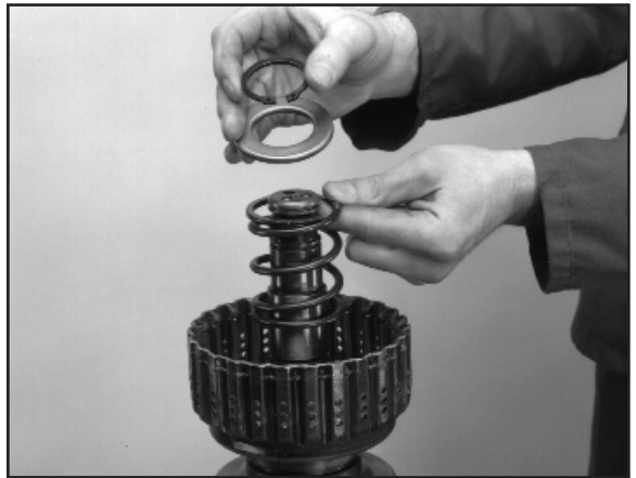
2:11 Remove the circlip, retainer and spring.
