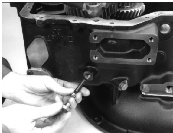
1:18 Remove the detent plug, inner detent ball and spring.
