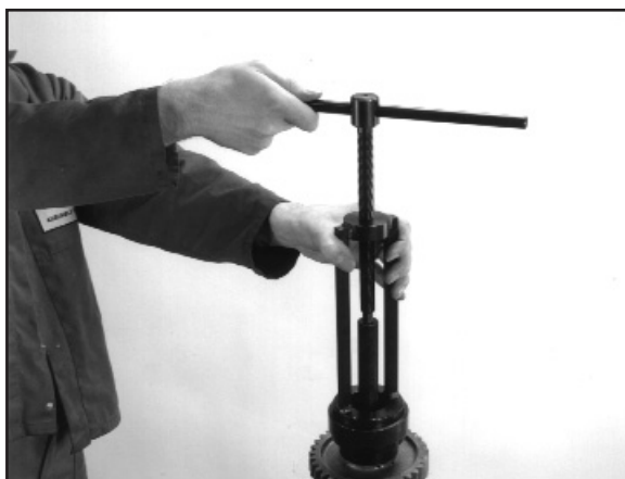
6:3 Using the appropriate bearing puller remove the rear bearing. (Tool No.KM3516)
