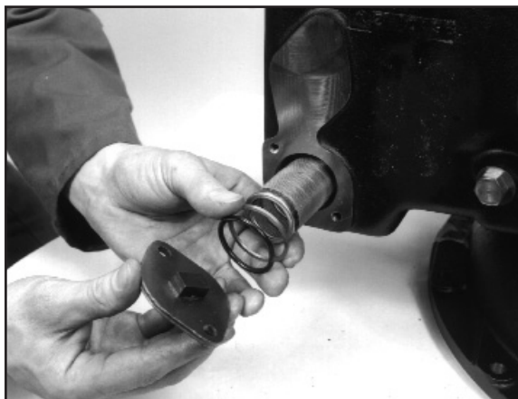
1:23 Remove 2 screws and withdraw the strainer cover, O ring, spacer and strainer.
