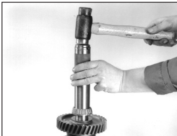
8:27 Using an appropriately sized tube re-fit the rear bearing.
