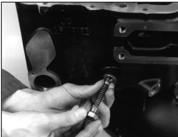
12:11 Replace the outer detent ball and spring. Tighten the plug to a torque of 30 to 40 lb.ft.
