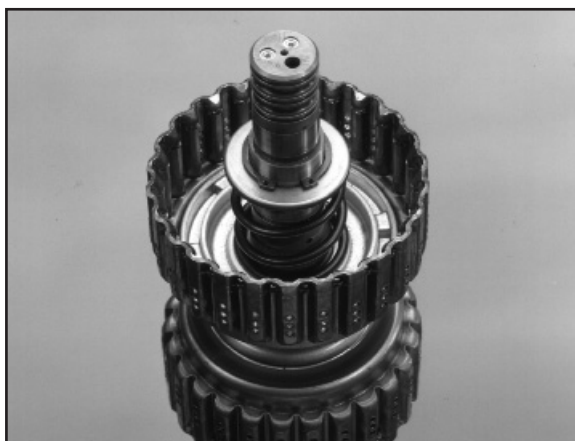
2:17 Replace the spring , retainer and circlip as shown.
