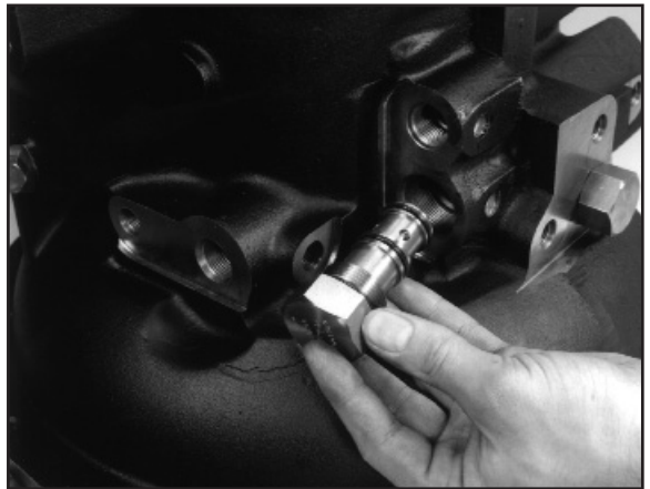
12:30 Lubricate the seals with transmission fluid then re-fit the pressure regulator valve and tighten to a torque of 34 to 44 lb.ft.
