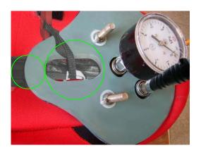
3. Check carefully if any bubbles appear from the Immersion Suit4. It is normal that the bubbles appear in the zipper and mark properly the leaking areas of the suit.
