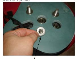
5. Install the o-ring gasket and tighten up the butterfly nut so as to eliminate leakage around the face seal.
