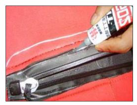
2. Apply a gentle amount of glue on the marked leaking areas. Let it dry for 8-10 minutes. Then apply once again, a glue layer on the immersion suit damaged area. Leave the immersion suit till the next day for the next use.
