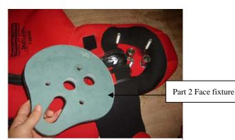
3. Place part 2 face fixture on part 2, by adjusting its holes carefully through the bolts and joints.
