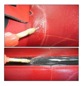
2. Sprinkle along seams and closures of the immersion suit with a soapy water solution.
