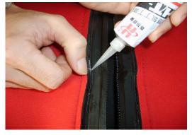
2. Let it dry for 8-10 minutes. Then apply, once again, a glue layer on both sides of Immersion suit's damaged area.
