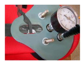
1. Provide air into the suit, through the foot pump, to a pressure of 0,7 to 1,4Kpa (0.1 to 0,2psi) [acc. MSC/Circ.1114.] Maintain the pressure to those limits for the air-test.
