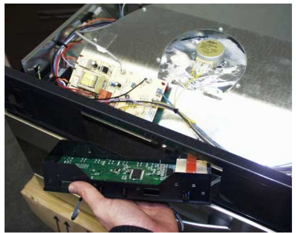
Fig.: Input electronic in installed condition and disassembling after unlocking
