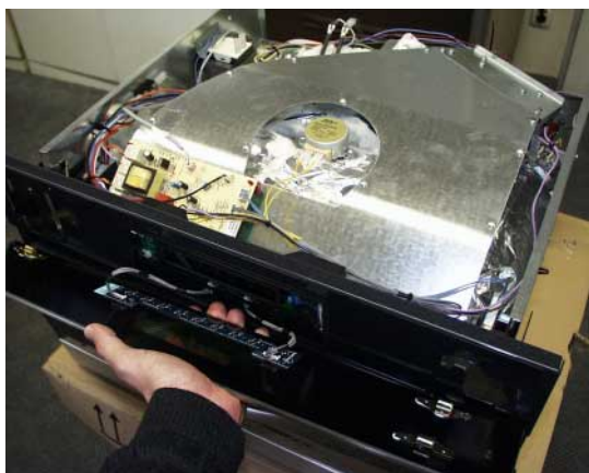
Fig.: Switch panel after disassembly
