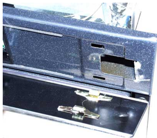
Fig.: Support springs switch panel
