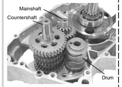
4 . Apply engine oil to pawls on each shift fork, 5 . and fit the forks into grooves on each gear.
