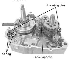
Fix screws on the crankcase, and screw them up in the numerical order.
