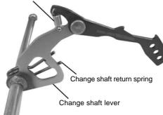
1 1 . Attach the change shaft lever to the crankcase.
