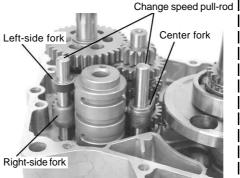
Pay attention to the location of each fork. Apply engine oil to a change speed pull-rod, and moving each shift fork, put in the rod to attach it to a case.
