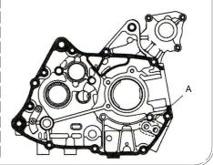
7 . Fix two locating pins and O-ring to the crankcase. Attach a stock spacer to the mainshaft. And attach the processed left crankcase, and join a right and left crankcases together by hitting them with a plastic hammer.
