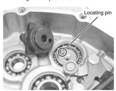
Change the spring with a provided spring. Aligning a hole on the shift drum cam with the locating pin on the drum, fix a cam. Put five shift drum cam pins into the drum cam with its tapered portion pointing down.
