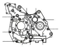
8 . Attach a spring and pin to the shift drum. Attach an O-ring to a neutral switch, and attach the switch to the case.
