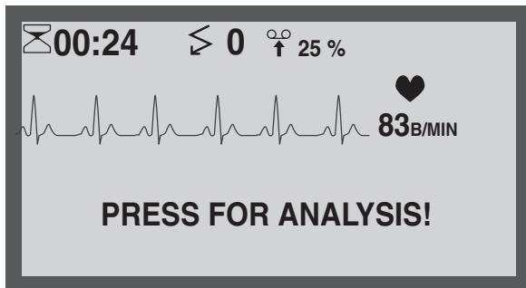
Figure 6-1. Screen with ECG waveform, heart rate and QRS blip
