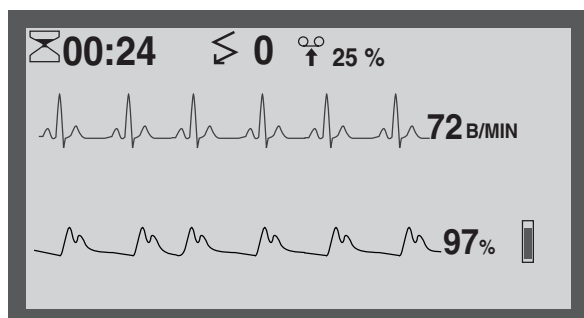
Figure 6-12. SpO 2 window on the display (semi-automatic mode, "ECG Display" option installed)
