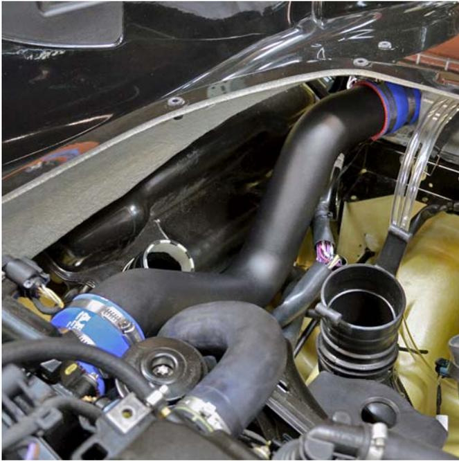
Install recommended Blow-off Valve onto supercharger to intercooler tube (see instructions provided with Blow-off Valve Kit). **Note direction and angle as shown below.**
