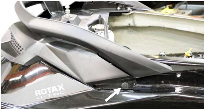
Remove coolant overflow reservoir. Remove grab handle (6 bolts).
