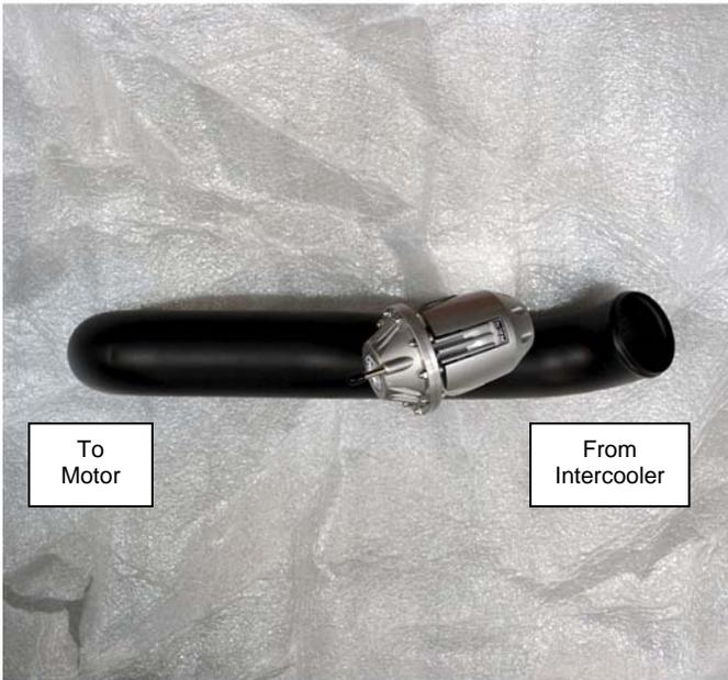
Install supercharger to intercooler tube. Secure with supplied clamps and stock clamps. **NOTE: Do not over tighten clamps.**
