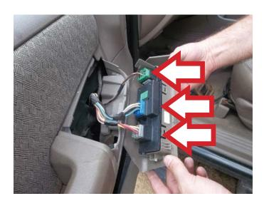
**STEP 11:** Attach the power switch assembly.
