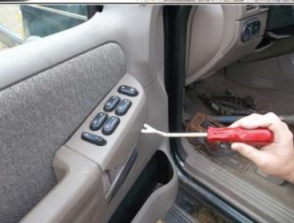
**STEP 3:** Disconnect the power switch assembly.
