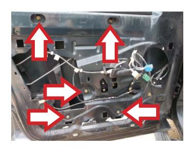
**STEP 13:** Remove the window regulator assembly through the main access hole.
