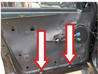
**STEP 9:** Using a 6mm socket and ratchet assembly, attach the two (2) interior door trim panel retaining screws.
