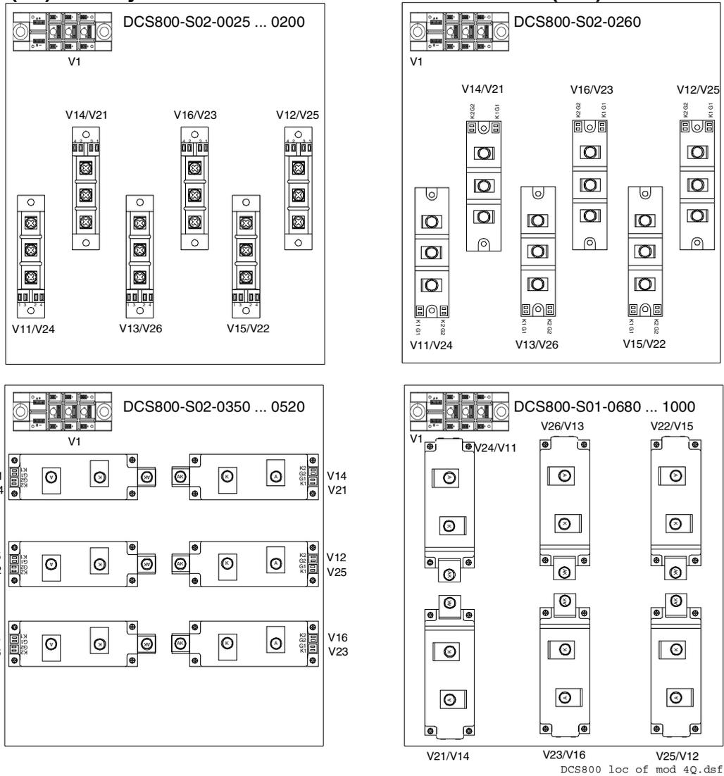
*Location of the OnBoard bridge and thyristor modules in DCS800-S02 (4-Q) units*
