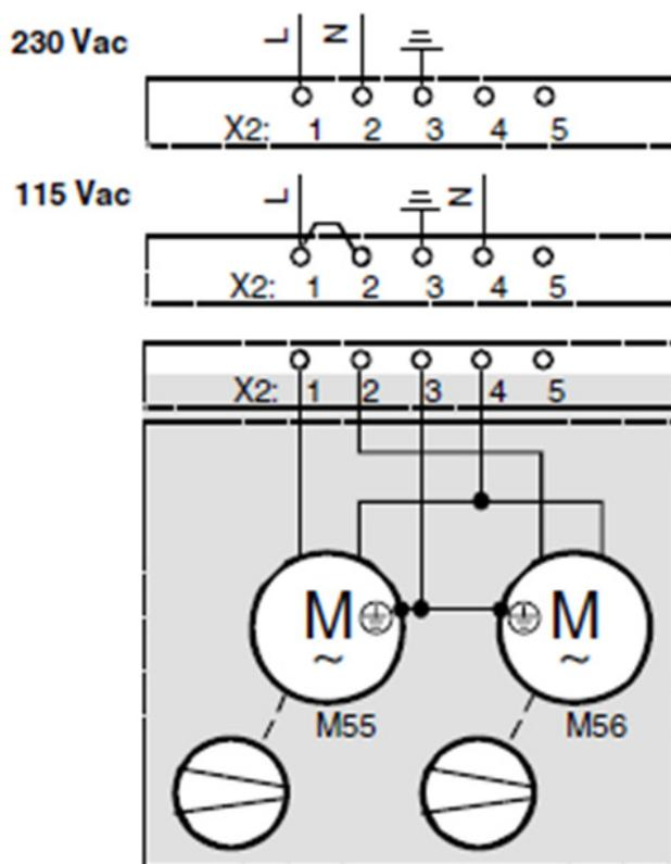
Connector X2 on top of converter housing
