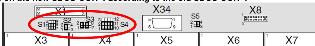
Copy the jumper settings (S1 to S4) of the old SDCS-CON-4 onto the new SDCS-CON-4 accordingly.
