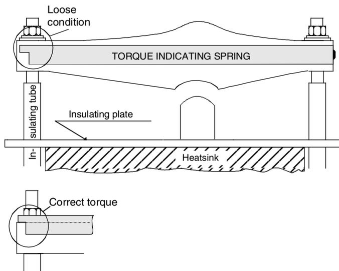
*Aluminum spring with welded indicating spring*
