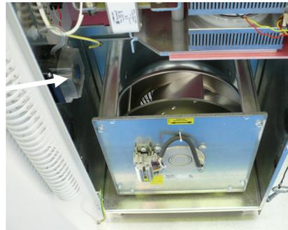
*Cooling air pressure switch*
