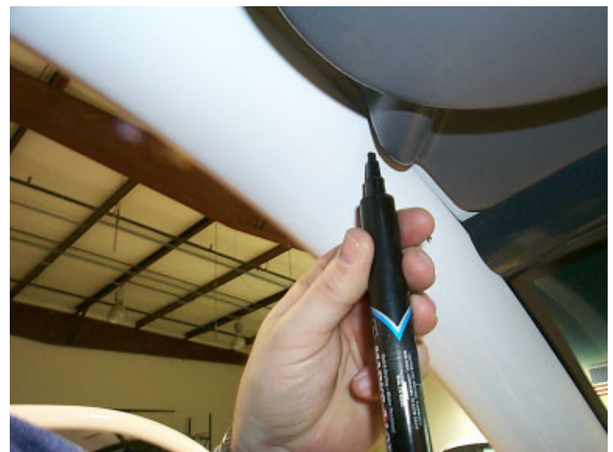
Fig. # 8 Mark hole locations for wiring harness
