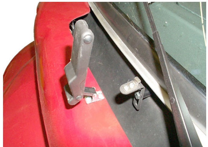
Fig. # 3 unclasp latch
