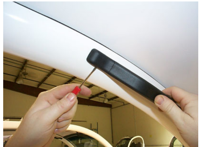
Fig. # 7 Remove grab handles
