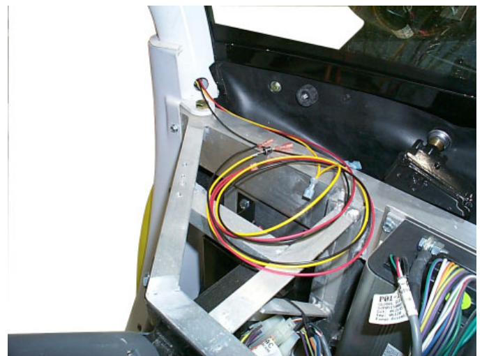
Fig. # 13 Route wiring harness
