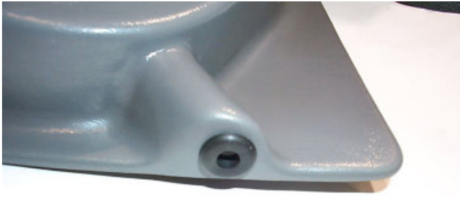
Fig. # 9 Drill Ø3/8" hole in stereo console and install rubber grommet
