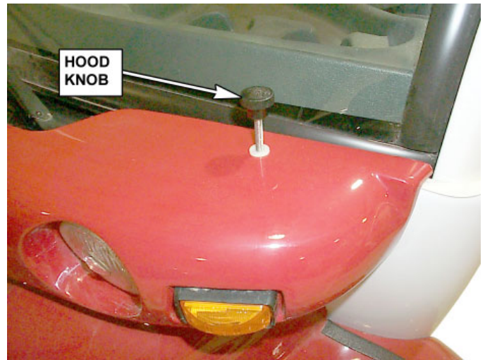
Fig. # 2 Loosen and remove hood knobs
