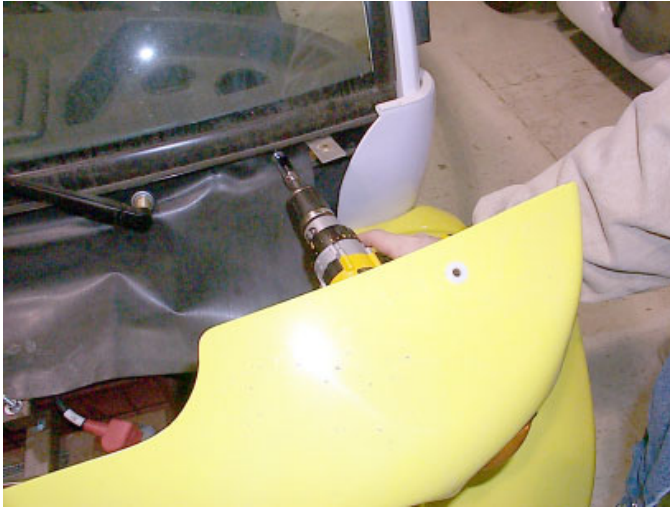
Fig. # 4 Loosen dash mount bolts
