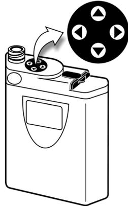
View the navigation buttons from the top of the monitor with the display facing you.
