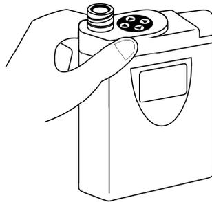
Once you have navigated to a menu with variables, press the response buttons to put the monitor into edit mode. Response buttons light when the monitor is in edit mode.
