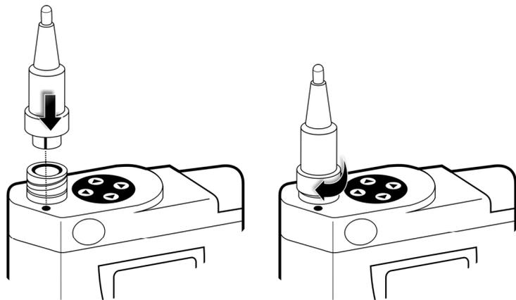
Leave the test plug connected until the test is complete.
