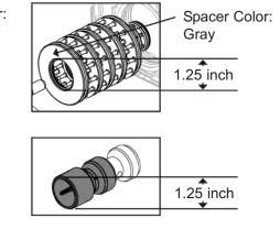
NOTE: The WS1CS downflow piston is a solid amber color. The WS1CS upflow piston is black and amber.
