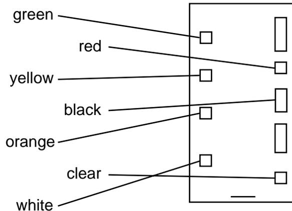
Figure 4.9.8 SpO<sub>2</sub> jack, wire side4.9.9 Replacing the SpO<sub>2</sub> board.
