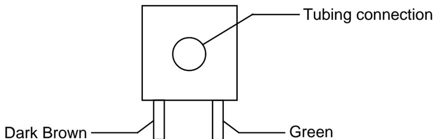
Figure 4.12.7 bottom view of valve (pneutronics)
