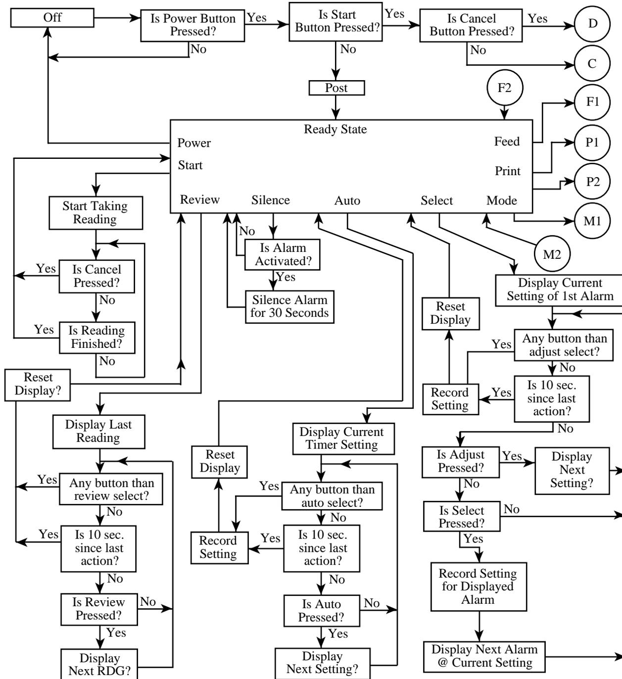
**Figure 1.5 Block Diagram of Unit Operation**
