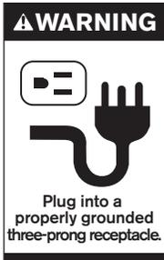
The Keating Custom Pasta Gas System is equipped with a 9' neoprene covered, 3 wire electrical cord with a three-pronged grounded plug for protection against electrical shock. This plug must be placed into a 120V properly grounded three-pronged outlet (NEMA 5-15 or 5-20). For proper grounding procedures see local codes or, in the absence of
