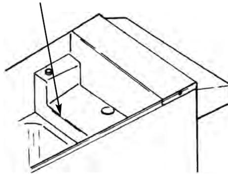
When the water fill toggle switch (located between the green and blue indicating lights) is turned on, the Pasta System vessel automatically will be filled to the proper level. If the vessel is being manually filled with water from a faucet or through the manual fill button, fill to just below the overflow deck. The black manual fill button is located to the right of the blue water fill indicating light.
