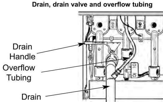
2. Slowly turn handle. The drain valve will be completely open after 1/4 turn.
