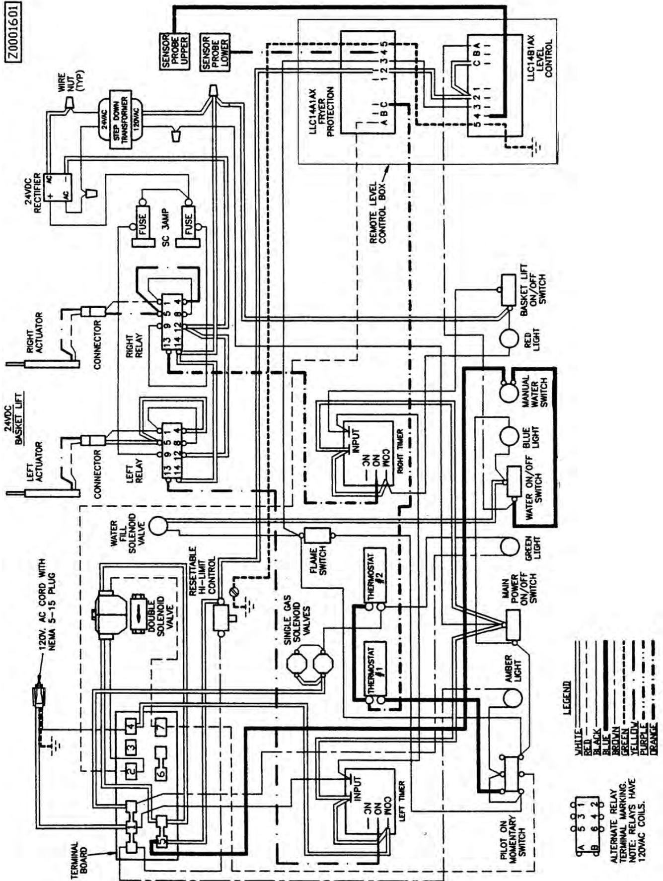
**GAS PASTA SYSTEM WITH BASKET-LIFT WIRING DIAGRAM (2007 MODEL)**
