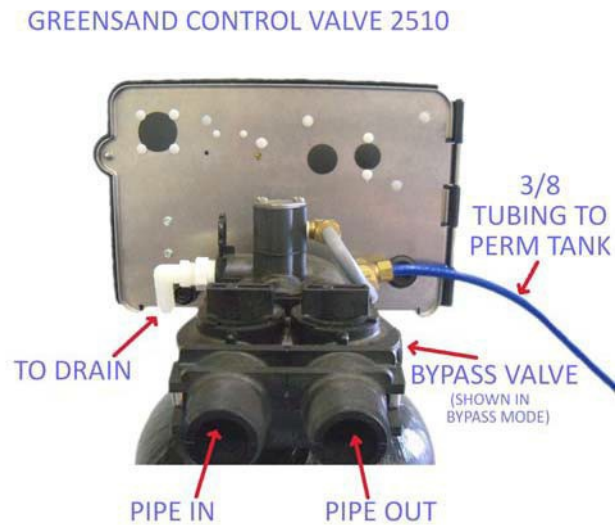
Fig 3: Fleck 2510 from the rear showing the inlet and outlet end-connector fittings 1" or 1-1/4" NPT in Noryl plastic. Brass end-connectors are also available for connecting to copper tubing.
