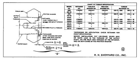
WHEN INSTALLING THE PITMAN ARM AND RETAINER ASSEMBLY, ALIGN THE TABS OF THE RETAINER WITH THE TWO NOTCHES IN THE PITMAN ARM. HAND TORQUE THE RETAINER TO THE VALUE SHOWN IN CHART "A" ABOVE. REMOVE THE RETAINER AND MEASURE THE DISTANCE FROM THE END OF THE SHAFT TO THE RECESSED AREA OF THE PITMAN ARM. THE ACCEPTABLE DIMENSIONS ARE LISTED IN "B" ABOVE. IF THESE DIMENSIONS ARE NOT ACHIEVED, REPLACE THE PITMAN ARM AND OUTPUT/SECTOR
