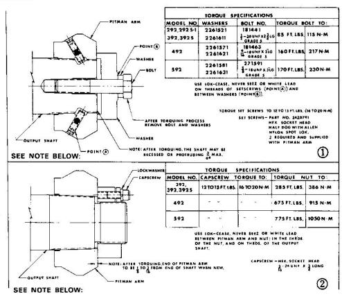
NOTE: WHENEVER A PITMAN ARM IS INSTALLED A MEASUREMENT MUST BE TAKEN FROM THE END OF THE SHAFT TO THE FACE OF THE PITMAN ARM, THIS SHOULD BE TAKEN AFTER THE ARM HAS BEEN TORQUED TO THE PROPER SPECIFICATION AND THE INSTALLATION TOOL OR NUT HAS BEEN REMOVED. IF THE NUT STYLE RETENTION IS USED ②, RETORQUING IS REQUIRED.
