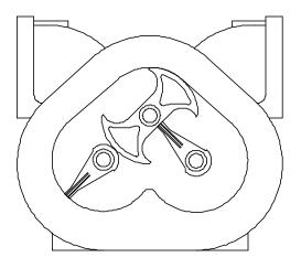
The rotors in the meter are designed to operate at close tolerances to one another and the wall of the fluid chamber. There are slight gaps between the rotors and the chamber wall. Because of this, it is important that the meter be properly applied for the flow rate and operating pressure of the system.
