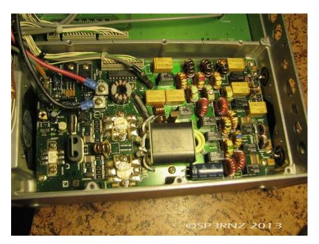
To do the mod we must pull the PCB out of chassis, so let's start with unscrewing all necessary screws, all of them including transistor screws. Then we should disconnect two HF outputs on the rear. Be careful, as these pins need to be bend a bit to suck the solder out.
