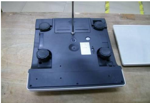
2. Put the scale upside down, Loosen and remove the screw on the battery cover.
