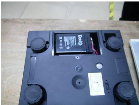
6. Put the rechargeable battery in the chamber with literal side upward and the wire to the right side.
