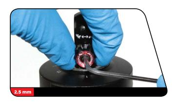
Refer to the rebound and damper settings that you wrote down for your shock at the beginning of the service. Set each adjuster to the recorded number of clicks/turns and fill the air can to the desired pressure.
