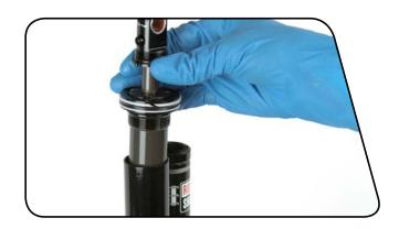
Remove the shock from the vise and pour the fluid from the damper body into an oil pan.
