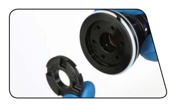
Remove and replace the two seal head glide rings and the quad seal.
