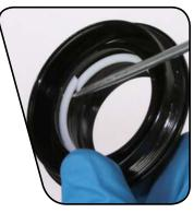
Use a pick to remove and replace the o-ring located just below the threads on the outside of the air can collar. Spray isopropyl alcohol on the air can collar and clean it with a rag.
