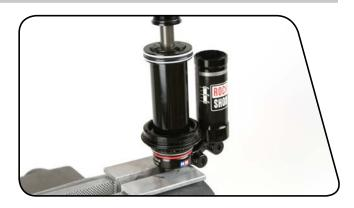
Hold the bottom out bumper away from the seal head and insert the RockShox Vivid 24 mm Spanner Wrench into the pin holes of the seal head. Turn the spanner wrench counter-clockwise to remove the seal head from the damper body.
