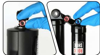
Record the air can clocking number that is in line with the Beginning Stroke Rebound knob on your shock to assist with air can reassembly. Also take note of how the air can and Beginning Stroke Rebound knob are positioned relative to the IFP reservoir.
