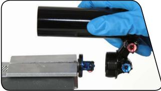
Insert a 2 mm hex wrench into the nut side of the compression valve to push out the compression needle.
