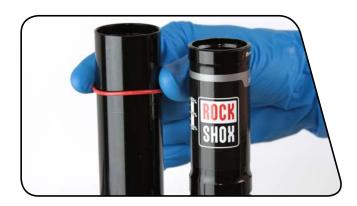
Grease the inside of the air can collar and begin to install it, with the threaded side up, at an angle onto the damper body. Push the quad seal with your finger as you install the collar to prevent it from getting pinched. Slide the collar down the damper body.
