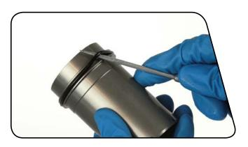
Remove and replace the air can o-ring, located inside the large opening of the air can, just above the internal threads.
