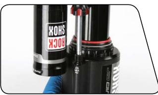
4 Use a T10 TORX® wrench to remove the IFP reservoir fill cap. Use a small hex wrench or pick to depress the Schrader valve and release all air pressure from the IFP reservoir.
