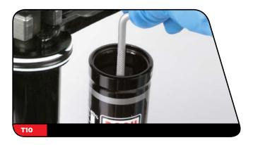
Use a 3 mm hex wrench to loosen the lower stop bolt of the Compressor and remove it from the shaft assembly.
