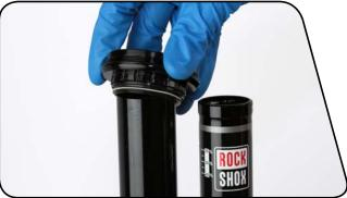
**7** Remove and replace the crush washer on the damper tube centering ring.
