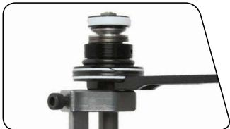
Insert the shaft assembly into the damper body at a 45 degree angle, while rotating the piston into the fluid in the damper body.
