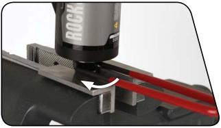
Remove the shock from the vise and remove the lock ring from the shaft eyelet by hand.
