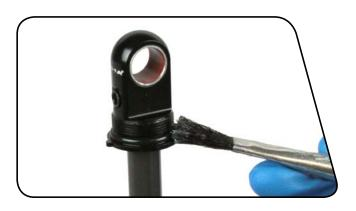
Apply a liberal amount of Parker  $^{\circledR}$  O-Lube to the air can collar quad seal and glide rings.
