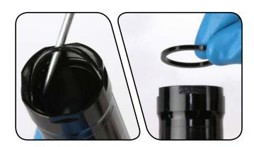
Use a T10 TORX® wrench to remove the IFP bleed screw.
