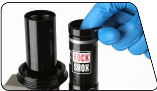
Keep the damper body covered with your hand and use a T10 TORX® wrench to install the bleed screw into the bleed port and tighten it until the IFP begins to spin.
