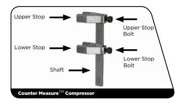
Position the Counter Measure<sup>™</sup> Compressor onto the shaft assembly as shown. Pull the upper and lower stops away from each other to clamp the spanner wrench into the seal head. Use a 3 mm hex wrench to tighten the upper stop bolt.
