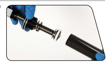
Remove and replace the shaft eyelet o-ring, located at the base of the threads on the shaft eyelet.
