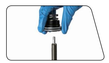
**7** Remove the bottom out bumper from the seal head.
