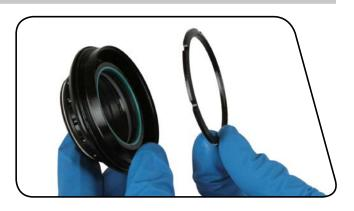
Thread the air can collar into the top of the air can by hand until it stops. Use a flathead screwdriver to pry the dust wiper seal out of the air can collar. Remove the air can collar from the air can by hand.
