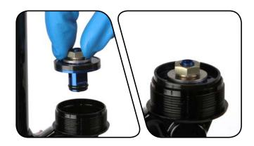
Thread the IFP reservoir onto the body eyelet by hand. Use a 31 mm flat wrench to tighten the IFP reservoir to 11.3 N·m (100 in-lb). There will be a small, visible gap between the IFP reservoir and the body eyelet. This is ok.
