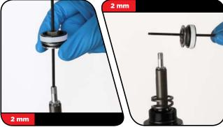
Remove the seal head from the shaft by hand.
