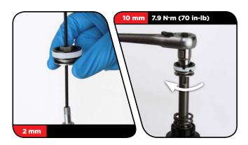
Remove the shaft assembly from the vise.
