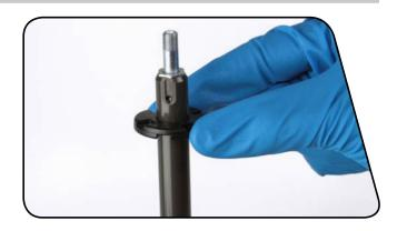
Grease the interior of the seal head and install it onto the shaft assembly with the Counter Measure™ Spring oriented upward.
