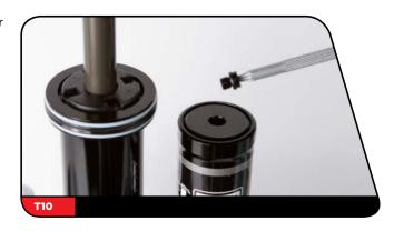
Spray the entire shock with isopropyl alcohol and clean it with a rag.
