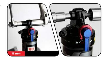
Unthread the catcher from the threaded rod and remove the tool from the shaft eyelet.
