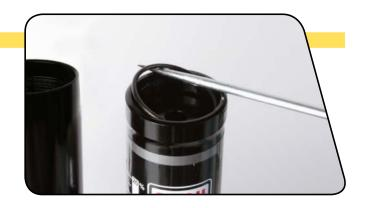
Thread the Vivid Pump Adapter into a shock pump. Thread the pump and Vivid Pump Adapter into the IFP reservoir cap. Pull up on the pump and rock it side to side to remove the reservoir cap from the IFP reservoir. Remove the reservoir cap assembly from the pump/adapter.
