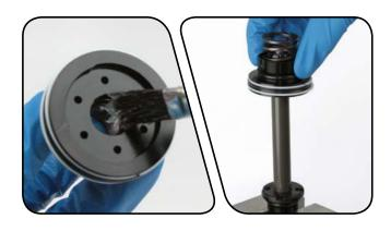
Use the 2 mm hex wrench to install the piston assembly onto the shaft. Use a torque wrench with a 10 mm socket to tighten the nut to 7.9 N·m (70 in-lb).
