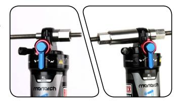
Clamp the catcher in a vise or hold it secure with a 13 mm wrench.
