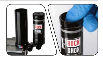
Use a pick to remove the retention clip from the IFP reservoir.
