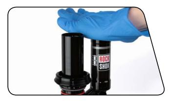
Install the IFP, flat side up, into the reservoir. Use your thumb to evenly and slowly push the IFP into the reservoir just past the step in the reservoir.
