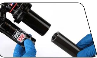
2 Clamp the body eyelet into the vise. Install the air can centering ring onto the air can collar with the chamfered, stepped side facing upward.
