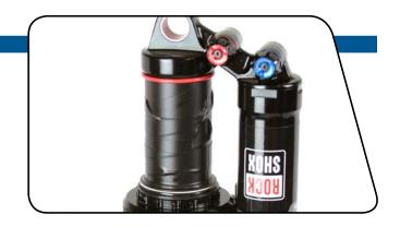
2 Clamp the RockShox Vivid Air Can Wrench into a vise. Place the air can into the wrench. Use the bottom bracket tool to turn the air can collar counter-clockwise and remove it from the air can. Remove the shock and the wrench from the vise.
