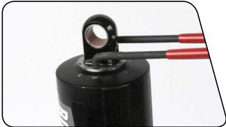
Position the pin spanner into the lock ring, then clamp the shock by the shaft eyelet into the vise, leaving just enough room for the spanner to rotate. Use the spanner to tighten the lock ring to  $22.6 \text{ N} \cdot \text{m}$  (200 in-lb). Remove the shock and spanner from the vise.
