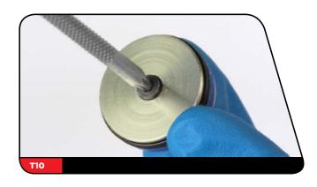
Remove and replace the IFP bleed screw o-ring.
