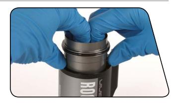
Remove and replace the air can inner sleeve o-ring.
