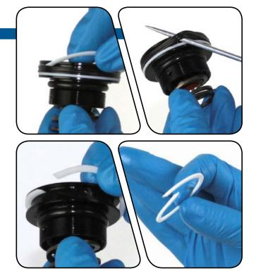
9 Use a pick to remove and replace the o-ring located in the interior of the seal head and the o-ring located on the outside of the seal head.
