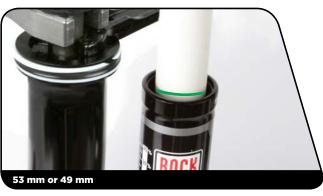
Use a T10  $\mathsf{TORX}^{\ensuremath{\mathbb{R}}}$  wrench to install the bleed screw into the bleed port and tighten it until the IFP begins to spin.
