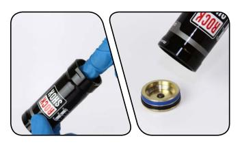
Remove and replace the IFP quad seal and glide ring.
