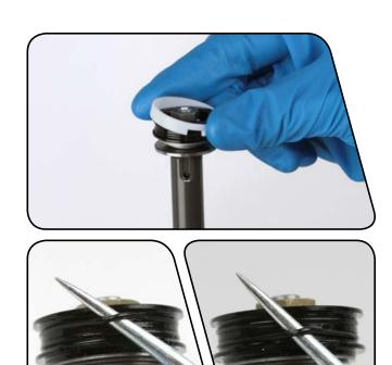
Use a socket wrench with a 10 mm socket to unthread the piston nut. Insert a 2 mm hex wrench through the piston nut and into the piston bolt, main piston, and shim stack washers. Keeping all parts together, carefully remove the piston assembly and hex wrench from the shaft and set it aside.
