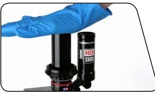
Once most of the fluid from the damper body has moved to the reservoir, use the palm of your hand to tap downward on the top of the reservoir repeatedly to move fluid back into the damper body. This will further assist in purging air bubbles from the system.
