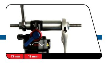
Reinsert the threaded rod and push pin through the shaft eyelet.
