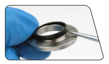
Place the damper tube centering ring onto the end of the damper tube that does not have holes. Hold the shock with the damper body opening facing downward. Insert the damper tube into the damper body and rotate it until the centering ring is seated in its groove.
