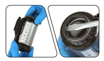
Place a new dust wiper seal onto the end of a seal press tool as shown. Use the seal press tool to install the dust wiper seal into the smaller opening of the air can collar until there is no gap between the dust wiper seal and the air can collar.
