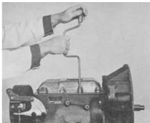
Figure 2-Remove shift rod cover capscrews. NOTE: See Page 23 for Diecast Cover Disassembly
