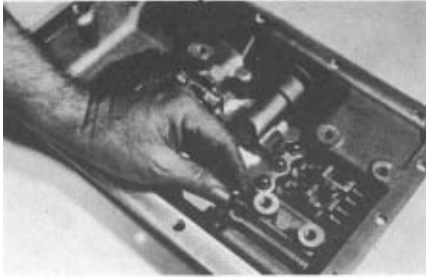
Figure 101 - Remove mesh lock poppet balls, quantity 4.
