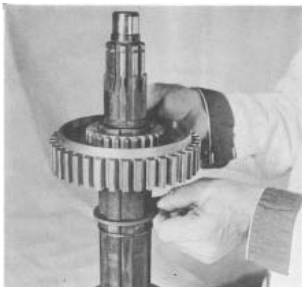
Figure 33 - Remove 2nd gear and locating washer.
