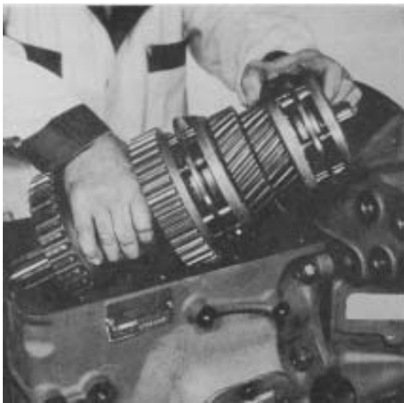
Figure 18 -Remove mainshaft assembly
