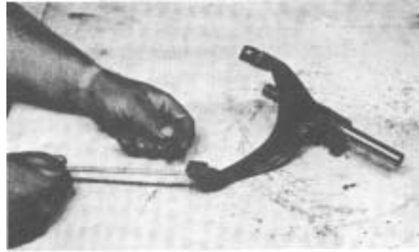
Figure 10 - If the second, third, fourth or fifth shift fork bushing is to be replaced, remove worn bushings from fork. Install new bushing and bend bushings tab over top and bottom of fork.
