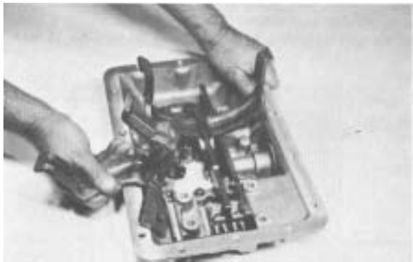
Figure 116 - Position 4th & 5th shift fork and rail on poppet ball in neutral.
