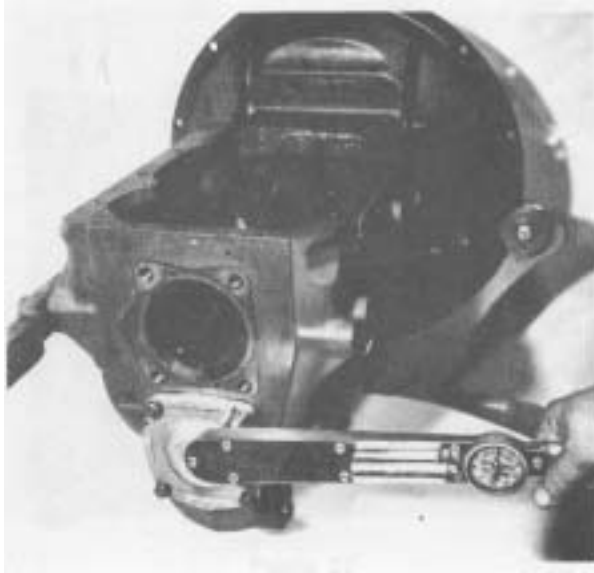
Figure 65 - Coat a new gasket on both sides with a grade #2 multi-purpose grease. Position
