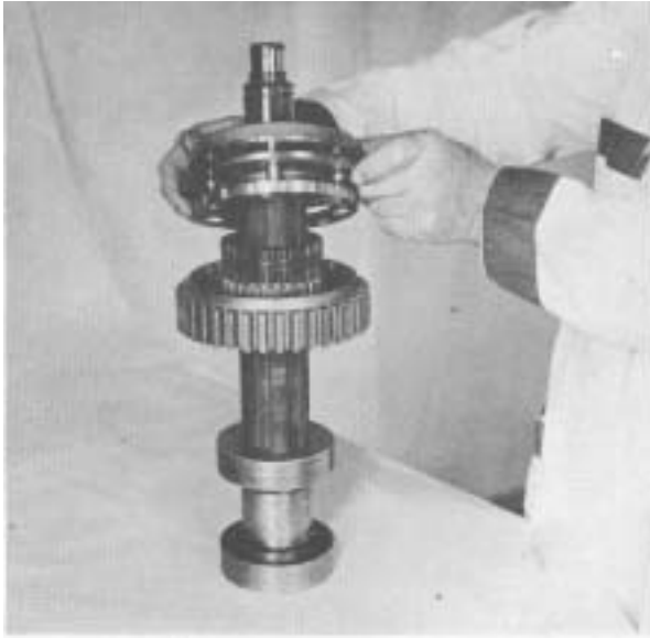
Figure 29 - Remove 2nd & 3rd synchronizer assembly.
