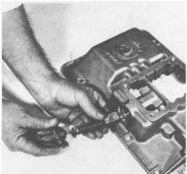
Figure 105 - Remove reverse latch plunger spring and plunger.
