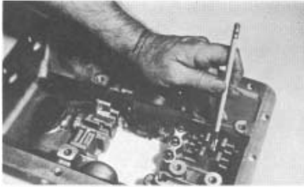
Figure 112 - Note position of tapered interlock cross pin in relation to rail.
