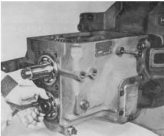
Figure 13 -Remove countershaft rear bearing cap.
