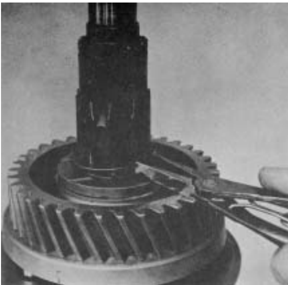
Figure 26 - Remove 4th & 5th shift hub sleeve and 4th speed gear.
