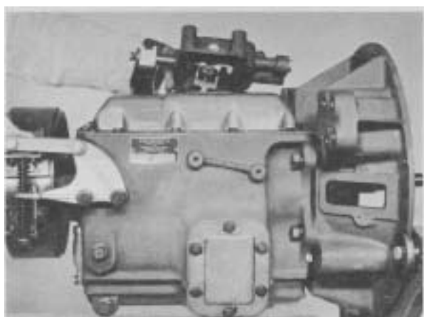
Figure 1-Remove control top or remote control assembly.
