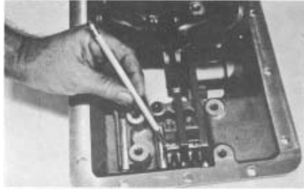
Figure 115 - Install 2nd interlock tapered pin. Align pin with interlock cross pin hole.
