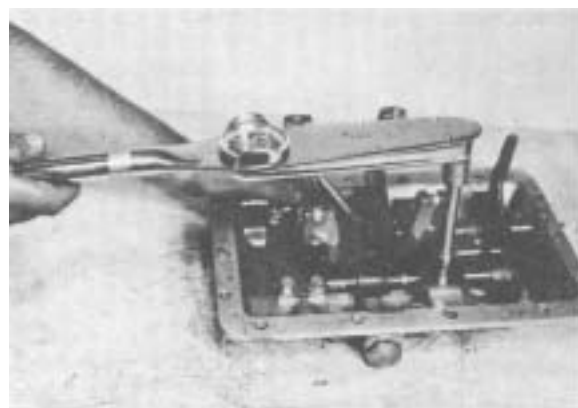
Figure 21 - Tighten support cap screws 20 to 25 ft. lbs. torque [27,2 - 33,8 N.m].
