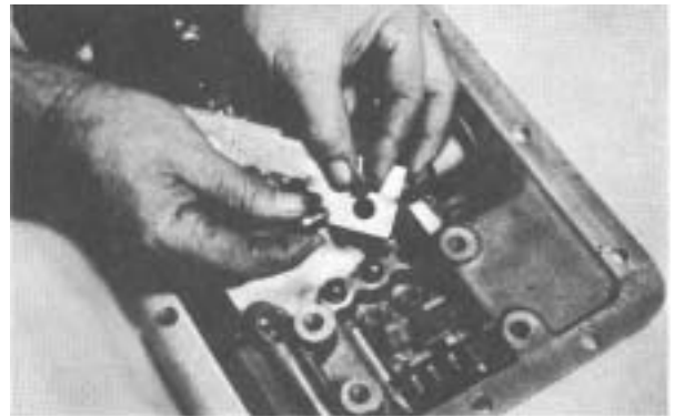
Figure 99 - Use caution as not to lose interlock cross pin, interlock tapered pins or mesh lock poppet balls.
