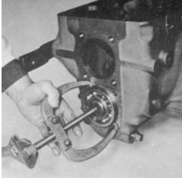
Figure 21 -Pry countershaft to the rear to expose rear bearing.
