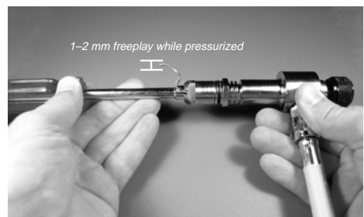
Fig. 9 – Lever Height Adjustment
