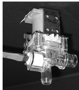
Figure 1. Adjusting Valve
