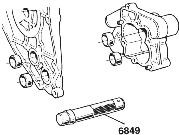
Press the bushes out of the bracket and the pump housing, using mandrel no. 6849.
