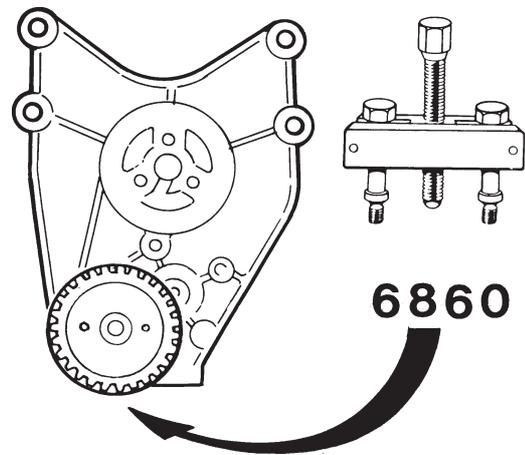
Pull the oil pump gear off the shaft, using extractor 6860.
