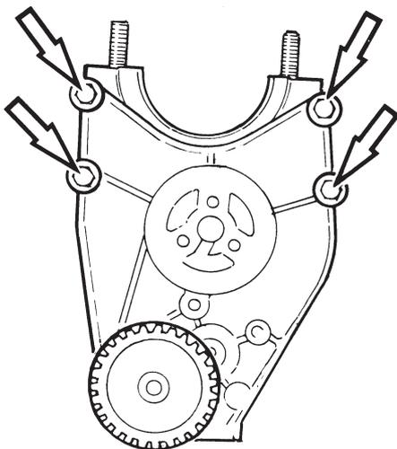
Screw the main bearing cap to the oil pump bracket.
