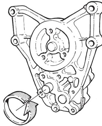
Move the gear wheels over to the bracket. Install the pump housing and tighten the screws. Check that the pump gears move easily and do not catch on each other, by turning the pump shaft a **complete turn**.
