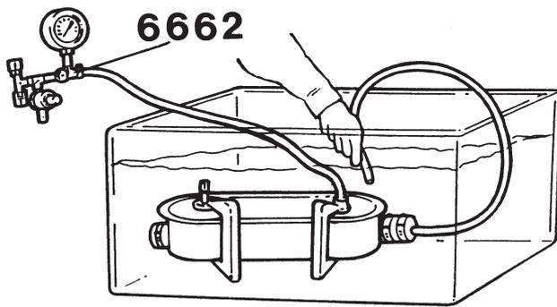
Connect the hose connection from pressure testing equipment no. 6662 to 6845.
