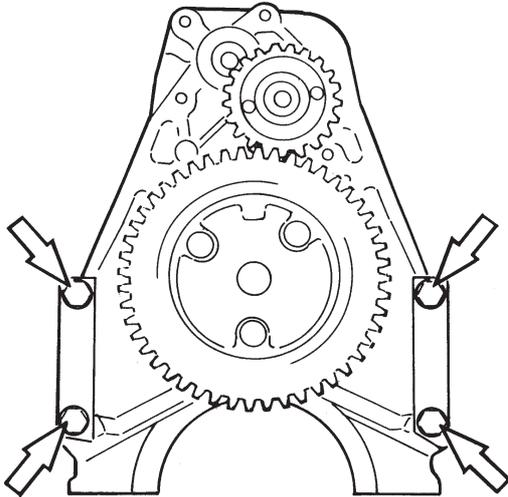
Remove the bearing cap from the oil pump bracket.
