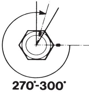
Tighten the unions **270–300°** for new pipes. Pipes which have previously been installed shall only be tightened **60°**.
