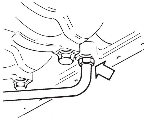
Undo the oil supply pipe and the brackets from the cylinder block. Remove the pipes and brackets.
