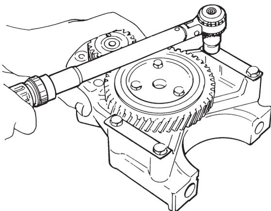
Screw the bearing cap to the oil pump bracket.
