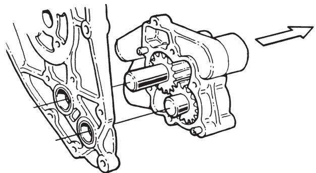
Undo and remove the screws which hold the pump housing.
