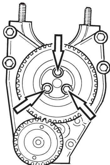
Install the idler gear and torque the screws to **33 Nm (3.3 kpm)**.
