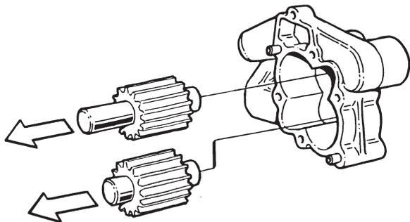
Remove the pump gears from the housing
