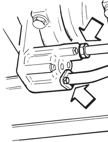
Undo the suction and oil supply pipes from the oil pump.
