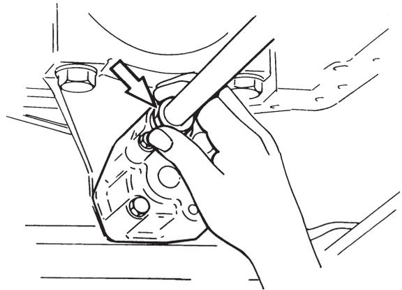
Install the oil supply pipe on the pump and the cylinder block.
