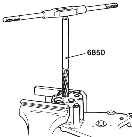
Ream the bushes in the pump housing, using tool no. 6850.
