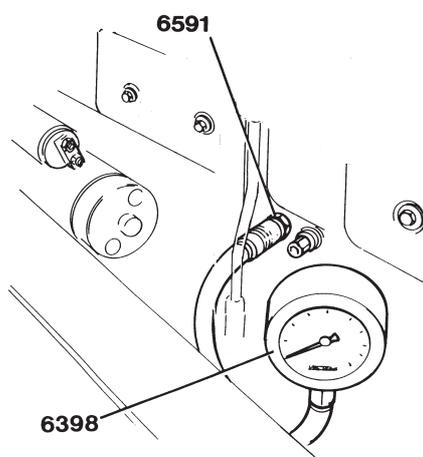
Install nipple 6571 and connect pressure gauge 6398 to the nipple.
