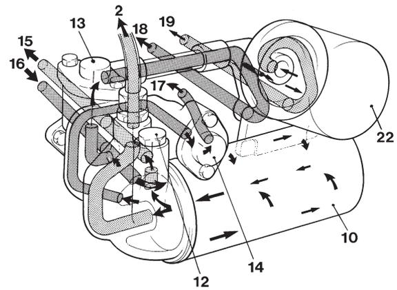
Lubrication system (detail illustration of filter housing) TAMD 63
