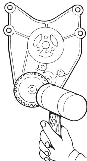
Heat the oil pump gear to **180±20°C** and tap the gear onto the shaft with a plastic-faced hammer.
