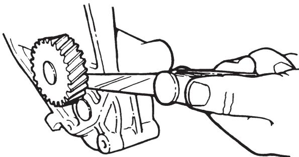
Check that the clearance between the bracket and gear wheel is **1.0–1.5 mm**.
