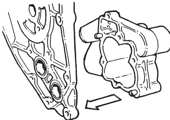
Screw the pump housing to the bracket, to provide support for reaming the bushings.
