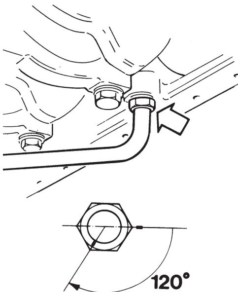
Tighten the union on the cylinder block **120°** for new pipes. Pipes which have previously been installed shall only be tightened **60°**.
