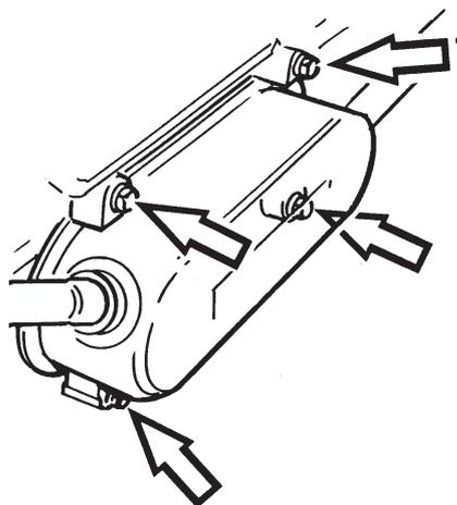
Remove the oil cooler fastening screws. If the engine has a fuel shut-off cock, undo the brackets which are fastened to the two upper screws and hang them up.
