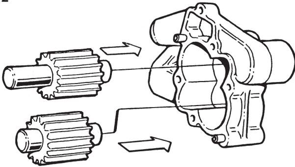
Oil the pump gears and bushes with engine oil, and put the pump gears into the housing.
