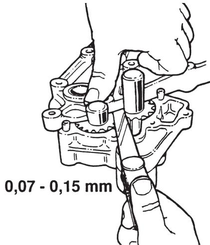
Check the end float on the pump gears, using a feeler gauge.
