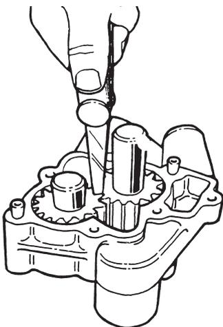
Check the pump gear flank clearance, using a feeler gauge.
