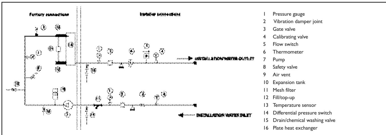
If the installation requires a useful head higher than that obtained by installing a pump assembly and storage tank, it is recommended that an additional pump is installed on the unit. The pump can be easily installed on the unit by removing the special pipe stub provided.
