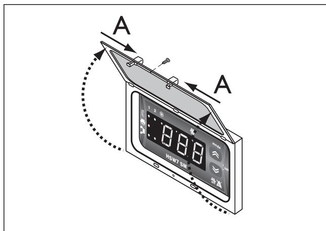
To access the control panel, open the door:
