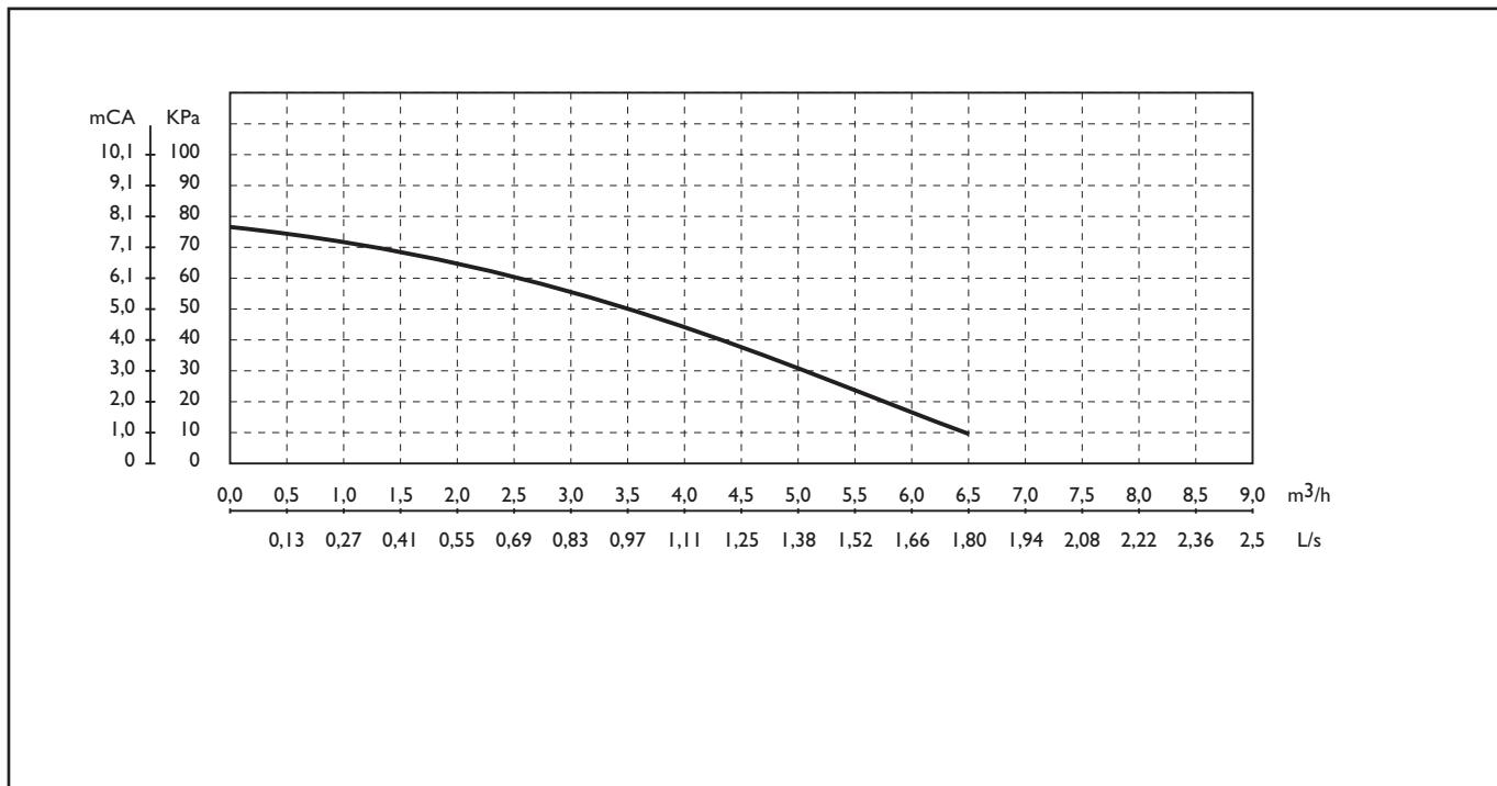
(\*) To obtain the useful head of the installation, subtract the pressure drop of the plate heat exchanger.
