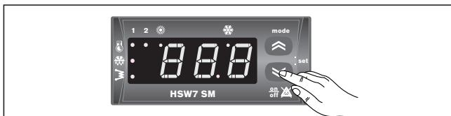
The temperature of water returning from the installation appears on the "values display".
