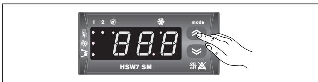
The cooling LED comes on. After a couple of seconds, the compressor 1 LED flashes until the compressor comes on
