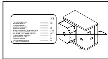
**⚠ Tampering with or the removal or absence of rating plates or other means enabling the unit to be identified causes problems during installation and maintenance.**
