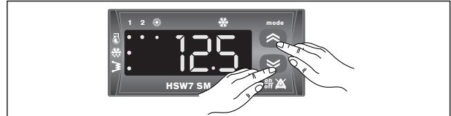
The water return temperature is displayed: the settings are complete. To display the status of the unit, the alarms and the operating hours, return to the SEt level, and then perform the procedure described above, selecting the desired index using the and buttons.
