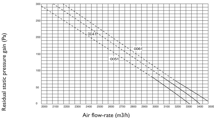
⚠ The characteristics indicated above refer to units with ducted outlets, with a 0.5m long straight duct and a cross-section equal to the cross-section of the fan.
