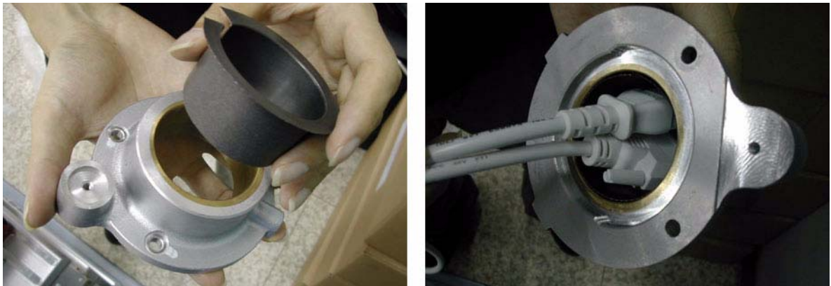
Figure 8-37 Inserting the oilless bush
