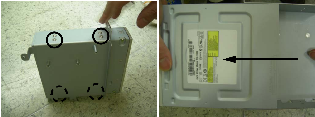
Figure 8-130 Unscrew 8screws and remove the DVD Drive from the bracket
