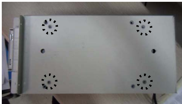
Figure 8-272 Color Printer Fixture Top Installation
