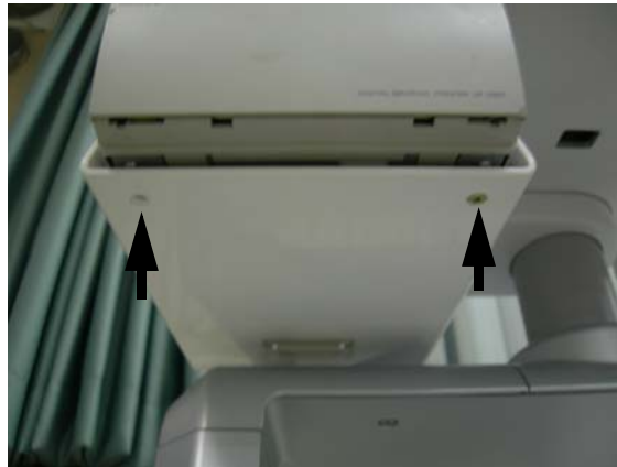
Figure 8-245 BW Printer Fixture Keyboard installation
