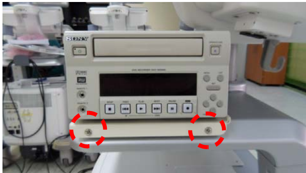
Figure 8-325 SONY DVR Fixture Top Installation
