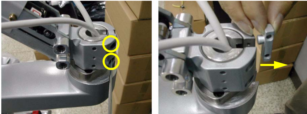
Figure 8-28 Removing the Arm stopper
