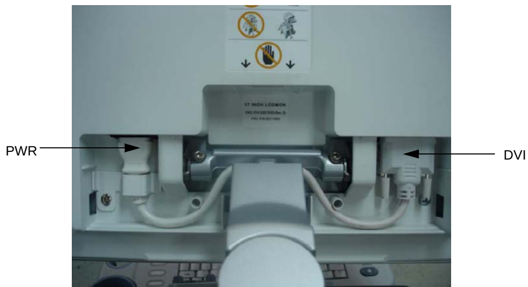
Figure 5-13 LP6 17" LCDMON Signal I/O
