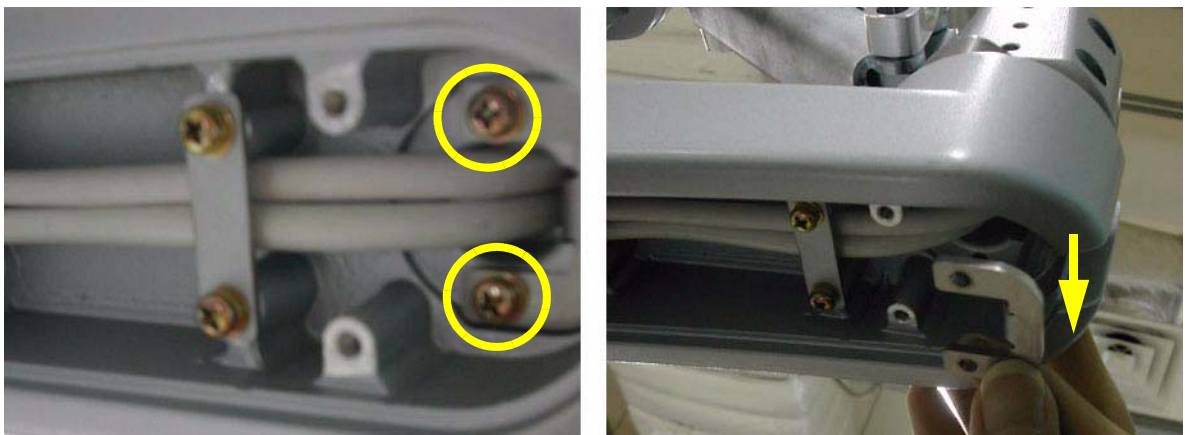
Figure 8-27 Removing the Lower arm guide bracket
