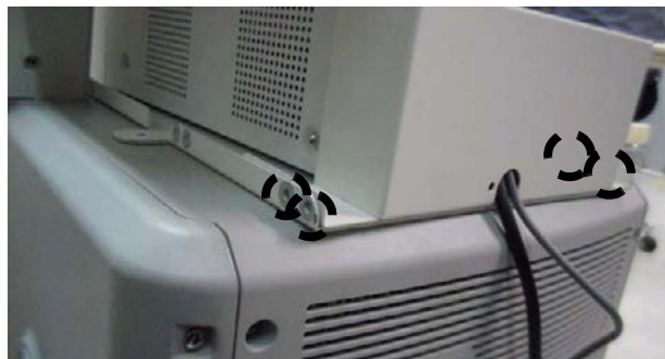
Figure 8-261 Color Printer Fixture Middle installation
