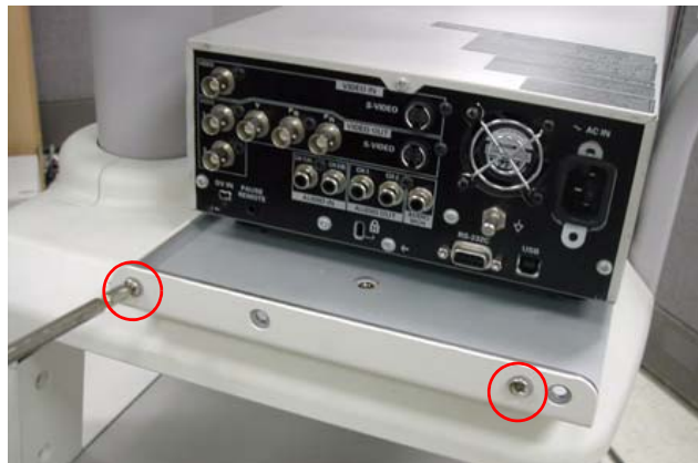
Figure 8-298 Printer VCR DVD Fixture Top installation (LQ MD800)
