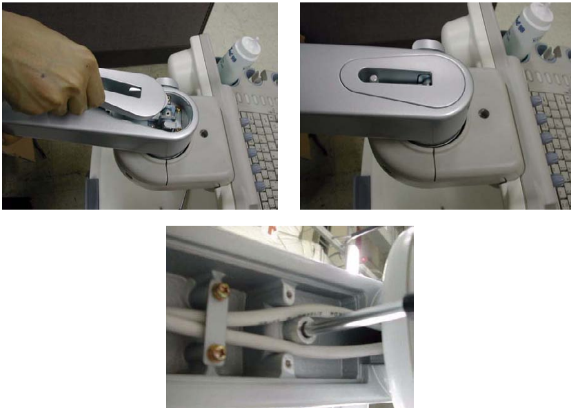
Figure 8-56 Assembling the Lock Cover
