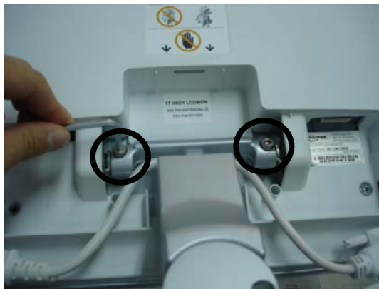
Figure 8-4 Separating the 17" LCD monitor
