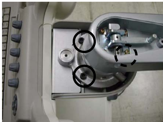
Figure 8-41 Assembling the arm neck pipe
