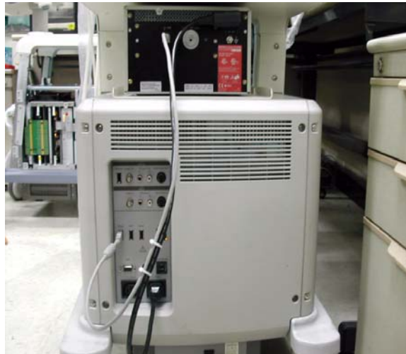
Figure 8-255 Color Printer Fixture Middle installation
