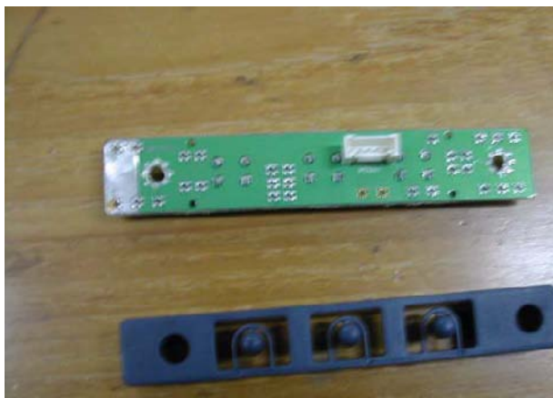
Figure 8-55 Assembling the Lock Knob
