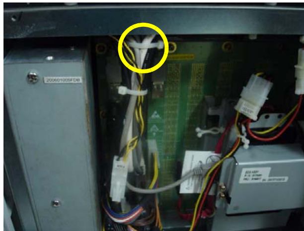
Figure 8-131 Connector and Screw2 screws on the Nest Fan
