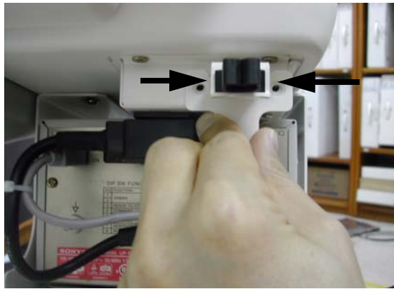
Figure 8-309 Additional Task Lamp Installation
