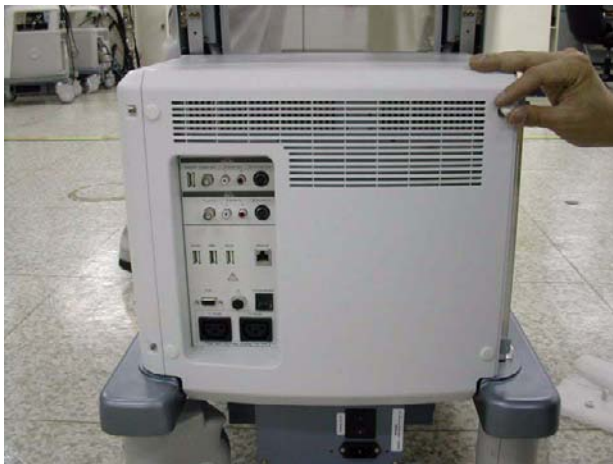
Figure 8-91 4 rubber caps and 4 screws on Rear Cover
