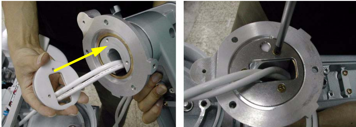
Figure 8-39 Fixing the flexible arm stopper
