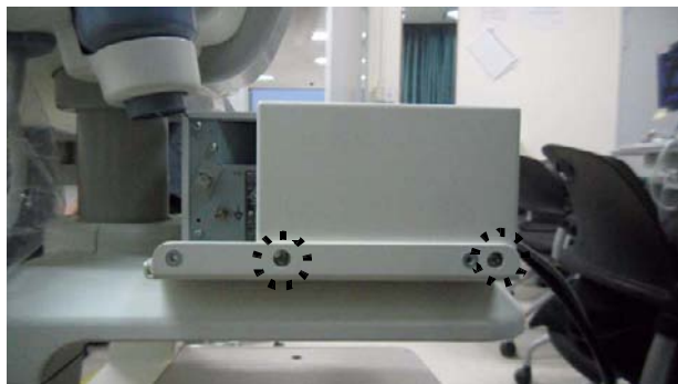
Figure 8-273 Color Printer Fixture Top Installation
