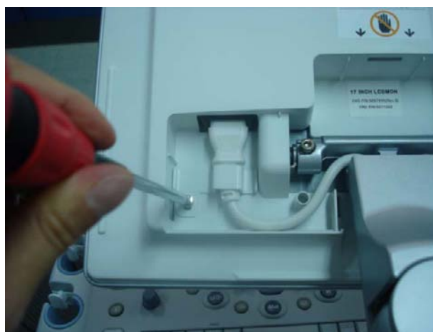
Figure 8-18 Removing the power cord bracket
