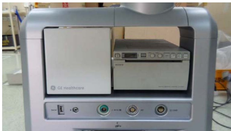
Figure 8-318 BT11 Drawer Option Installation
