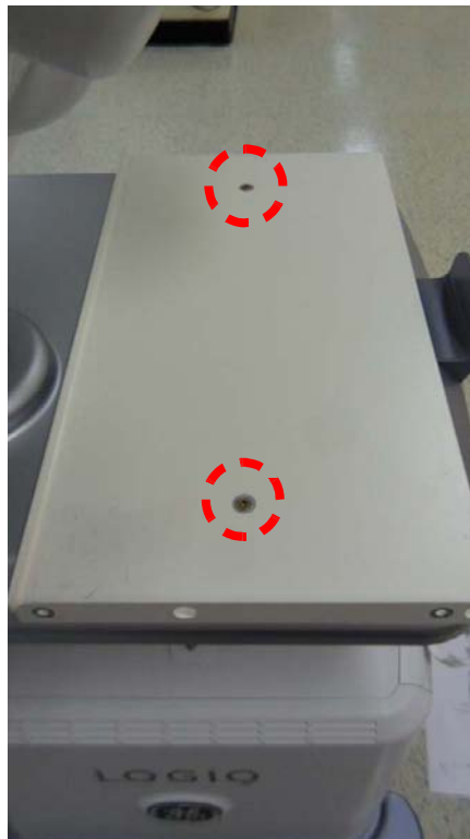
Figure 8-323 SONY DVR Fixture Top Installation
