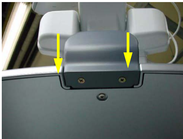
Figure 8-302 Rear Handle Installation
