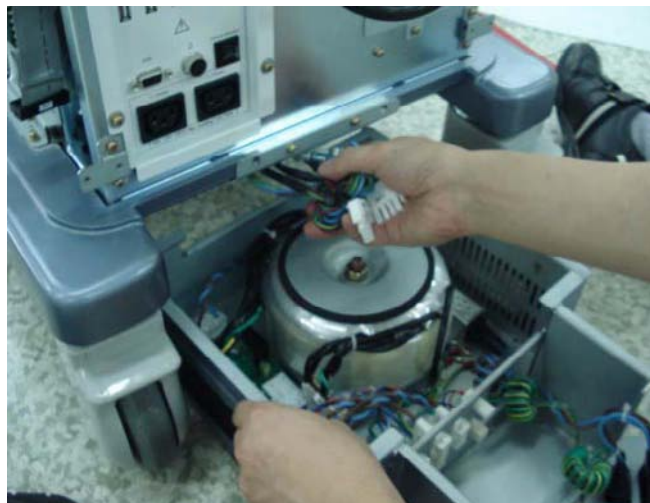
Figure 8-145 Insert the Transbox assy
