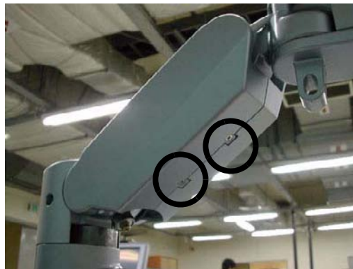
Figure 8-59 Assembling the Arm Cover L & R
