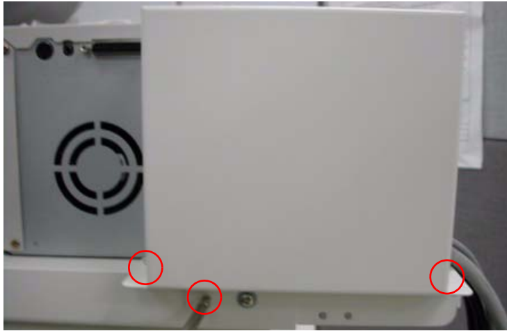
Figure 8-281 Printer VCR DVD Fixture Top installation
