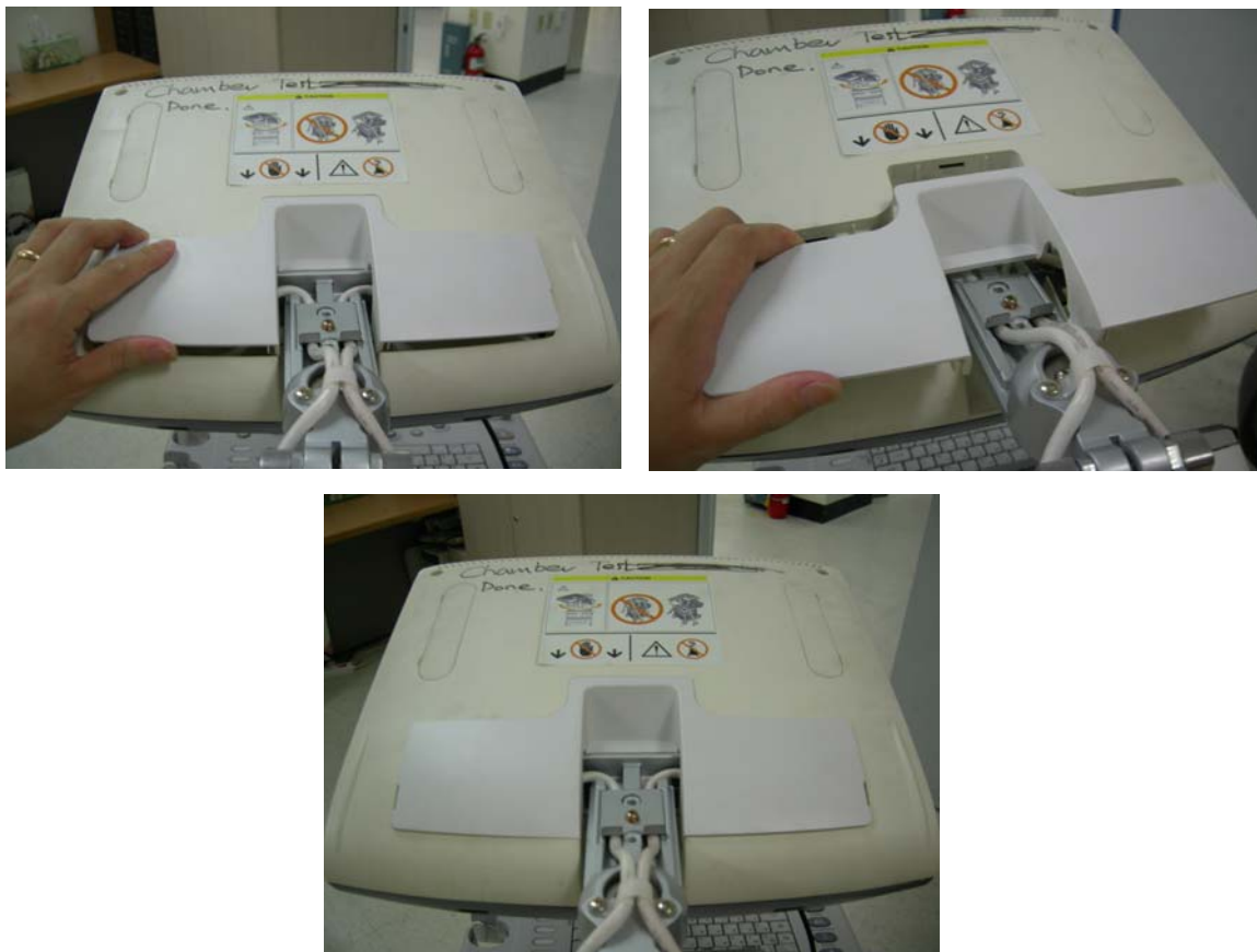
Figure 8-53 Assembling the LCD cable cover
