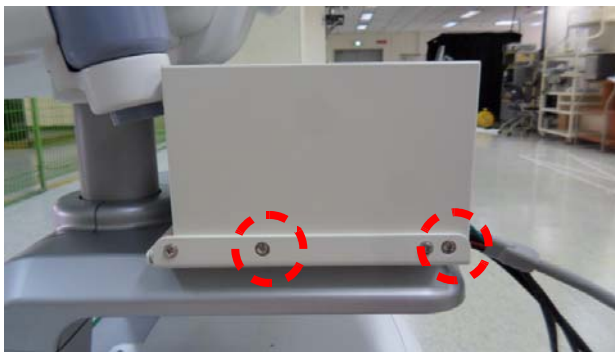
Figure 8-327 SONY DVR Fixture Top Installation
