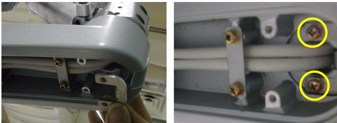
Figure 8-46 Assembling the Lower arm guide bracket
