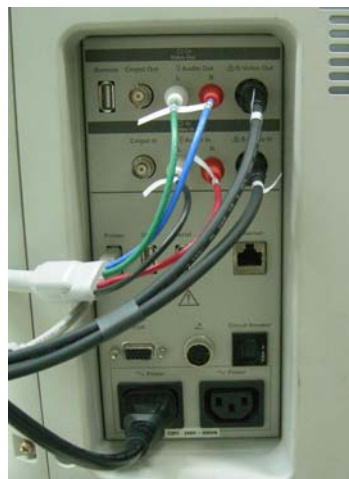
Figure 8-300 Printer VCR DVD Fixture Top installation (LQ MD800)
