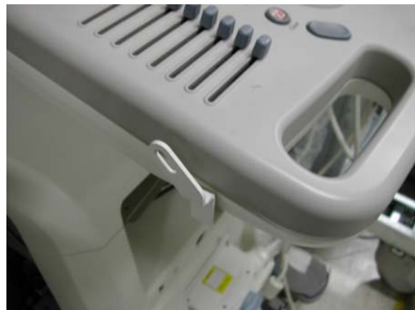
Figure 8-233 installation of Microphone
