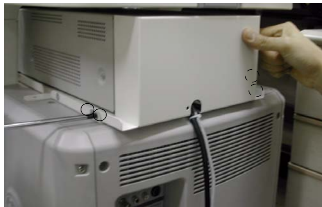
Figure 8-256 Color Printer Fixture Middle installation
