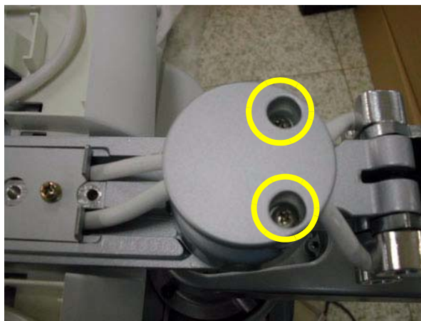
Figure 8-65 Removing the Arm cable cover
