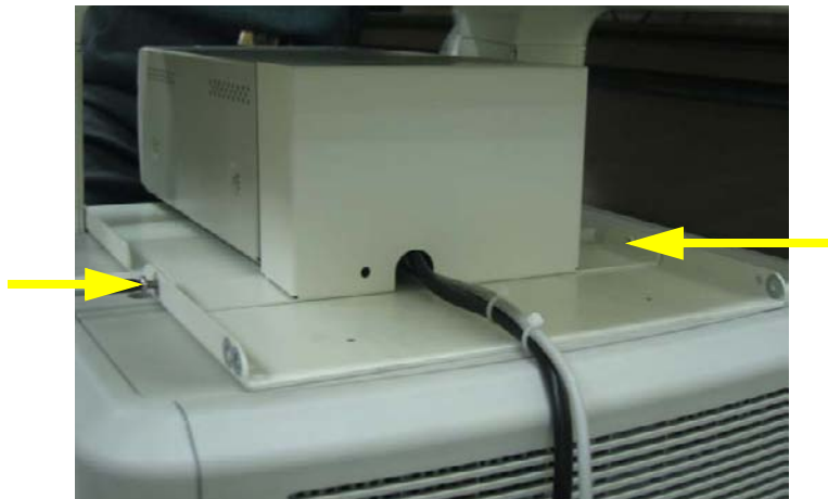
Figure 8-251 BW Printer Fixture Middle installation
