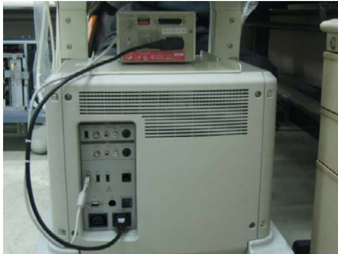
Figure 8-250 BW Printer Fixture Middle installation
