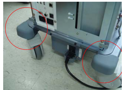
Figure 8-312 Protect Cover Installation
