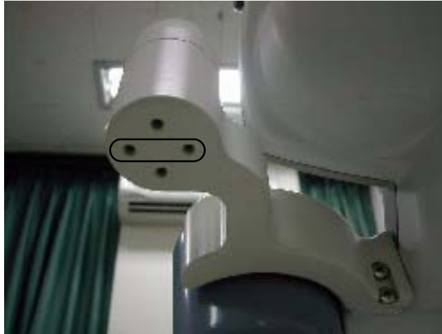
Figure 8-230 Endo Probe Holder Installation
