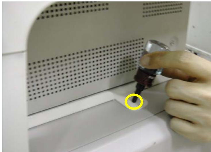
Figure 8-254 Color Printer Fixture Middle installation
