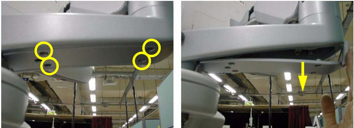
Figure 8-25 Removing the Arm bottom cover
