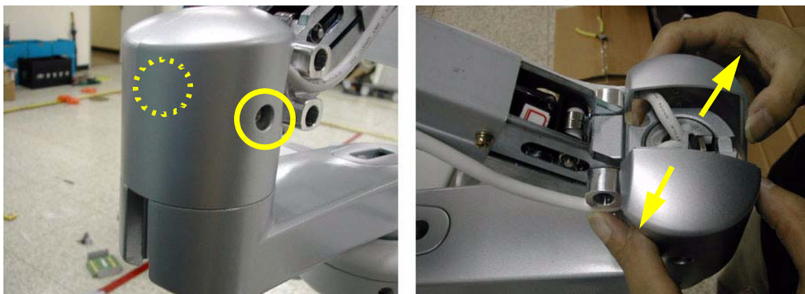
Figure 8-24 Removing the Cam cover L & Cam cover R
