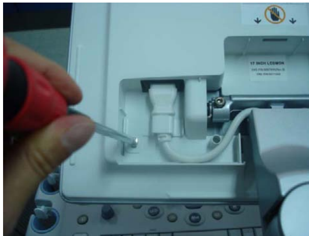
Figure 8-2 Removing the power cord bracket
