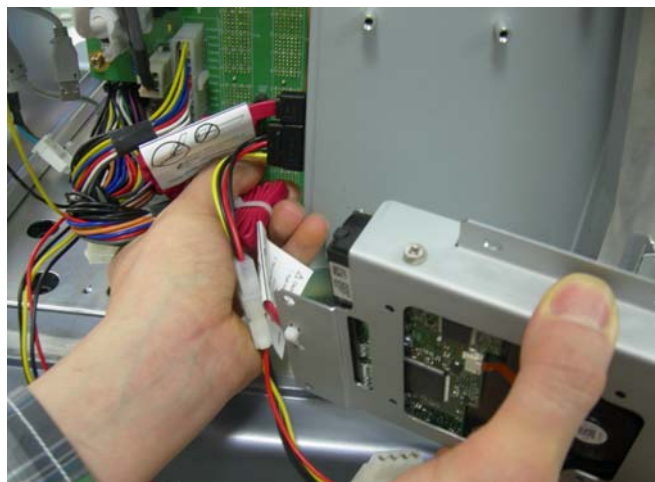
Figure 8-137 Disconnect the SATA Cable
