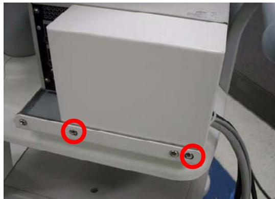
Figure 8-267 Printer VCR DVD Fixture installation top
