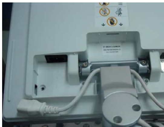
Figure 8-38 Inserting the flexible arm
