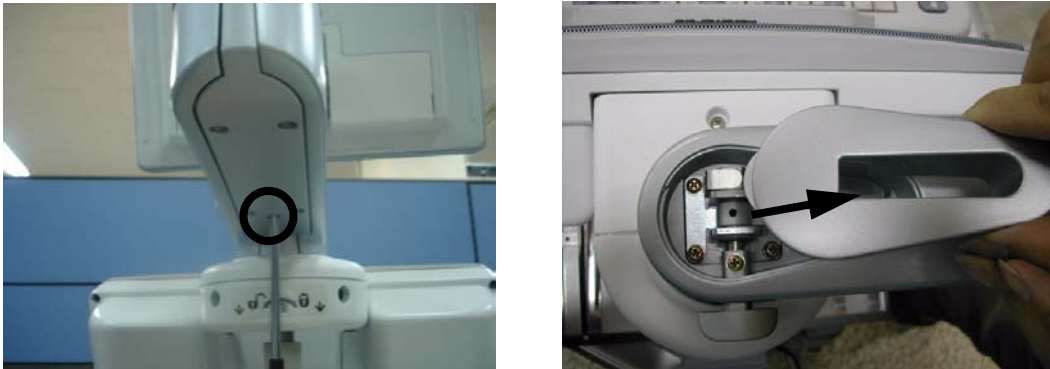
Figure 8-66 Removing the Arm lock cover
