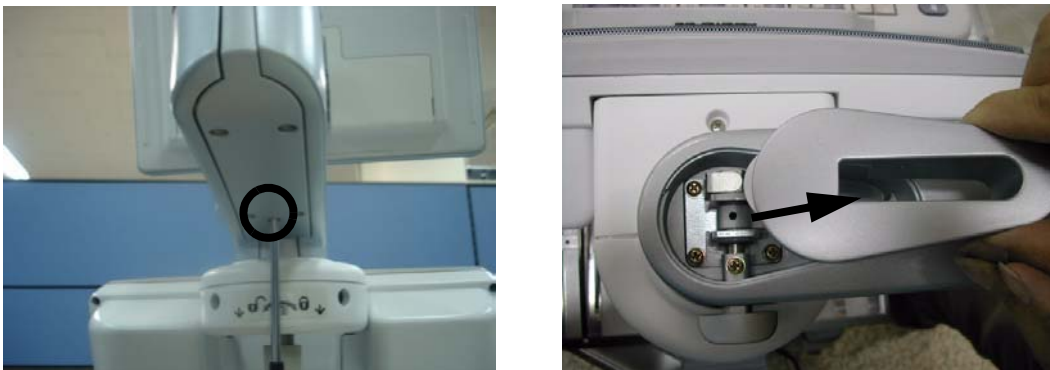
Figure 8-67 Removing the Arm lock cover
