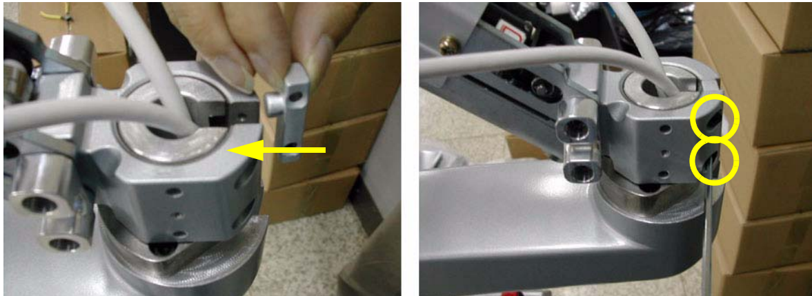
Figure 8-45 Installing the Arm stopper
