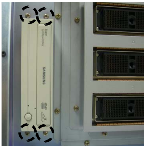
Figure 8-129 Unscrew 4screws and remove the DVD Assy
