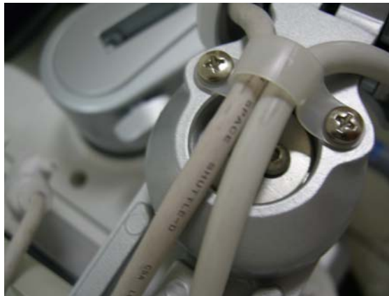
Figure 8-50 Assembling the Cable clamp
