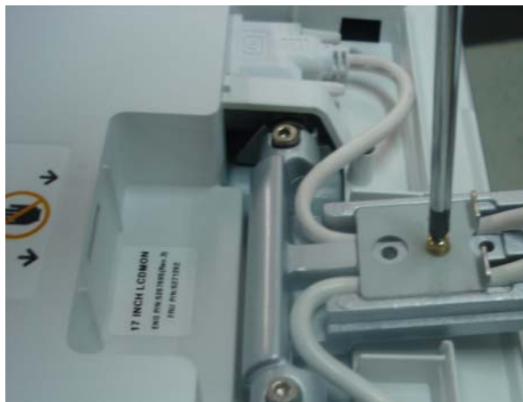
Figure 8-49 Assembling the Cable bracket
