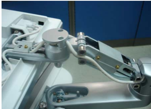
Figure 8-48 Placing the Cables
