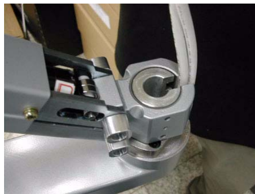
Figure 8-44 Putting in the cables
