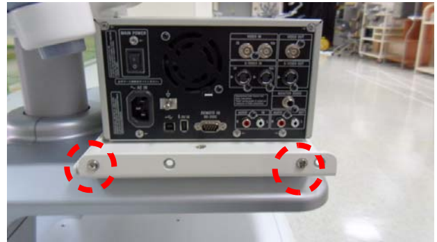
Figure 8-325 SONY DVR Fixture Top Installation
