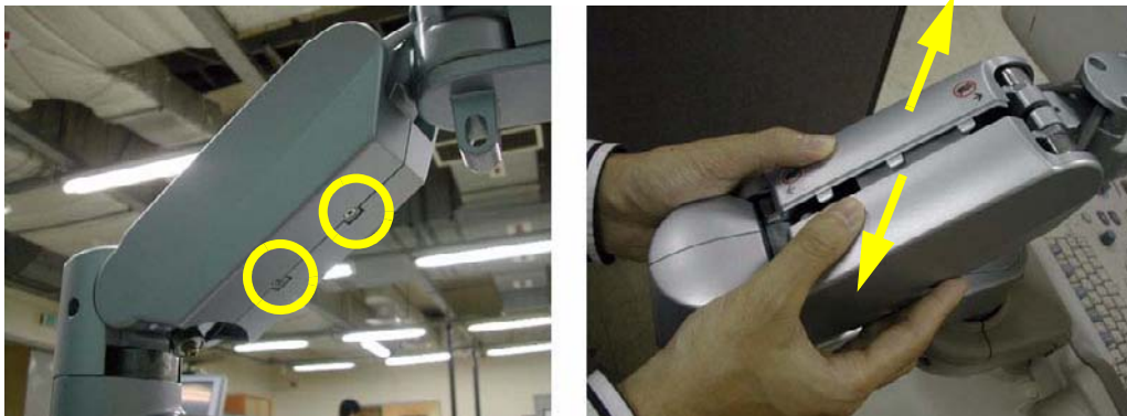
Figure 8-62 Removing the Arm cover L & Arm cover R
