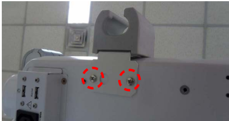
Figure 8-320 MTZ PROBE HOLDER Installation
