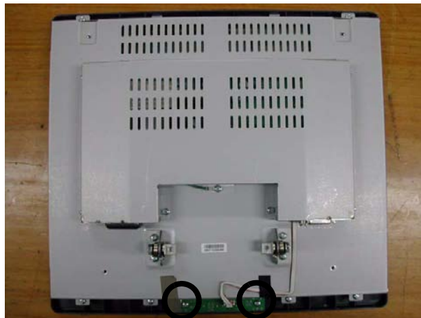
Figure 8-12 Removing the OSD Key Assy
