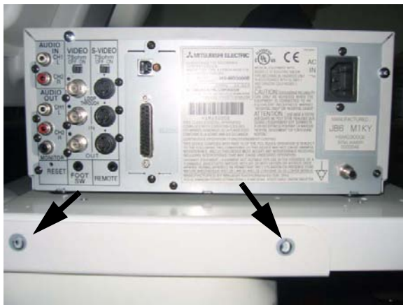
Figure 8-289 Printer VCR DVD Fixture Top installation
