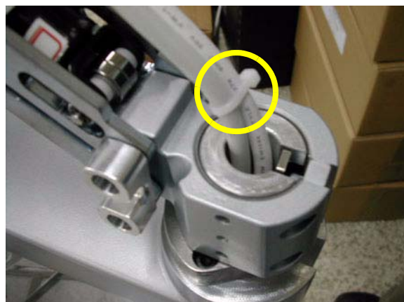
Figure 8-47 Tying the cables
