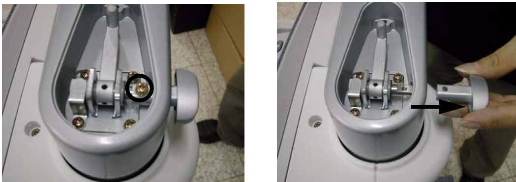
Figure 8-68 Removing the Arm lock Knob
