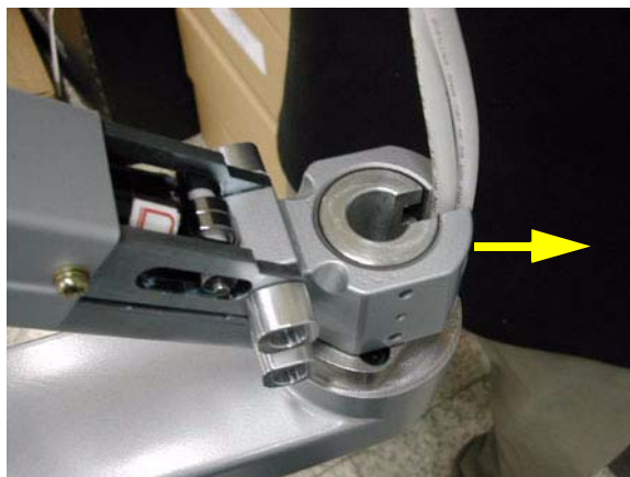
Figure 8-29 Pulling out power cable & DVI cable
