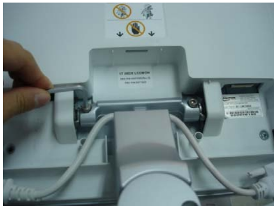
Figure 8-15 Removing the power code bracket
