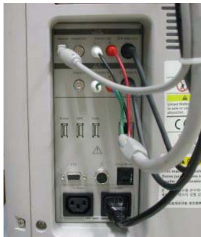
Figure 8-293 Printer VCR DVD Fixture Top installation
