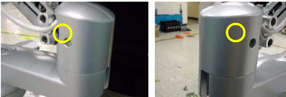
Figure 8-57 Assembling the Cam Cover L & R
