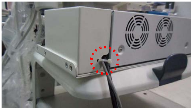
Figure 8-274 Color Printer Fixture Top Installation
