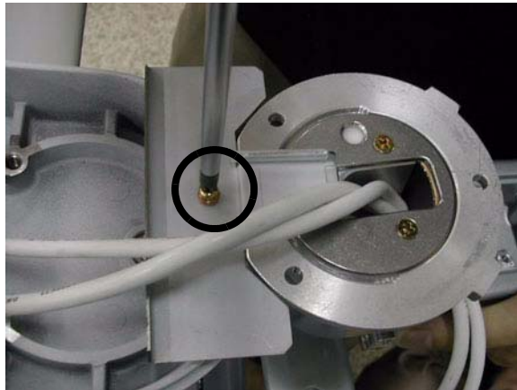
Figure 8-33 Removing OP bracket
