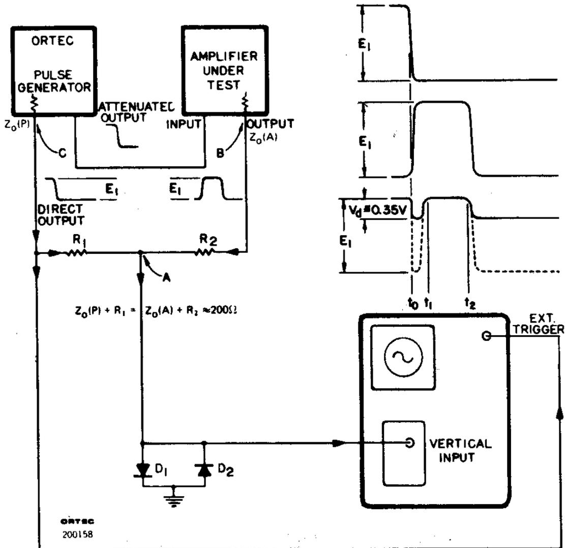
Fig. 4.5. Measuring Linearity by the Null-Balance Method.
