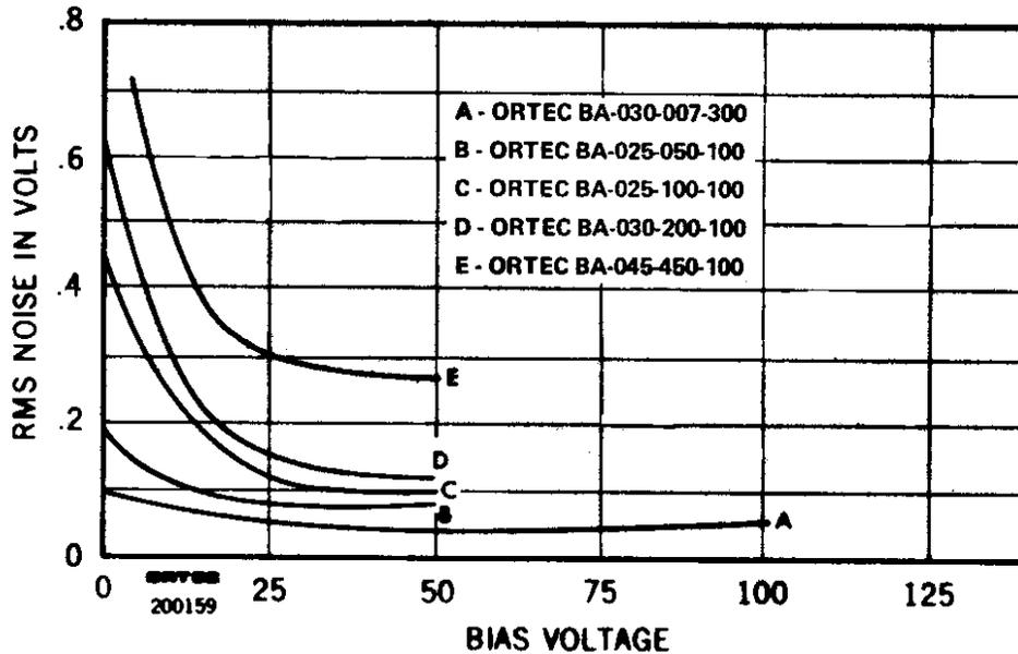
Fig. 4.4. Amplifier and Detector Noise vs. Bias Voltage.
