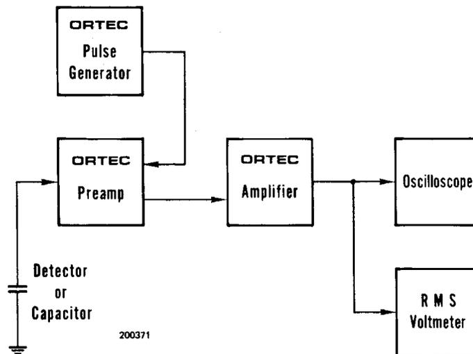
Fig. 4.1. Measuring Amplifier and Detector Noise Resolution.
