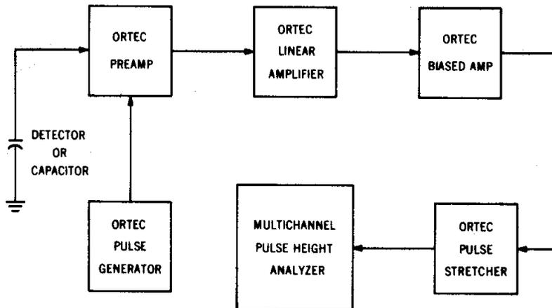
Fig. 4.3. Measuring Resolution with a Pulse Height Analyzer.
