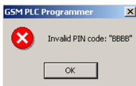
Note! PLC PIN code doesn’t change the SMI card’s PIN code. It can be used for extra security, but in most cases it is not needed.
