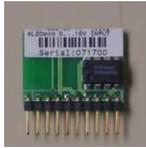
Analog input can be converted to digital input using analog to digital conversion module. E.g. if its used in AL20AN which has 8 analog inputs, these inputs can be converted to additional 8 digital inputs. Conversion module works all AutoLog which have AI module places (AL4 - AL20) and all GSM-PLCs (GSM8, GSM-16, GSM20). These cannot be used in AL10SP.
