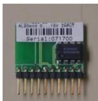
AutoLog GSM-PLCs needs to be equipped with analog input modules before analog inputs can be used. Analog input modules can be used in GSM-PLCs (GSM-8, GSM-16 and GSM-20).
