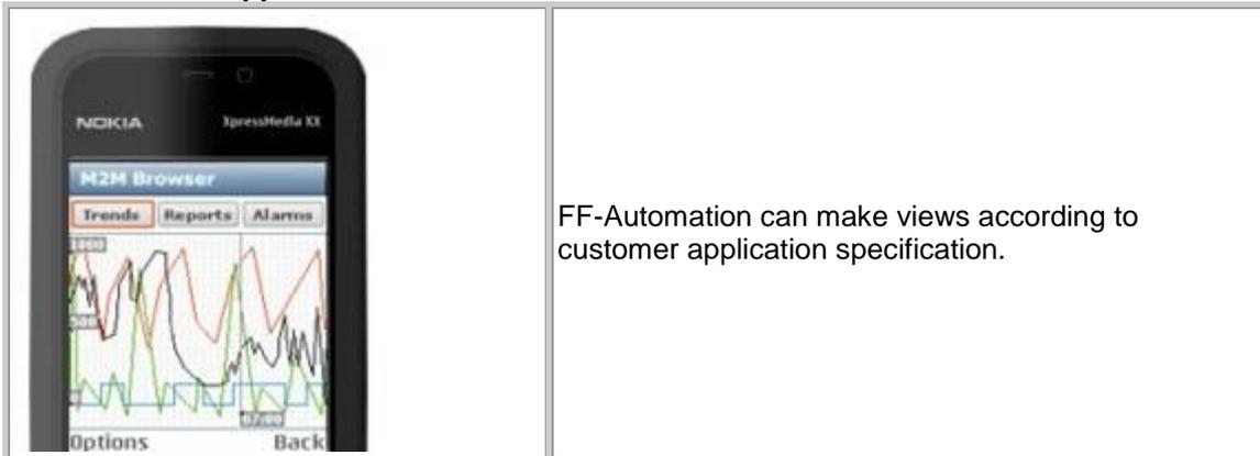
Normally graphical user interface views are browsed with desktop PC's Internet browser, but ControlMan pages can be designed to be used also with small resolution mobile phones. Mobile phone's Internet browser should have Flash support. Older GSM phones can be used to receive SMS text messages like alarms, work orders (Trouble ticket system), measurement reports and also to send control commands, set point changes, acknowledgements etc.
