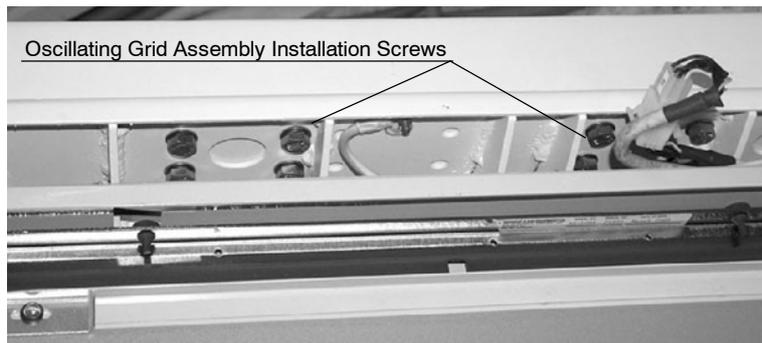
17. Connect J1 (only for Oscillating Grid Assembly with motorized Grid), J2 and GND from the Harness to the Oscillating Grid Assembly.
