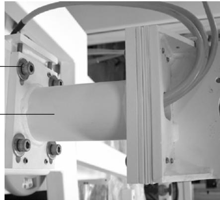
2. Assemble the Control Panel in the Support with the two screws, washers and nuts attached to the Control Panel.
