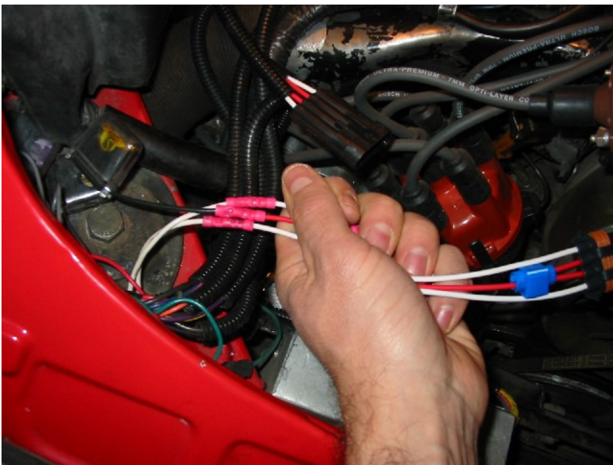
Figure 60: Fuel injector connector to 20Amp fuse
