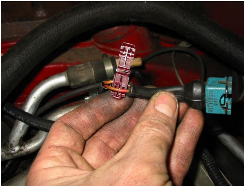
Figure 65: Fuel pump disable T-Tap
