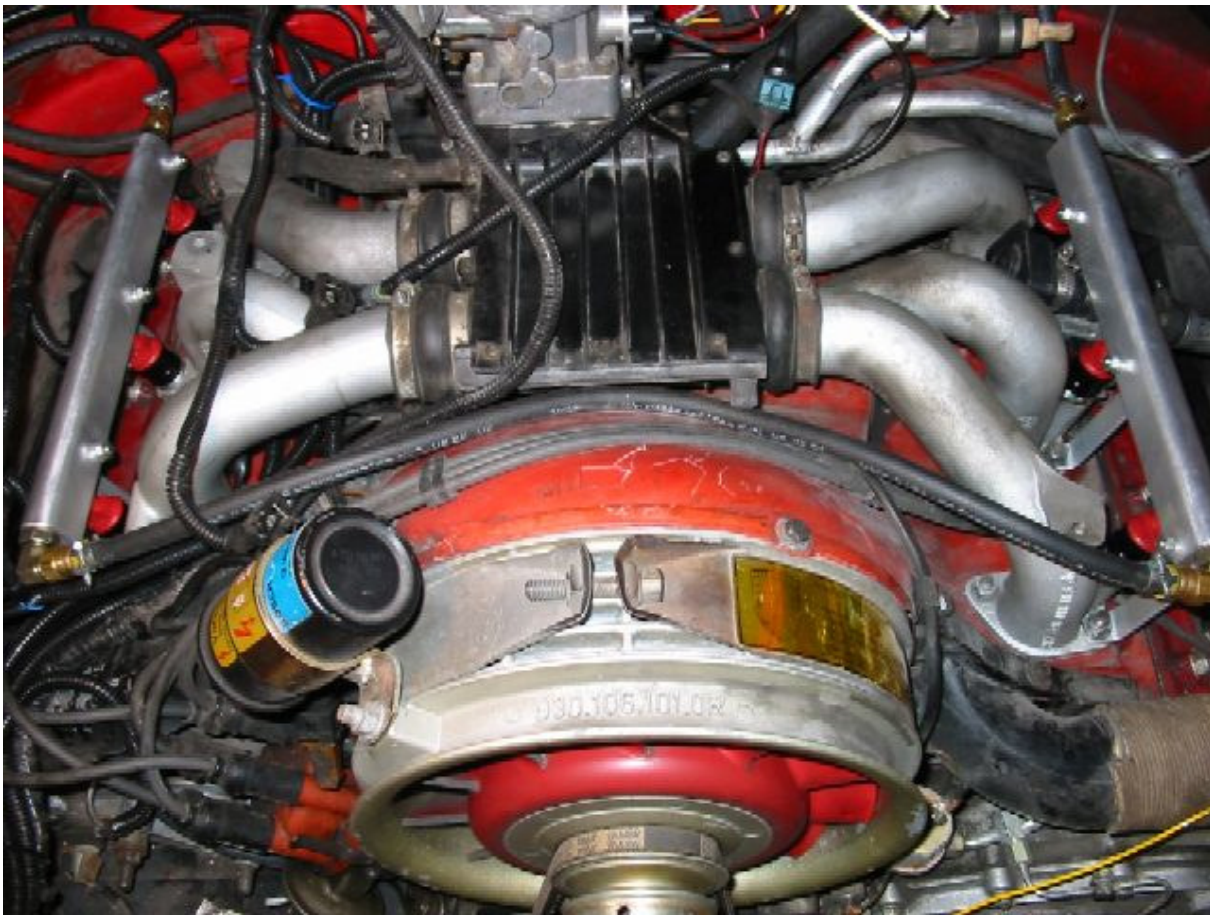
Figure 34: Fuel hose left to right rail
