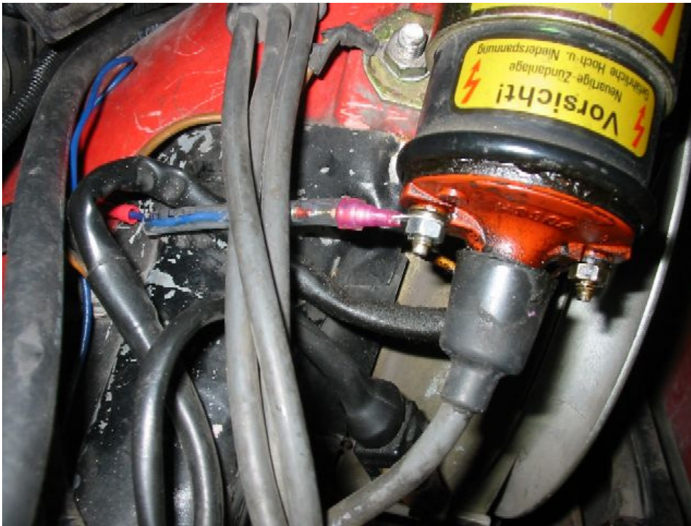
Figure 83: TACH pickup for BOSCH CDI ignition
