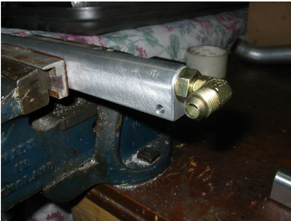
Figure 22: Fuel rail fitting (90 degree)
