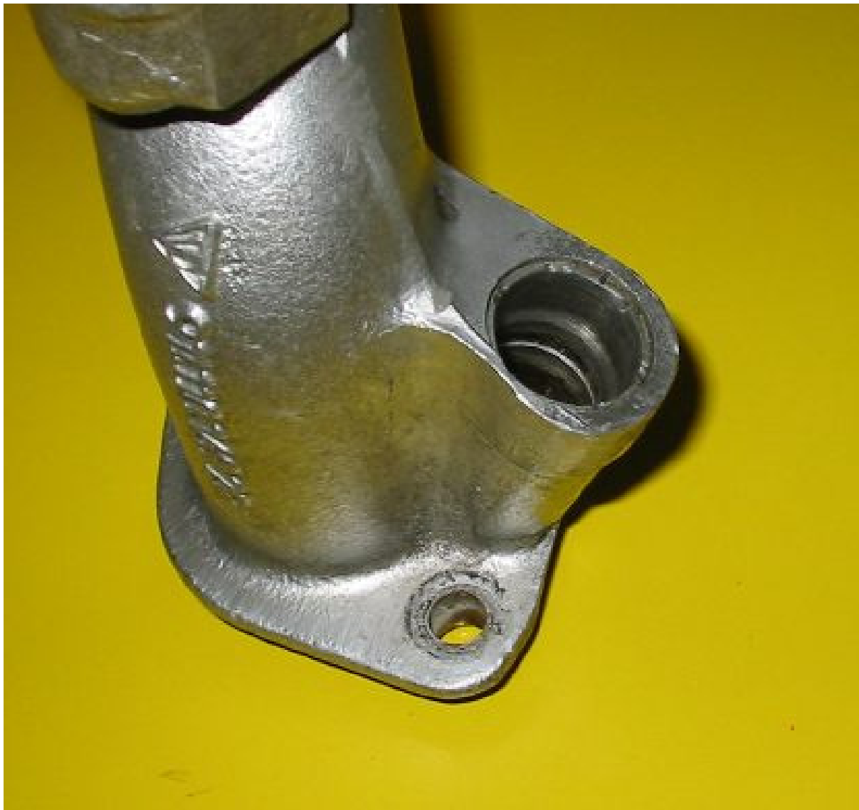
Figure 19: CIS injector bung removed
