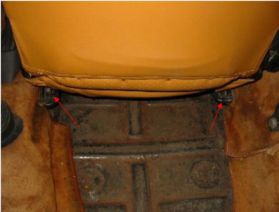
Figure 39: Passenger seat rear bolts
