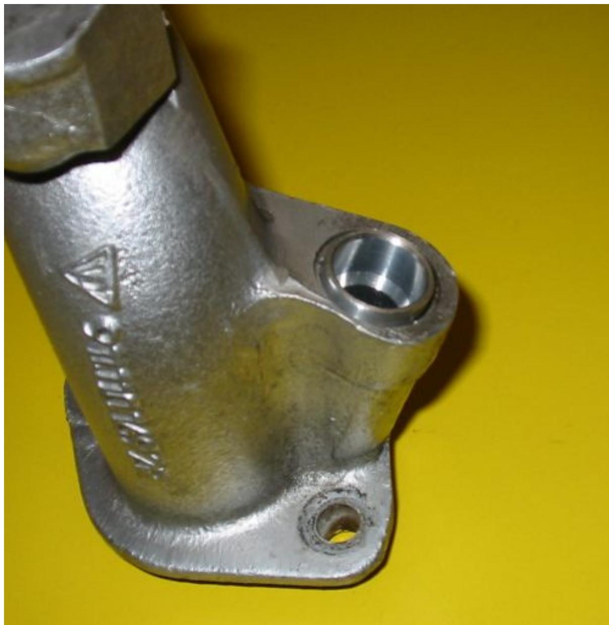
Figure 20: Intake runner with EFI injector bung
