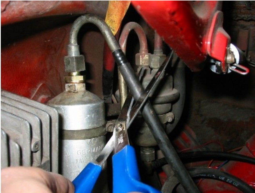
Figure 5: fuel feed line
