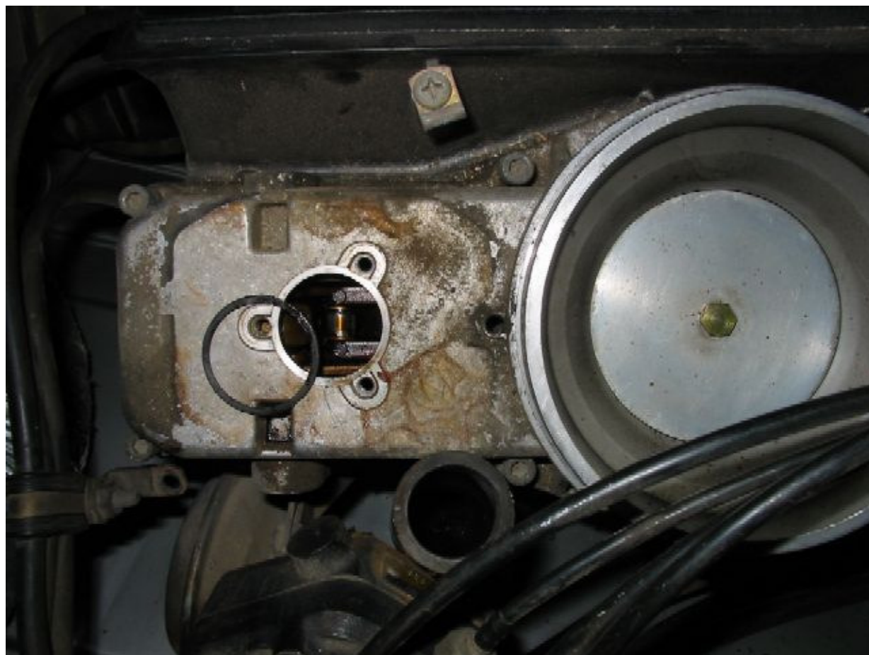
Figure 15: Fuel distributor removed
