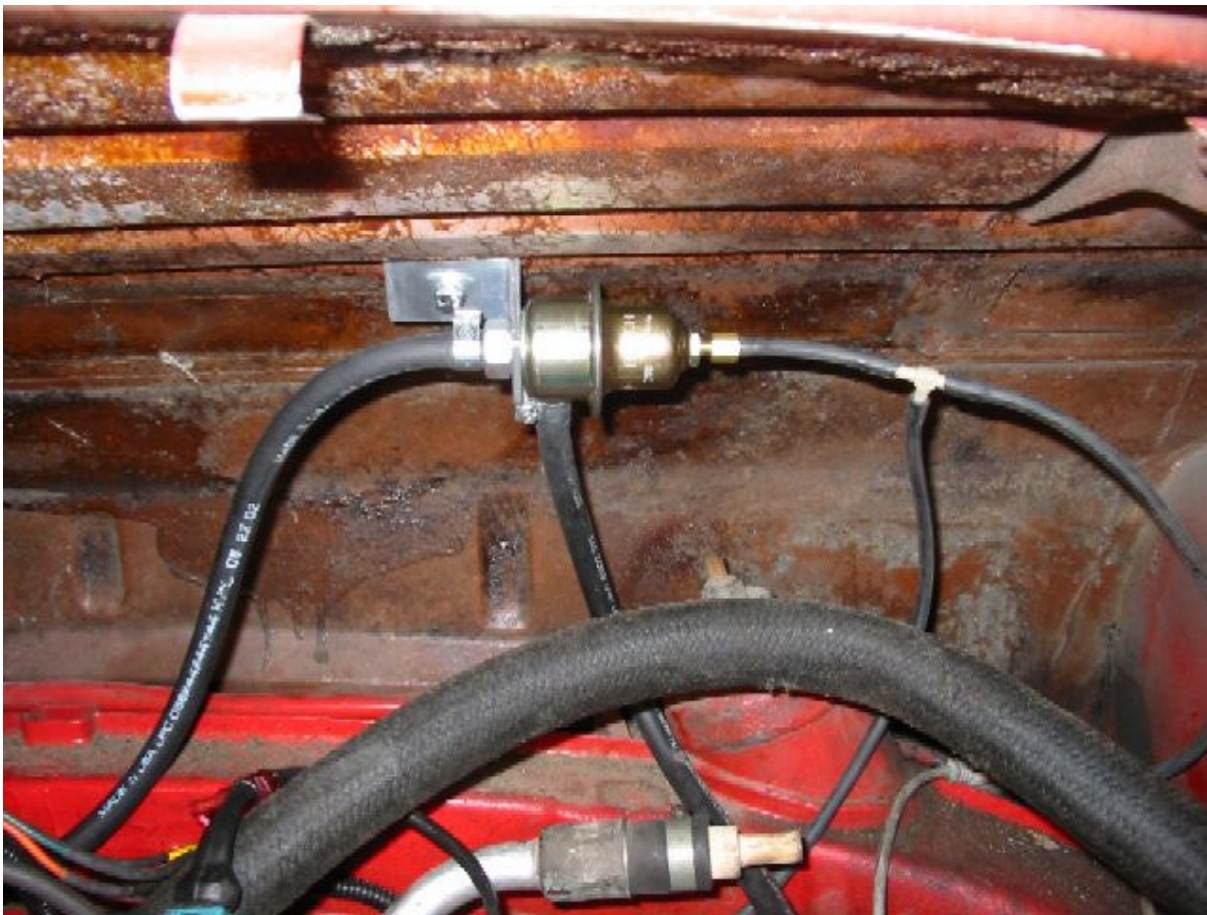
Figure 38: Completed fuel pressure regulator install
