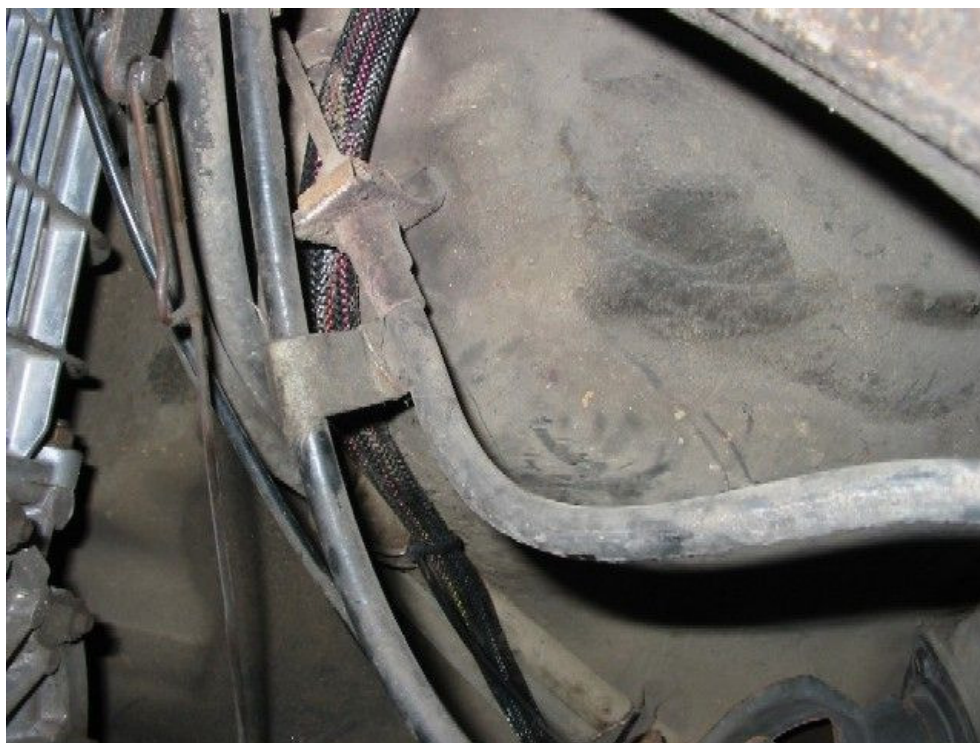
Figure 48: harness following fuel lines
