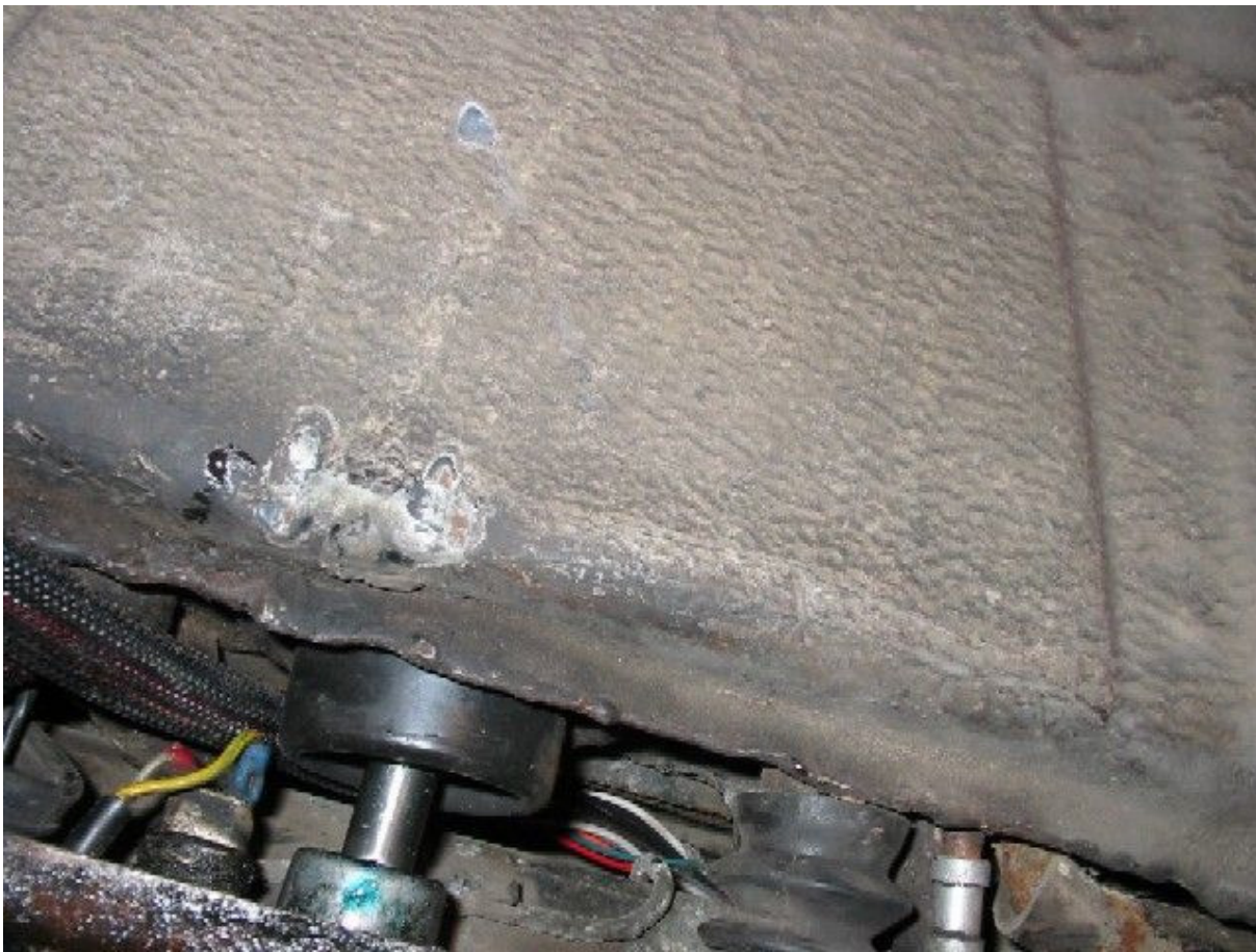
Figure 47: Harness exit hole
