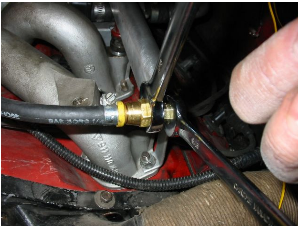
Figure 33: tightening fuel rail fittings
