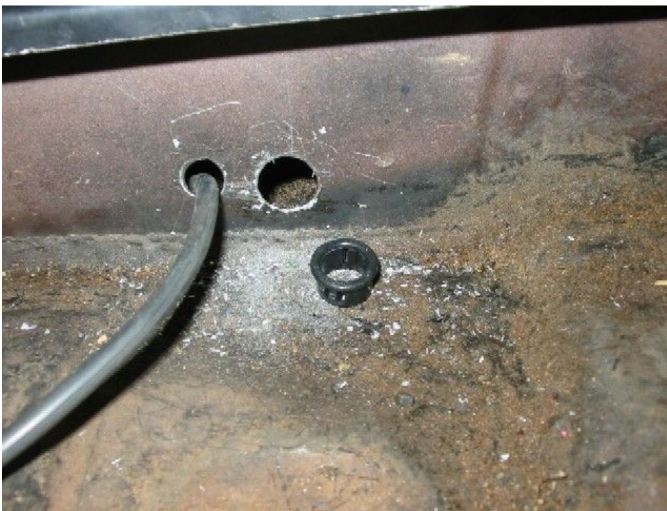
Figure 40: Routing holes in tunnel
