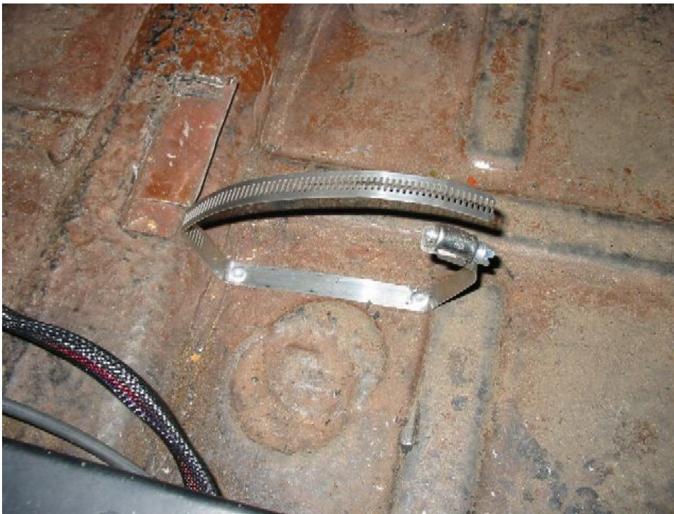
Figure 92: Mounting the ECU
