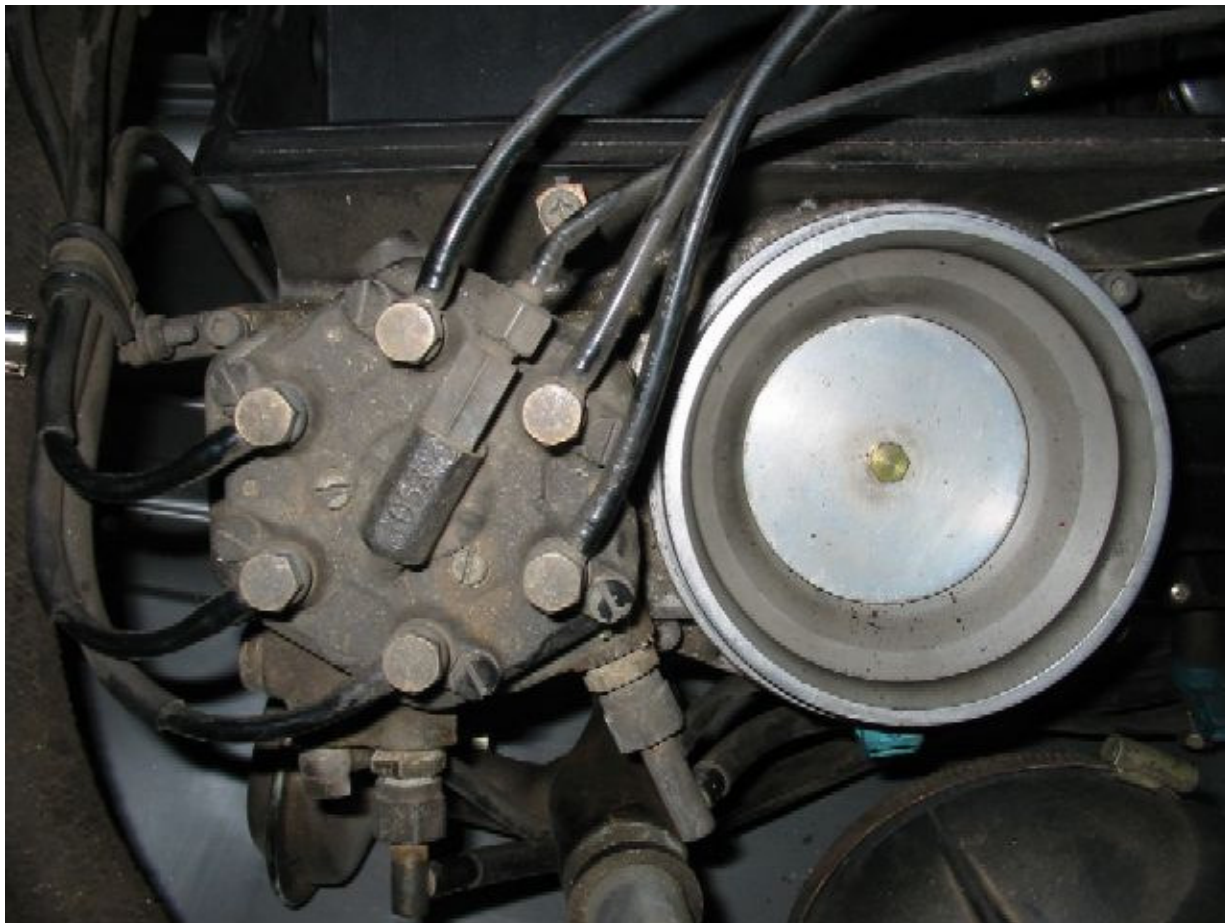
Figure 13: Fuel distributor and mixture control unit
