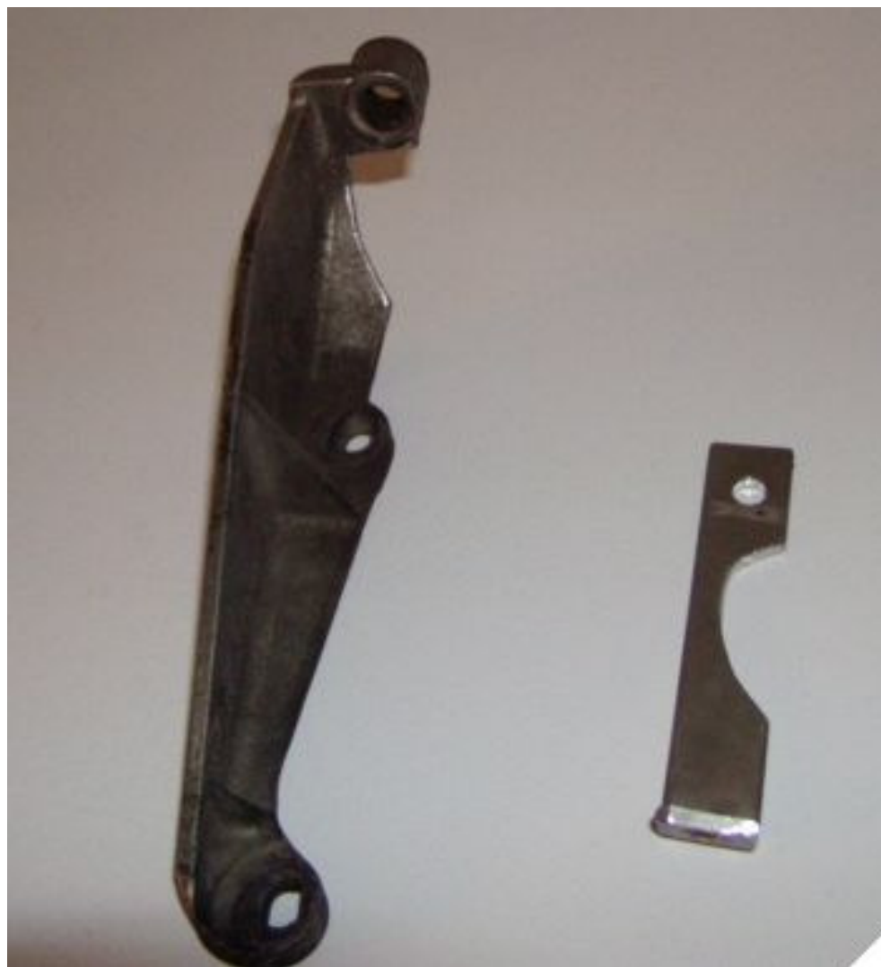
Figure 31: A/C compressor bracket modification
