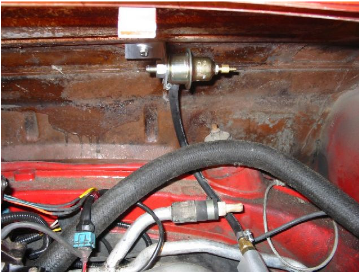
Figure 37: Fuel pressure regulator mounted
