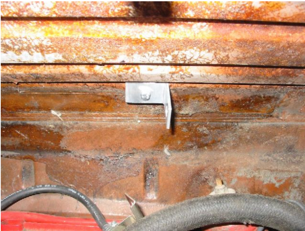
Figure 36: Fuel pressure regulator mounting bracket
