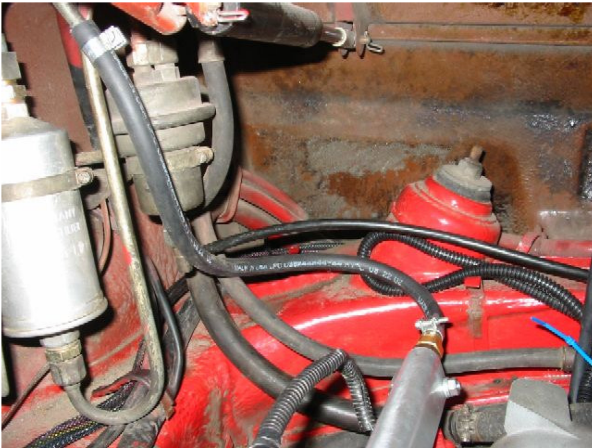
Figure 32: Fuel hose from filter to left rail
