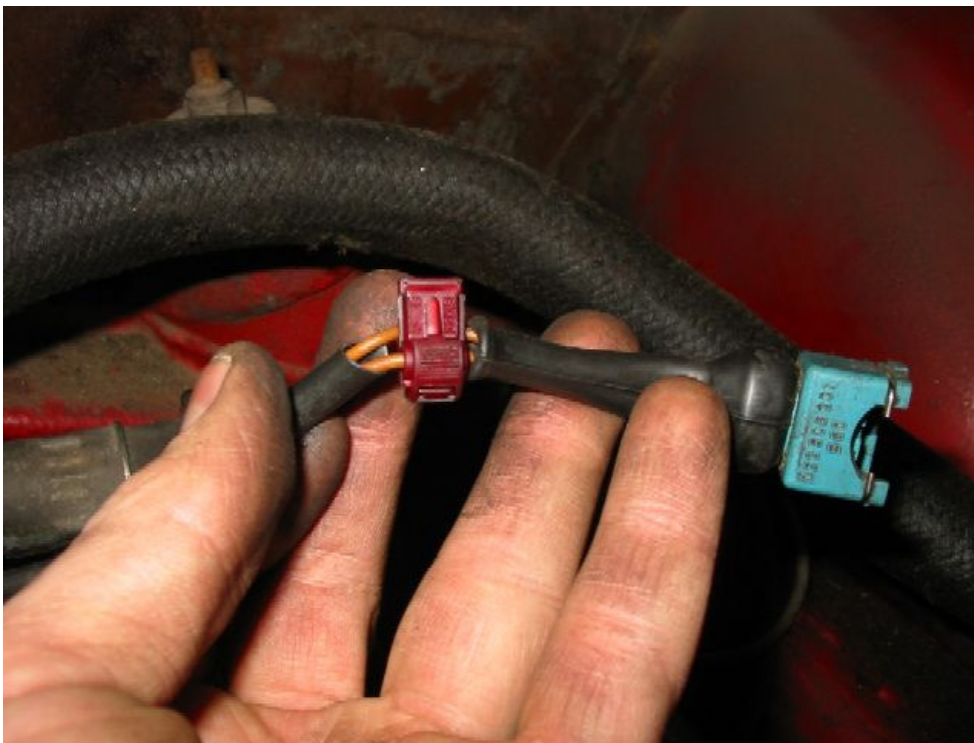
Figure 66: Tapped connection made to existing wiring (fuel pump disable)
