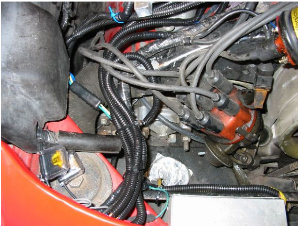
Figure 84: Adding the corrugated wire loom
