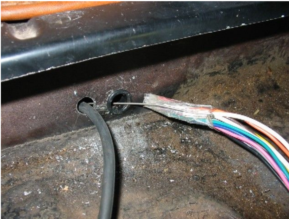
Figure 42: Pulling the harness
