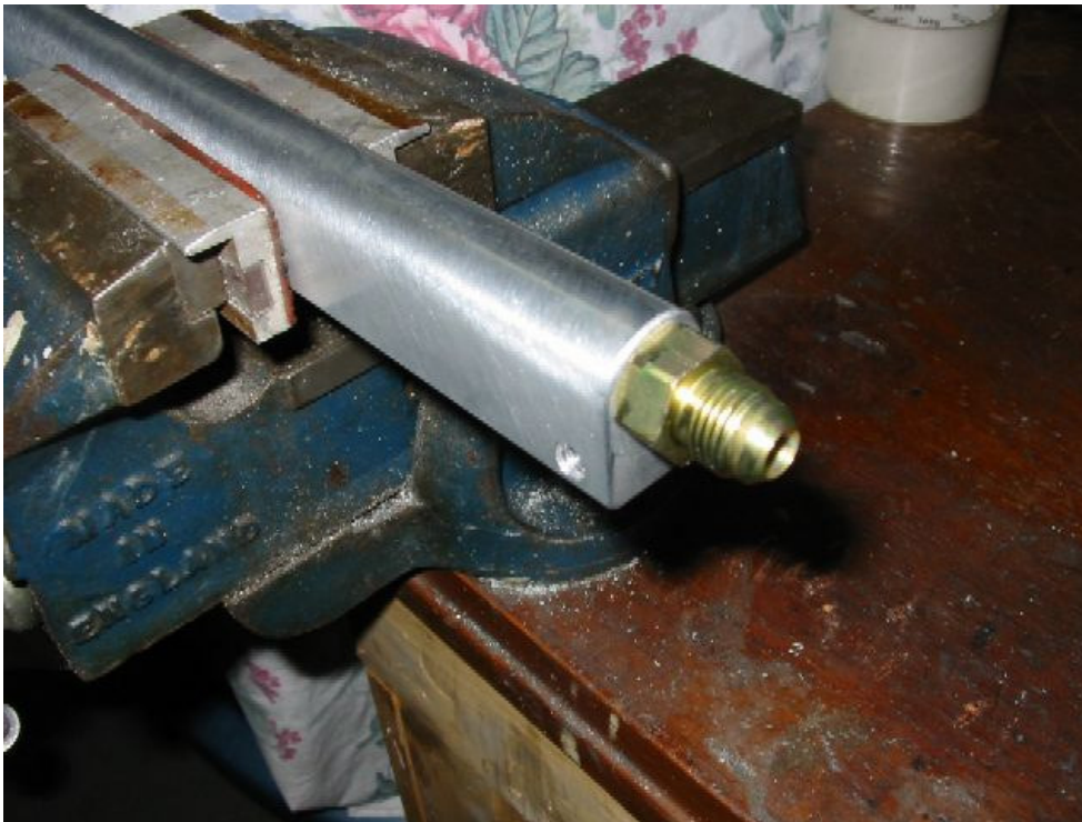
Figure 21: Fuel rail fitting (straight)
