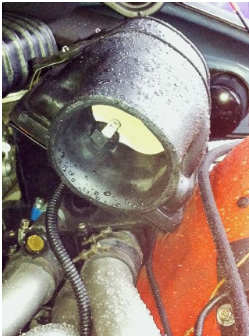
Figure 89 : Better MAT sensor location
