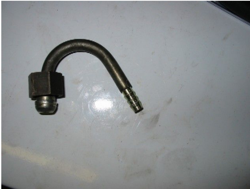
Figure 7: feed line fitting ready for installation
