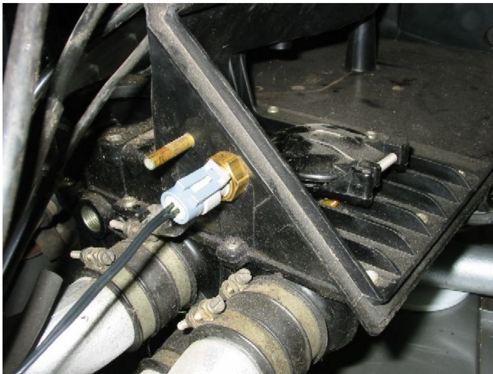
Figure 87: MAT location on airbox
