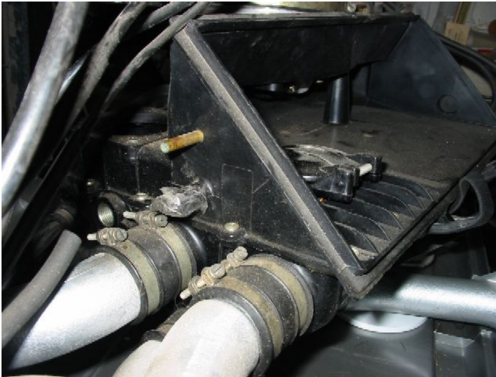
Figure 85: MAT location on airbox
