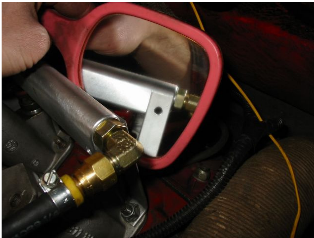
Figure 25: Fuel rail hole alignment
