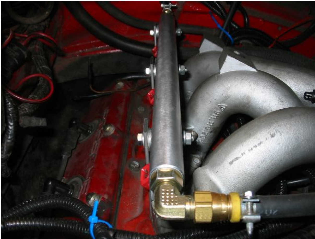
Figure 26: Left fuel rail completed
