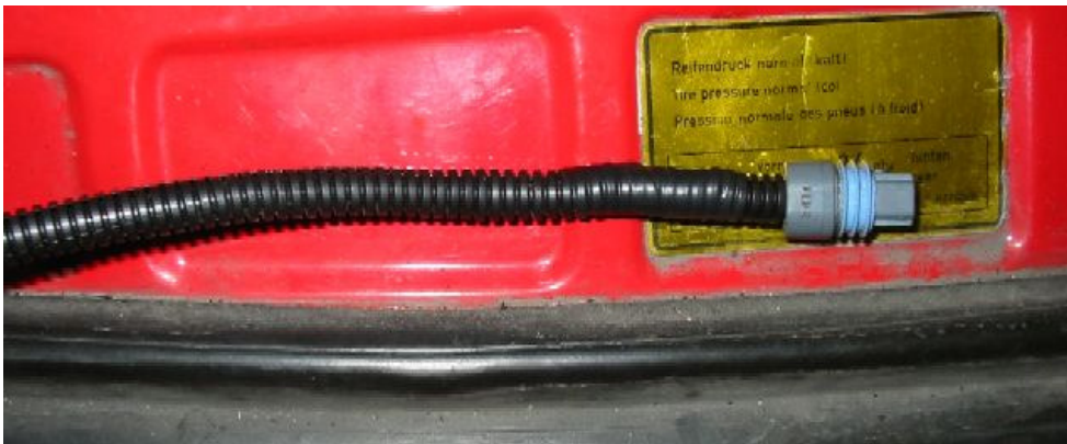
Figure 62: Air temperature sensor connector complete
