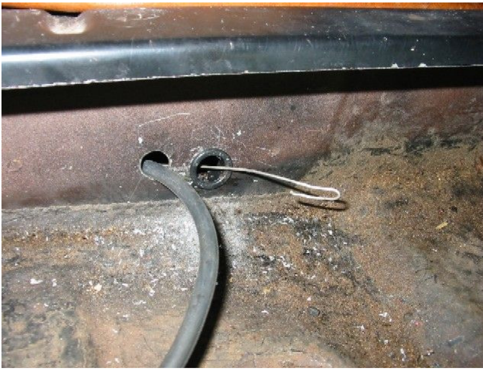
Figure 41: fishing the main harness
