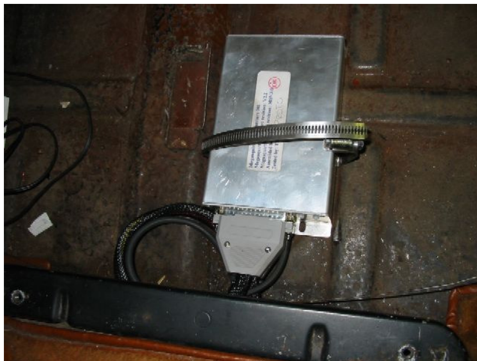
Figure 93: Mounting the ECU
