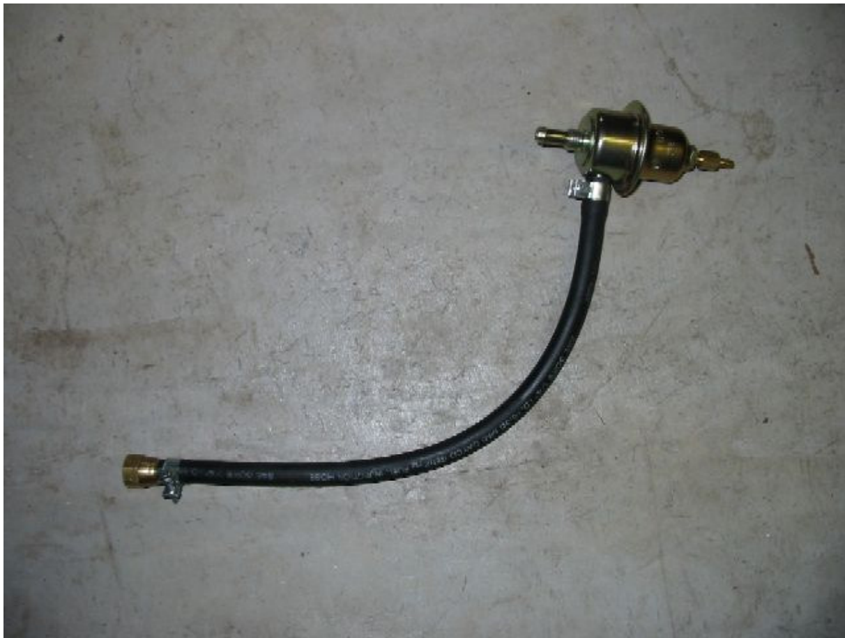
Figure 35: Fuel Hose attached to fuel pressure regulator
