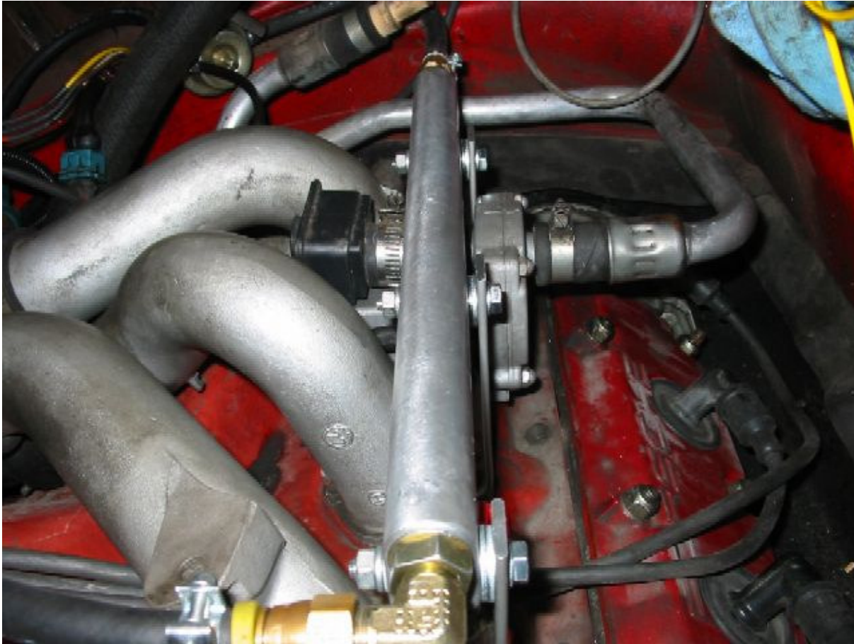
Figure 29: Right side fuel rail complete
