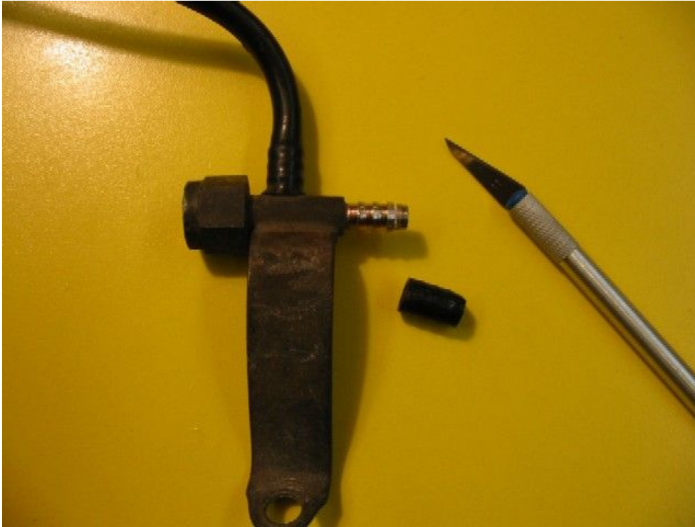
Figure 9: Return line Tee ready for install
