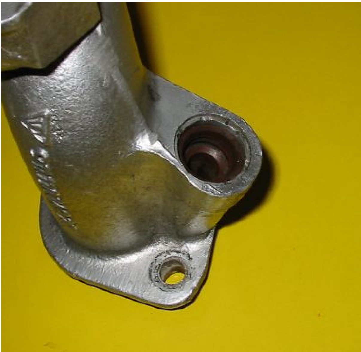
Figure 18: Intake runner with CIS injector bung
