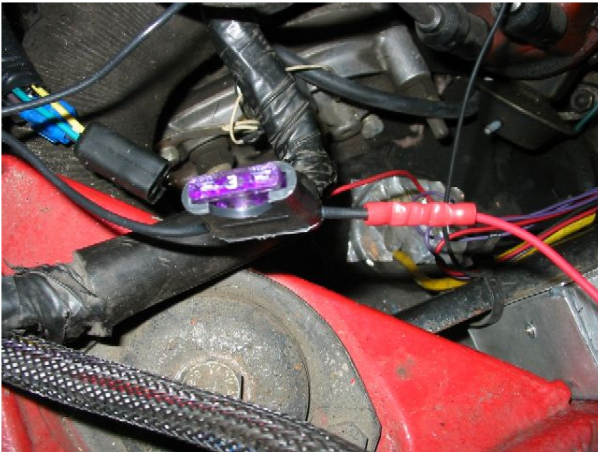
Figure 58: MegaSquirt power connection
