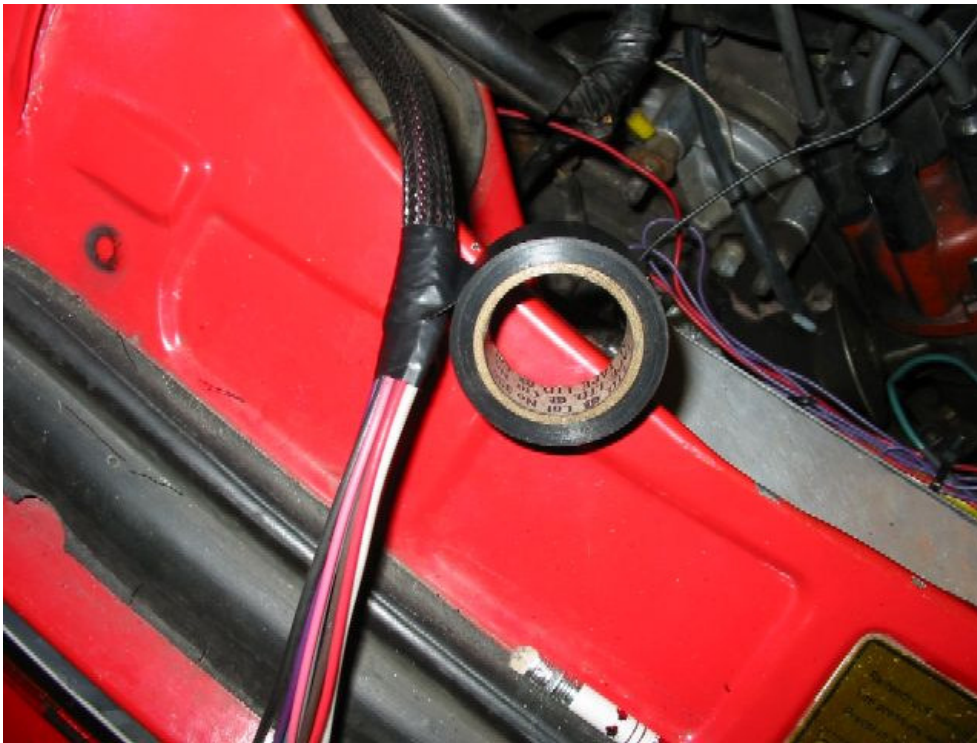
Figure 56: tape wire mesh sleeve
