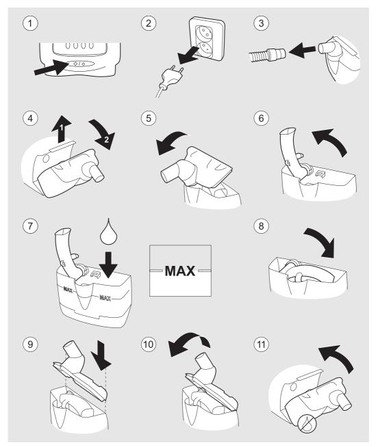
Add distilled water or boiled, chilled tap water to the humidifier until it reaches the marking "Max" on the humidifier. A full humidifier contains approximately 400 ml. Do not overfill the humidifier.
