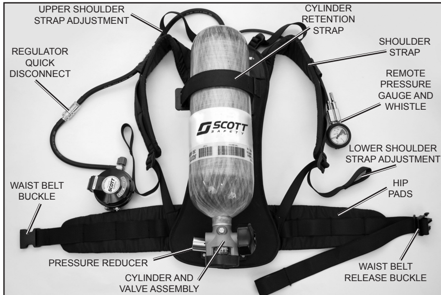
FIGURE 2 TYPICAL ACSI SCBA RESPIRATOR
