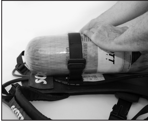
FIGURE 15 SECURE THE CYLINDER RETENTION STRAP
