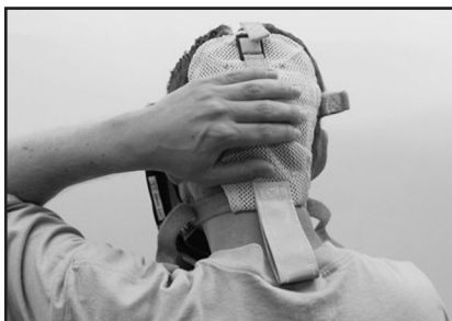
FIGURE 10-H HEAD HARNESS MUST BE FLAT AND CENTERED
