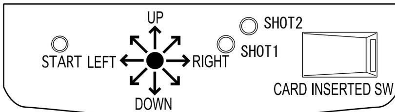
**1** The input buttons are functioning correctly if each respective display changes from “OFF” to “ON” when pressing the input buttons.
