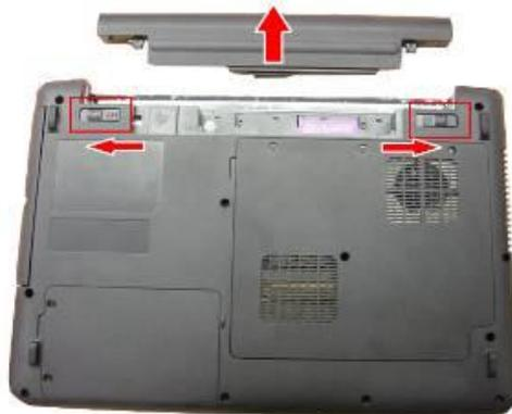
**NOTE:** Always start laptop disassembly by removing the battery pack first.
