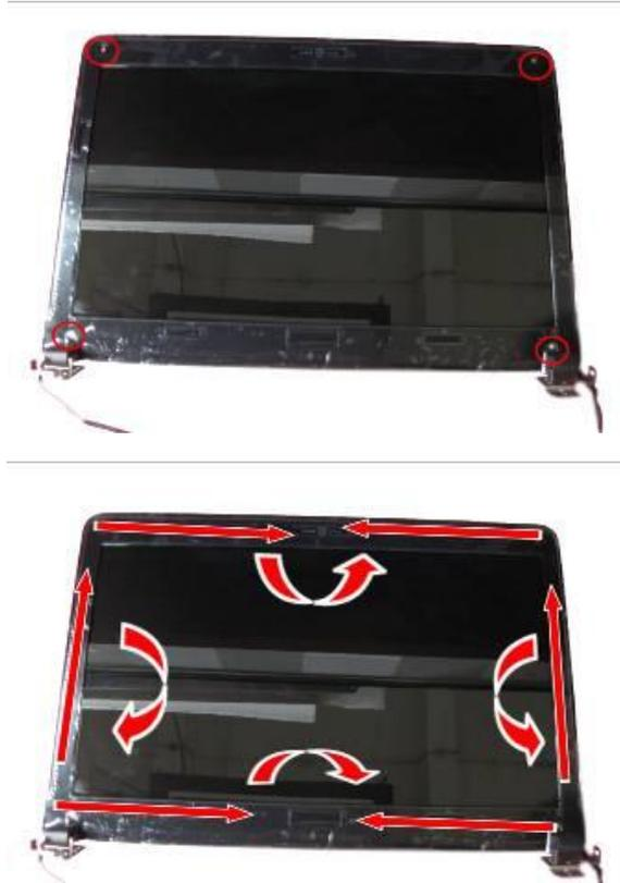
1.2.2 Disassemble LCD panel
