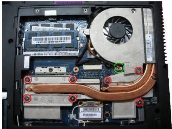
1.1.6 Disassemble WiFi card ;( first pull out RF connector, then take off 1pcs screw, and take out WiFi card)
