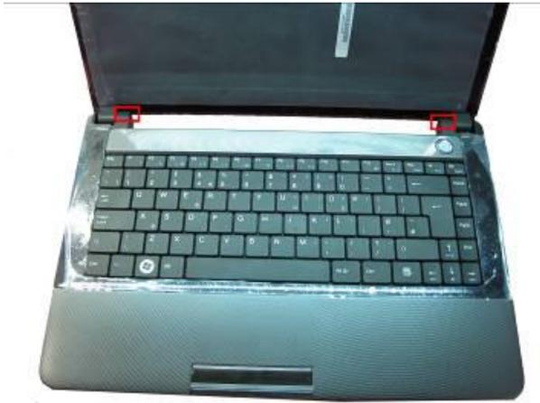
Reverse the machine first, and disassemble strip cover from left to right sides as below photo, then take off strip cover by up and down.
