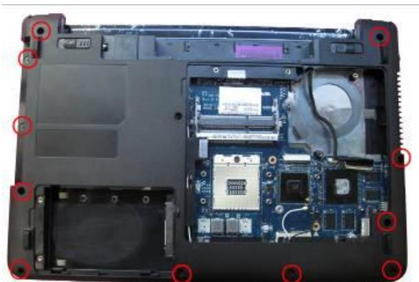
1.1.11 reverse machine and disassemble strip cover;
