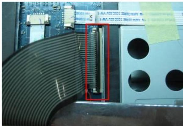
1.1.13 Open up power/B 、 speaker cable connector 、 T/P FFC & MIC cable connector , remove power/B and speaker;(take off 4pcs screw)
