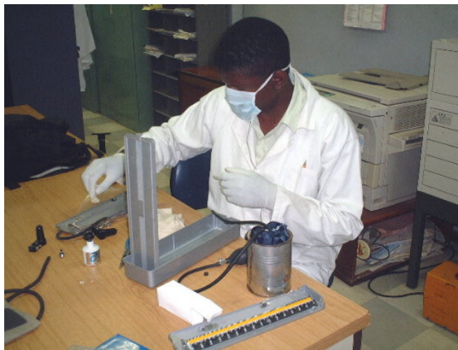
Photo 2.1 Protection from safety hazard: A medical technician wearing a mask and gloves repairs a mercury BP machine (Biomedical Engineering Department, University Teaching Hospital, Zambia).
