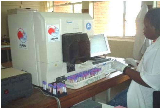
Photo 2.10 A haematology analyser: An analytical instrument that analyses RBC, WBC, HGB, HCT, MCV, etc. in blood sample; such equipment cannot be maintained only by operator and in-house service.
