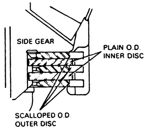
STEP 21: Install limited slip outer clutch disc (7). (Teeth on the outer diameter). See cross section reference after STEP 20.
