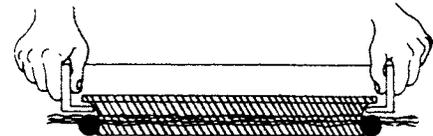
Wet toric in Tri-Chloroethane to let it slip easily under the housing retainer lip.
