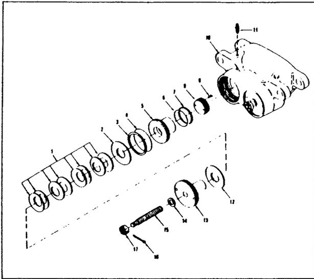
Fig. 1—Parking Brake Head TS-21976
