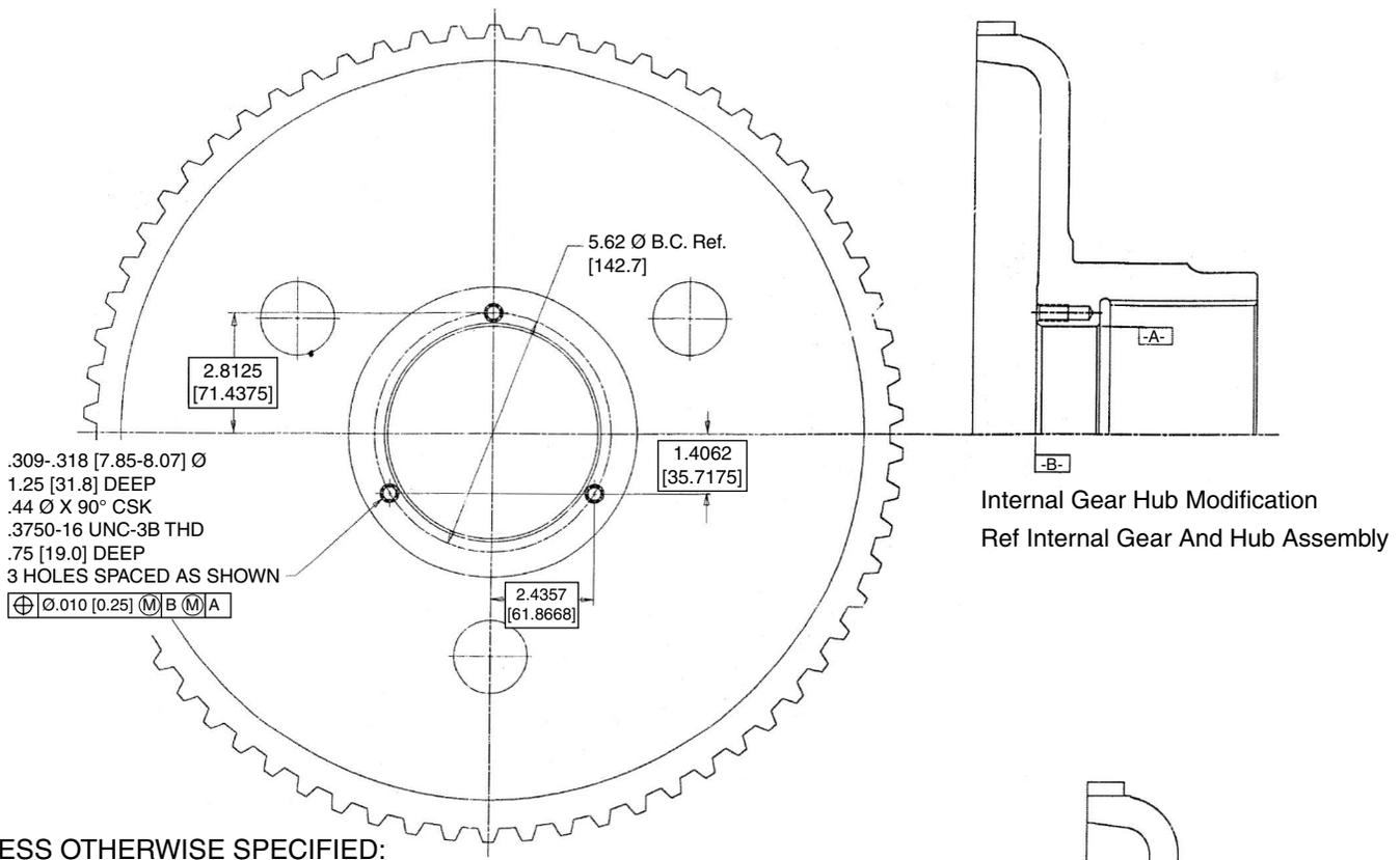
Internal Gear Hub Modification
