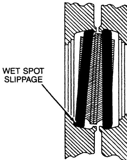
1. A wet spot between housing and ramp can cause sliding and cock the seal.
