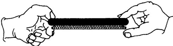
Toric must be on the bottom of the seal ring ramp. Make sure it is—**STRAIGHT.**
