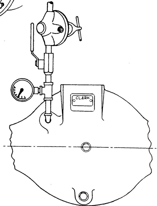
Air check the axle center section the same way as the wheel ends except the checking device is installed in the air breather hole in the axle center. If an air leak is detected, locate leak and correct. After air check is made, reinstall air breather in axle center.
