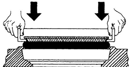
Toric can twist if it is dry on one spot or if there are burrs or fins on the housing retaining lip.
