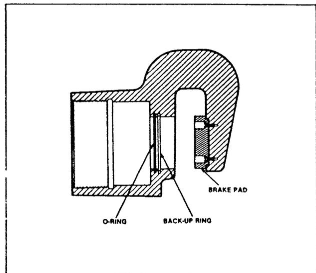
Fig. 2—Brake Head Housing TS-17361
