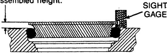
Height variation around the assembled ring should not exceed .040" (1.0 MM).
