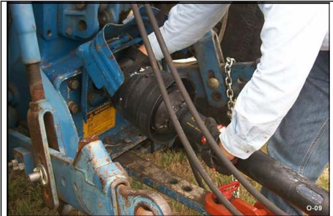
After the driveline is securely attached, place the tractor PTO master shield back in the operating position. OPS-R-0003
