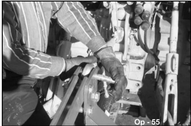
To disconnect the implement, first extend the tractor 3-point hitch top link to remove tension on the top link hitch pin. When the pin is loose and easy to rotate, remove the pin from the mower. Next remove both lower hitch pins.
