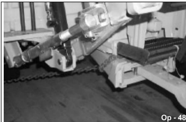
While hauling the tractor and implement, make occasional stops to check that the tractor and implement have not moved or shifted and that the securing chains have maintained tension. If during transport a hard braking, sharp turning, or swerving action was performed, stop at the next safe location to inspect the security of the load. *OPS-U- 0026*
