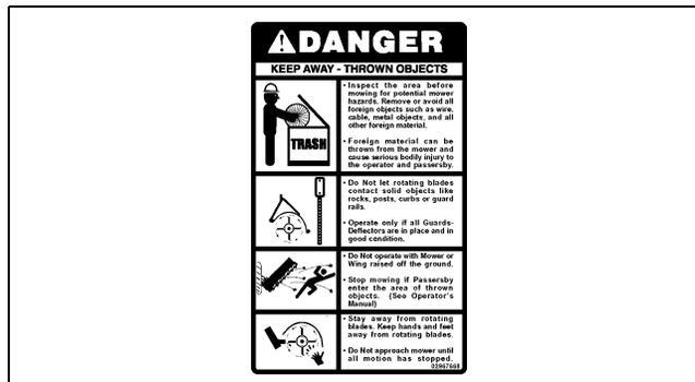
WARNING! Failure to use and maintain shields and deflectors in good condition may lead to injury or death from entanglement with rotating parts, being hit by objects thrown with great force by blades, or by blade contact.
