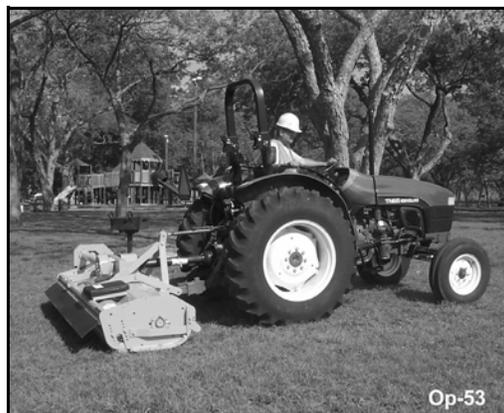
To avoid overturns, drive the tractor with care and at safe speeds, especially when operating over rough ground, crossing ditches or slopes, and turning corners. Tractor wheel tread spacing should be increased when working on inclines or rough ground to reduce the possibility of tipping.
