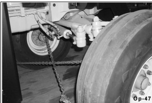
Arrange the chains so that when tightened, the chains are pulling downward and against themselves. Carefully tighten the securing chains or other fasteners used as much as possible using boomers or binders to apply maximum tension. Use extreme care when attaching and removing the securing devices as the extreme tension involved when released has the potential to inflict serious injury.
