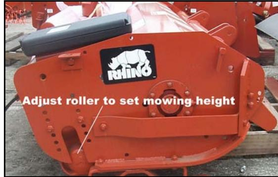
1. Place the tractor and mower on a level surface and completely lower the mower to the ground.
