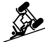
Be aware of the operating conditions. Do not operate the Tractor with weak or faulty brakes. When operating down a hill or on wet or rain slick roads, the braking distance increases: use extreme care and reduce your speed. When operating in traffic always use the Tractor's flashing warning lights and reduce your speed. Be aware of traffic around you and watch out for the other guy. (SG-19)
