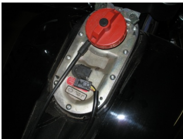
Step 5: Remove dash. Unplug the fuel pump connector and overflow hose. Start the engine to release the fuel pressure.
