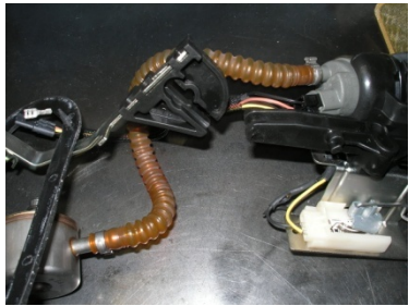
Step 9: Remove the pump assembly from the tank. Disconnect the wires from the plug. Remove the bail spring and separate the pump section from the plate section.
