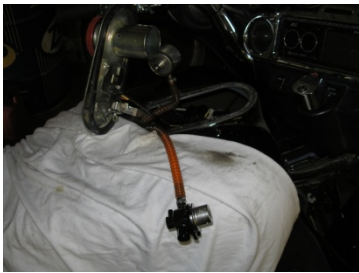
Step 8: Disconnect the regulator from the filter. You don't need to remove any fuel lines or clamps. Pull the regulator assembly from its housing.
