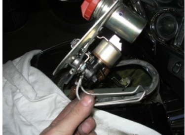
Step 7: Lift the pump assembly out of the tank enough to remove the bail clip. Hold on to the tab that the clip connects to, otherwise it will fall into the tank
