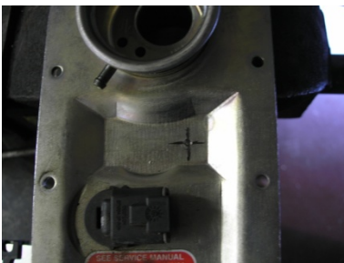
Step 10: Measure 9/32" from the edge of the stamped section. This is where you will need to drill for the bulkhead fitting. Be sure not to be any further away from the stamped section, otherwise it will interfere when you reassemble the pump assembly.
