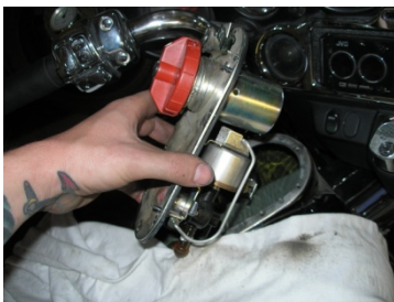
Step 6: Remove the fuel pump access plate.
