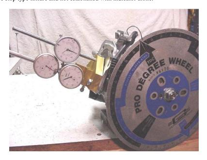
Cam will be checked with indicator reading off the top end of tappets, which will provide zero clearance. The inverted radius of the top of the tappet presents some problem to get accurate readings and to prevent binding of indicator stem. Indicator holder and positions are very critical in this operation
