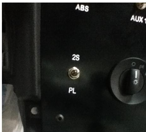
2. The RPM point is adjusted by moving the toggle switch up or down. The RPM will change in 100 RPM increments. The user range for the launch control is 2000 rpm to 7000 rpm and the PCM will not allow any settings beyond these limits.
