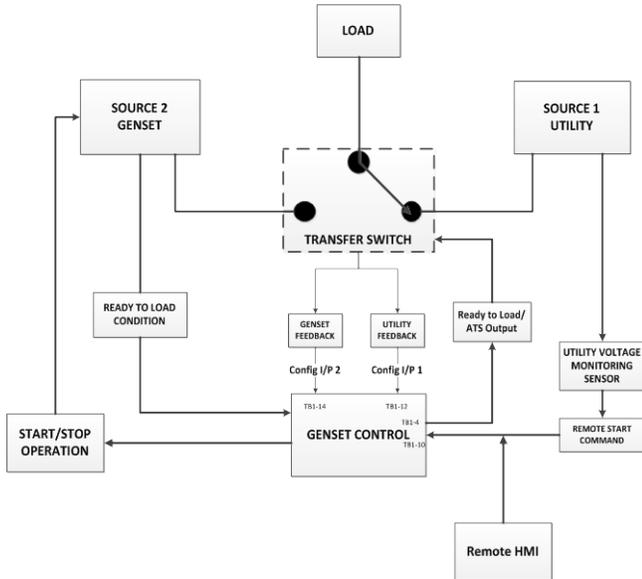
\* A utility voltage monitoring sensor (as shown in the AMF diagram above) must be connected in order to use the AMF feature on the 1302 control. Use Schneider Electric Relay RSB1A120U7, Socket RSZE1S35M.
