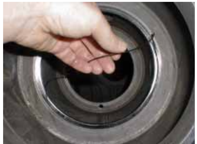
Fig. 4.5-3 Fit the O-ring
