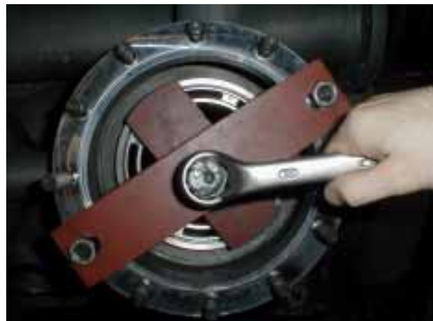
Fig. 4.5-8 Fit the cylinder liner
