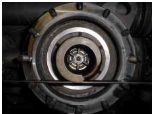
Fig. 4.8-4 Top view of discharge valve assy (new version)
