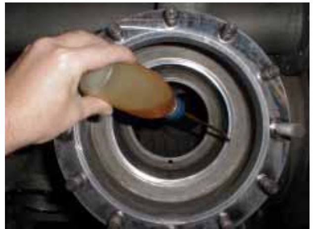
Fig. 4.5-2 Use compressor oil to oil the O-ring location
