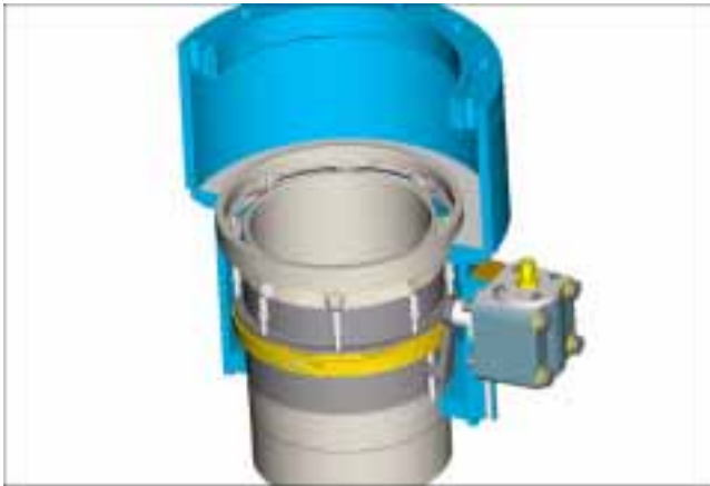
Fig. 4.5-9 Top view, suction valve with slots
