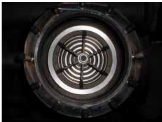
Fig. 4.8-2 Top view of discharge valve assy (new version)
