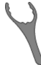
Fig. 2.8-1 Special tool for removing oil filters
