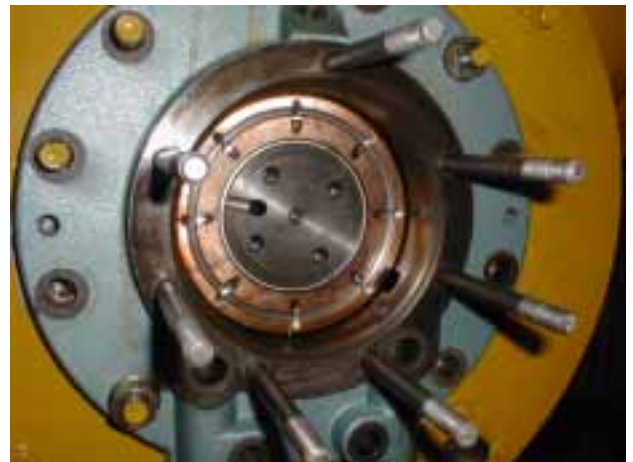
Fig. 4.1-8 Standard thrust bearing; refer also Fig. 2.10-2
