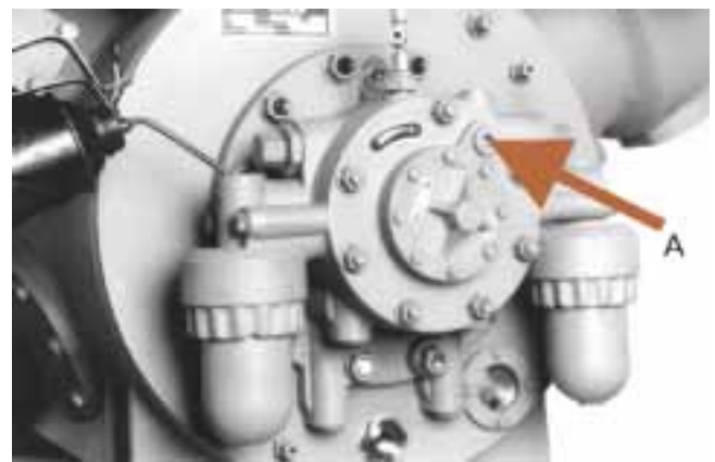
Fig. 4.12-2 Oil filters and location oil charge valve (A); not shown!
