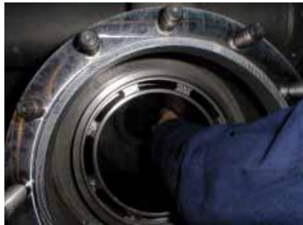
Fig. 4.5-7 Fit the cylinder liner
