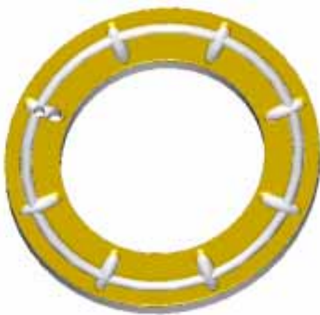
Fig. 2.10-1 Standard bronze thrust bearing, "mark 2"
