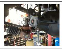
Mark the f. drive shaft for proper alignment during reassembly. Unbolt 9. and slide the drive line back to allow the axle to droop out.
