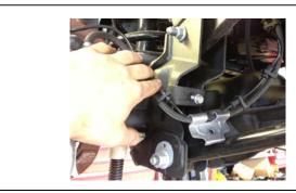
8. Unbolt and remove the f. brake line brackets from the axle.
