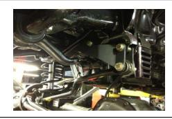
22. Install the track bar into the drop bracket.
