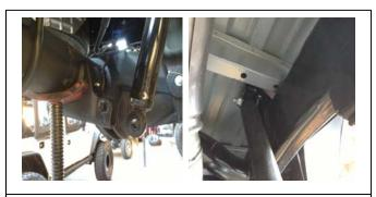
27. Support the rear axle and remove the shocks
