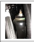
10. Fully support the f. axle and remove the shocks from the top first.
