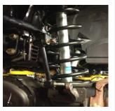
Install extended sway bar end links and adapter brackets.
