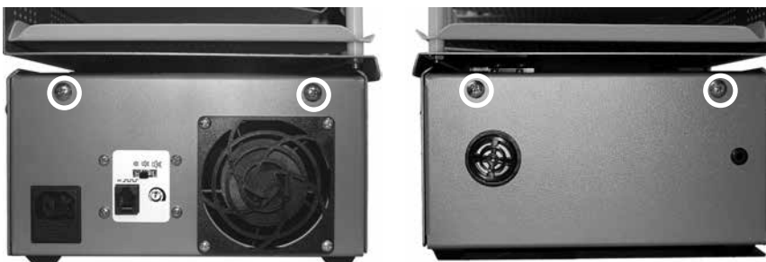
Slide rod screws (circled).
