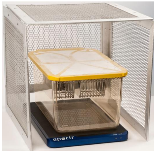
Figure 15. Completed Faraday shield assembly
