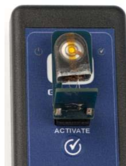
Figure 5. Activation of dual channel transmitter shipped in off state
