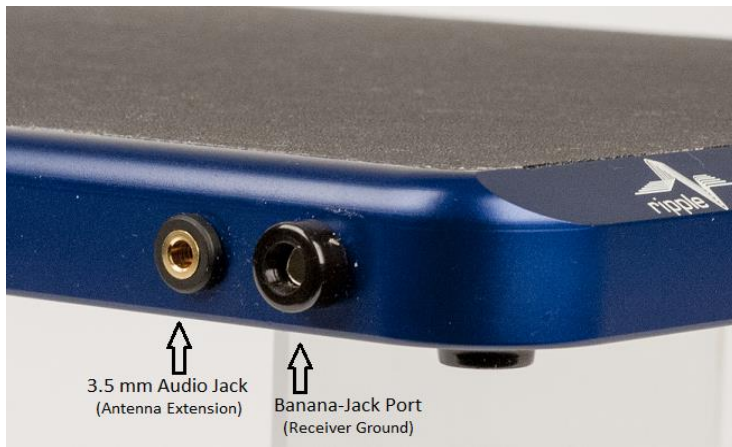
Figure 8. Antenna extension and Faraday shield connections
