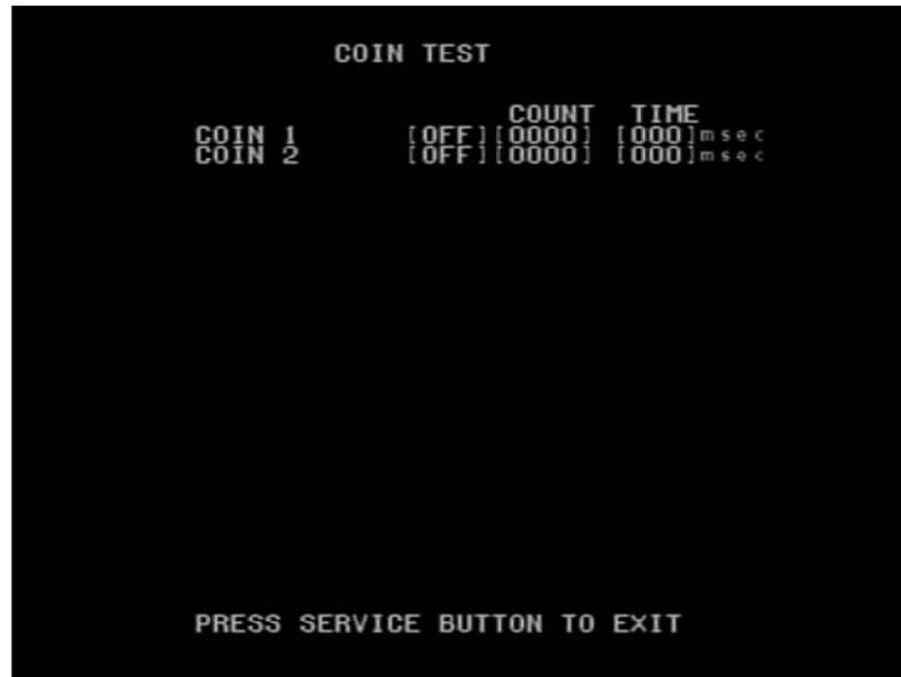
1. Function is working properly if the OFF display changes to ON when coin switch is activated.
