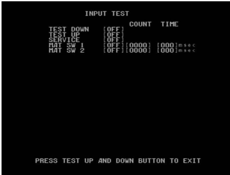
1. Controls are working properly if the OFF display changes to ON when operating the corresponding input device.
