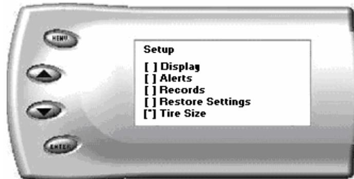
The *Evolution* has the ability to correct for changes in tire size. If you have changed your tires to a different size the PCM will miscalculate vehicle
